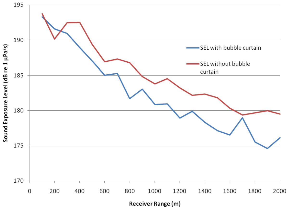
Figure 22: SEL versus range for the shallow water case at 5 m receiver depth.
