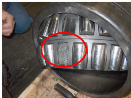
Pitting (wear) on one of 6 bearings from the planetary stage
