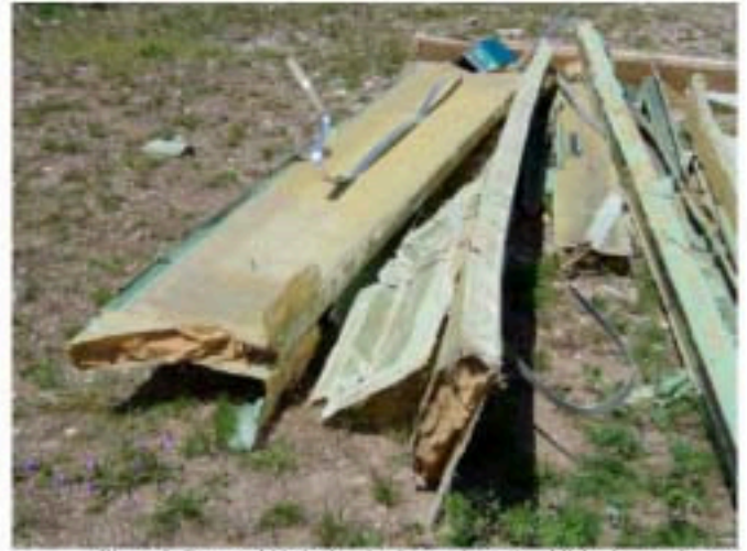
Figure 2: Damaged blade showing internal spars and lightning conductors
