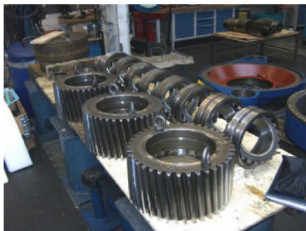
The three wheels and the 6 bearings from the planetary stage of a typical gearbox
