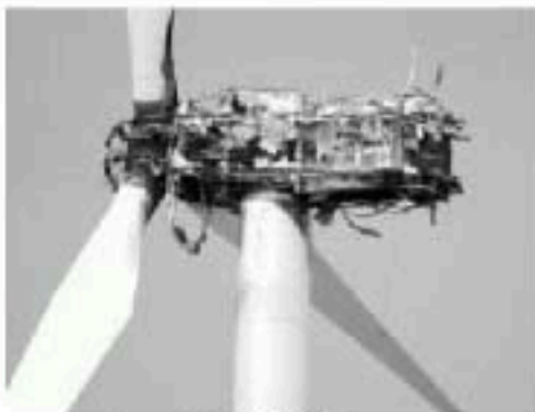
August 4, 2002: Fire VESTAS V80, 2 MW Year of construction: 2002 Location: Katzenberg near Meißen C20020804.1.bmp
