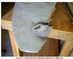
99999999.3.bmp Figure 1. Characteristic lightning signature on blade tip
