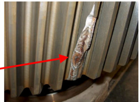
Broken tooth on the low speed gearwheel in a 2 MW gearbox
