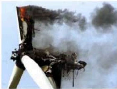
Fire caused by a short circuit, frictional overheating or lightning in 2004 in a Germany. Source: Der Spiegel, DPA.
