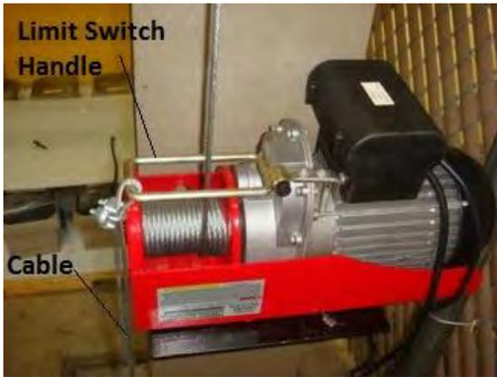
**Fig47.** Limit switch handle on hoist.
