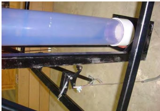
**Fig49.** Limit switch mechanism in action.
