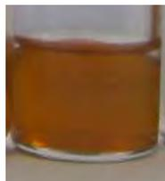
**Fig. 50—Thick, clear, orange colored, viscous epoxy resin.**
