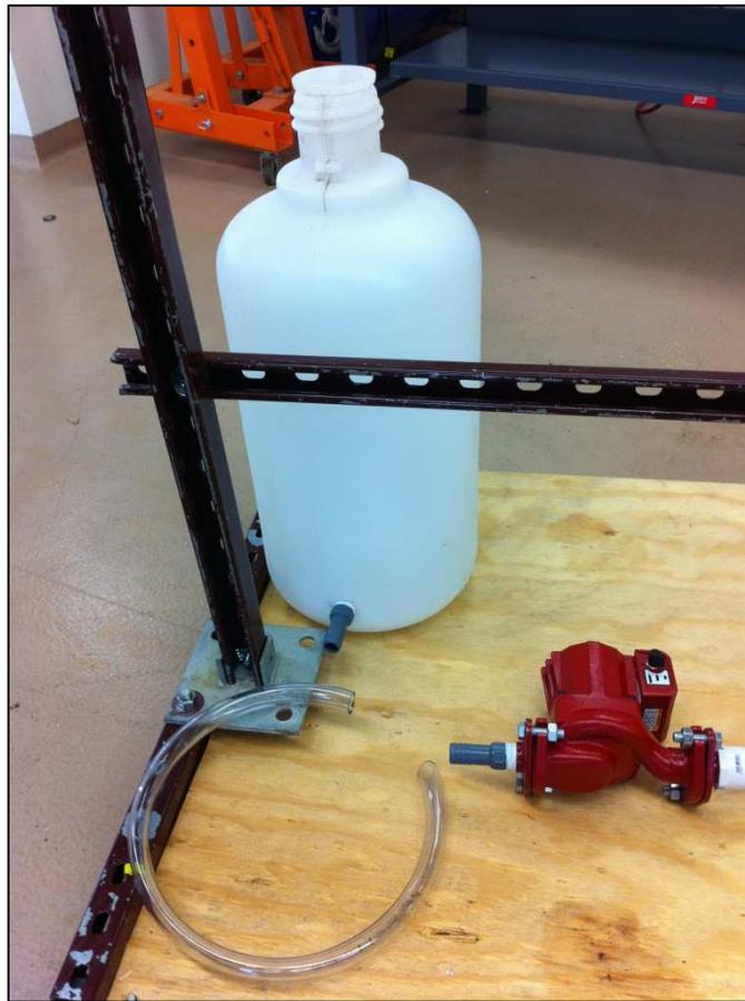
**Figure 5.13 Reservoir for the pump's water supply.** Once the system is filled with water, the only function of this reservoir was to act as an intermediate medium for the circulated water.
