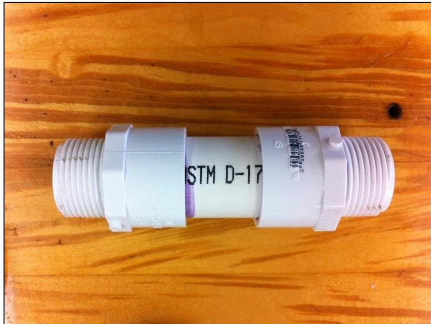
**Figure 5.10 1" Hard pipes with threaded connections**
