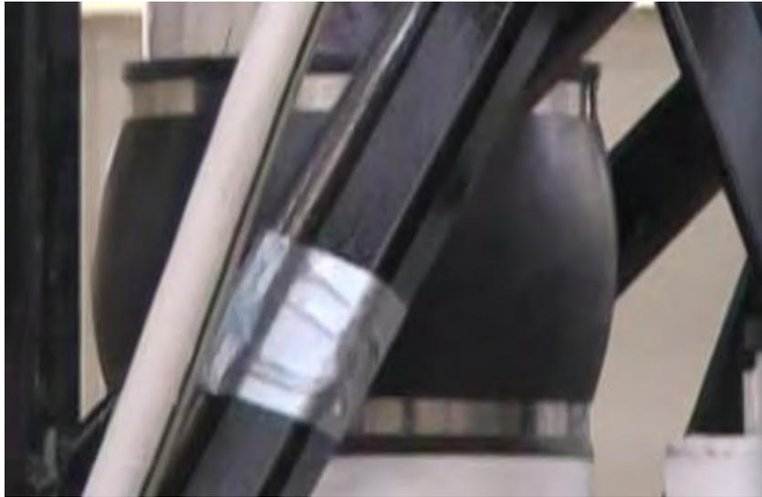
**Fig62.** The rubber coupling bulges due to hydrostatic pressure of the water column.
