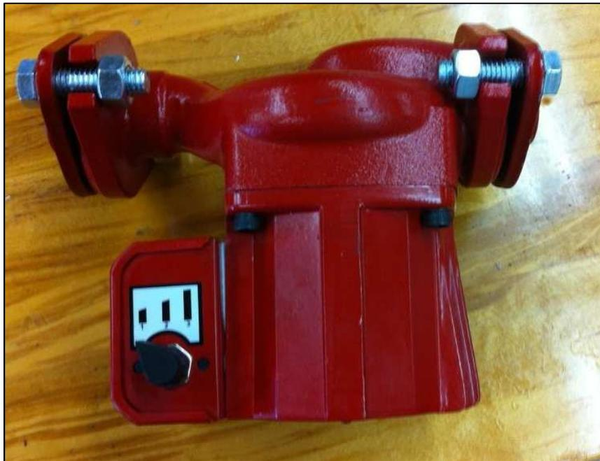
**Figure 5.5 3/4" Pump (The pump has 3 different speeds that can be adjusted by the switch)**
