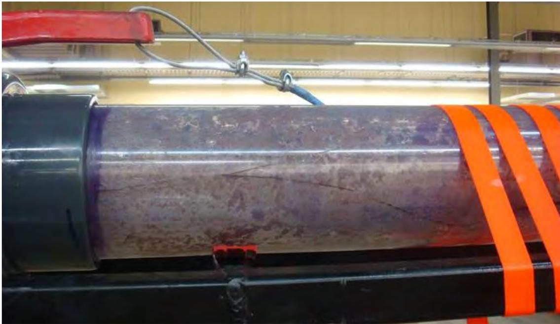
**Fig67.** Adhesion of epoxy for a vertical pipe at top section.
