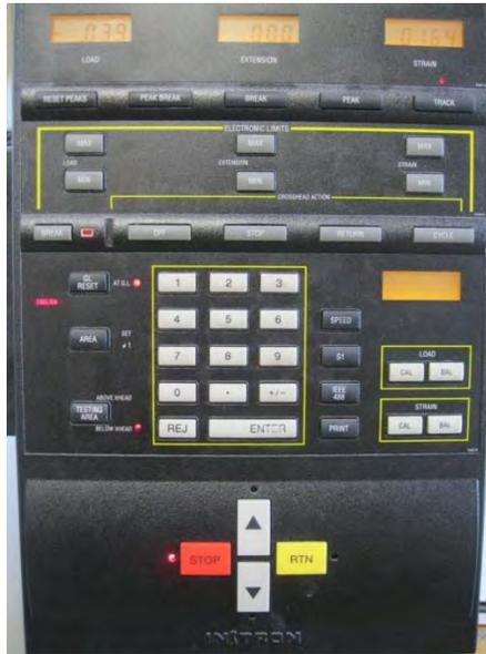
**Fig. 13—The control panel for the Instron 4206.**
