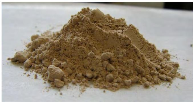
Fig. 11–The picture of barite powder applied in our research
