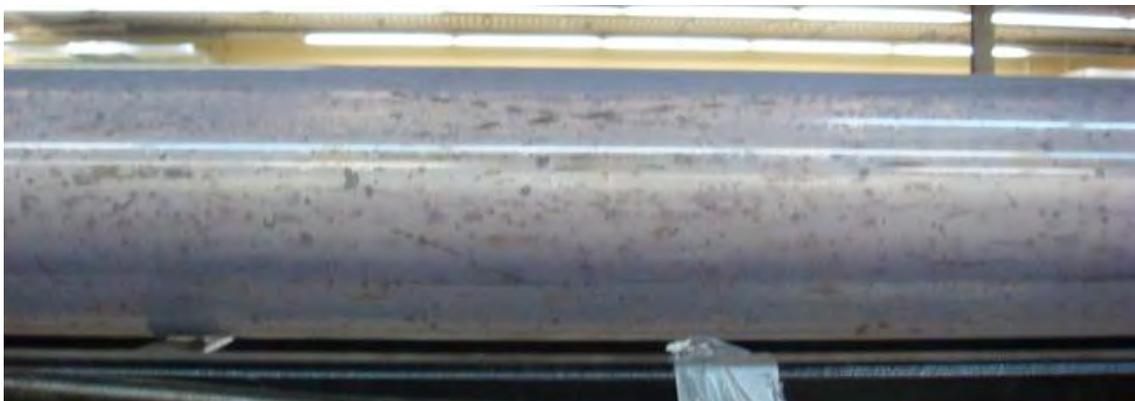
**Fig68.** Adhesion of epoxy for a vertical pipe at middle section.
