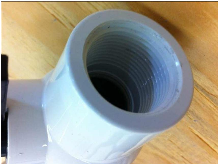
**Figure 5.9 1" PVC valve with threaded connection used in the assembly**
