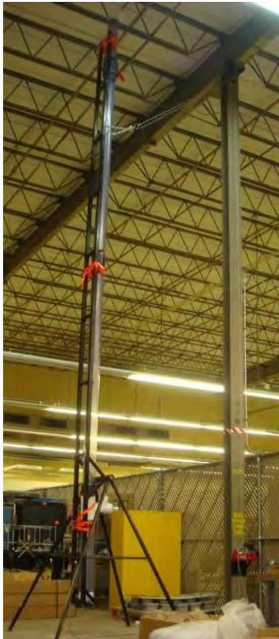
**Fig45.** The pipe support assembly in vertical position.
