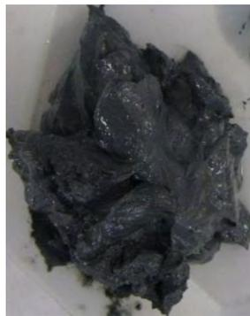
**Fig. 41—4010NM pipe dope compound**
