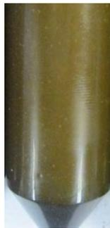
**Fig. 34—The fully cured sample of resin mixed with OCTG pipe dope.**
