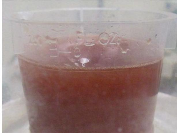
**Fig. 17**—An emulsion of resin droplets in seawater brine during and after mixing for one hour prior to curing.
