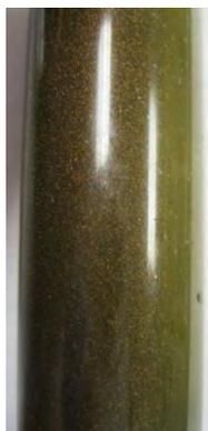
**Fig. 26—The fully cured sample of resin mixed with API-Modified pipe dope.**
