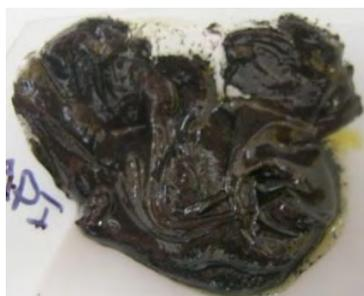
**Fig. 25—API-Modified pipe dope compound**
