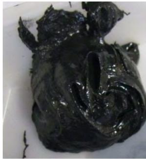
**Fig. 37—Metal-free pipe dope compound**
