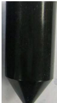
**Fig. 45—The fully cured sample of resin mixed with sour oil.**
