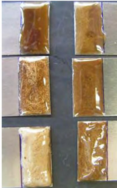
**Fig. 18**—After one hours of being soaked in synthetic seawater, the epoxy was mixed with synthetic seawater. The left three samples are for A epoxy system. The right three are F epoxy system's samples
