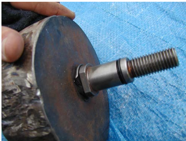
2000 fsw friction stud with the O-ring seal from the US Navy testing
