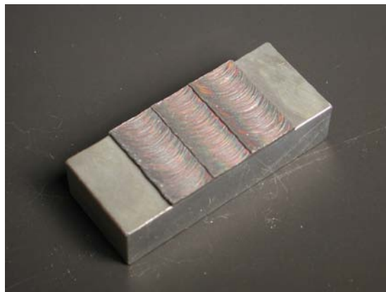
Figure 20 – Multi pass friction surfacing (Courtesy of GKSS Forschungszentrum)
