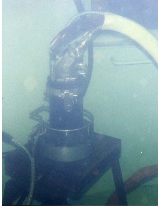
Figure 8 – The HMS3000 hydraulic tool in an electromagnet clamp.
