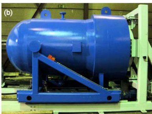
Figure 15 (a) The HyperWeld 2,500m (8,200 ft) deepwater welding facility at Cranfield University, UK and (b) the shell of Statoil's new 400 bar (13,120 ft) welding facility.
