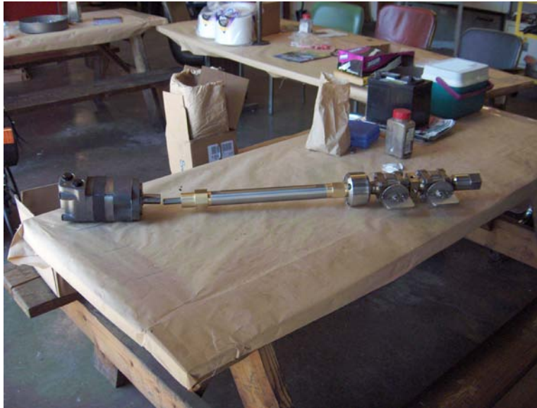
Hot tap drill motor, hot tap drill packer and dual valves above the friction stud mount
