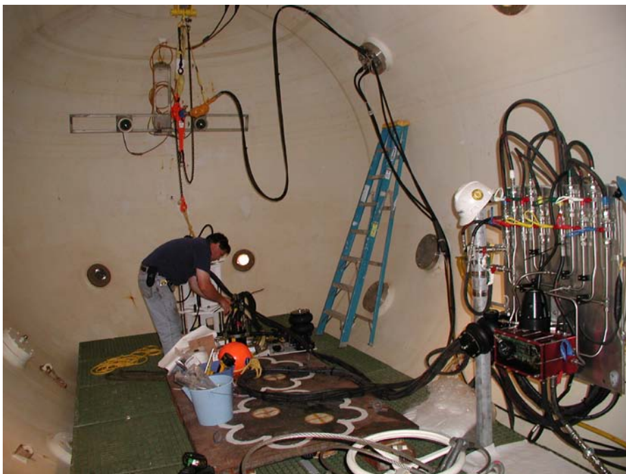
Interfacing the array of equipment to the bulkhead penetrators of the US Navy chamber
