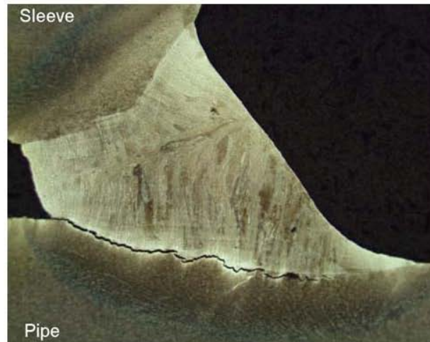
Figure 7 Instrumented restraint crack test for a pipe-on-pipe sleeve weld under radial constraint conditions showing cracking in the HAZ in the pipe wall [10].
