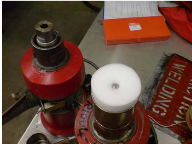
Figure 10 – A foam shroud fitted to an R1004 stud welding tool for underwater welding
