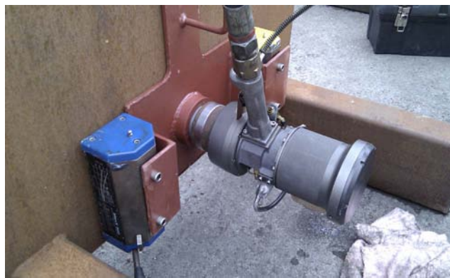
Figure 6a – An air powered tool in a jig with permanent magnets, used for an FPSO repair
