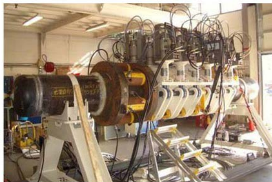
Figure 14 Retrofit tee for hot tap applications [30,35].
