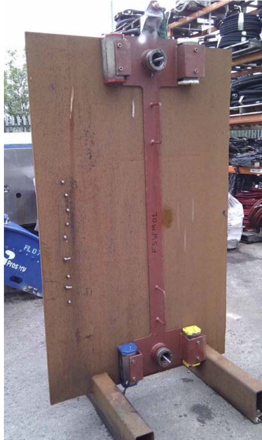
Figure 6b – The jig shown with M12 stud welds at each location
