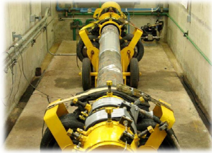
Figure III.4: Fatigue Testing of Upset SCR welded Joints
