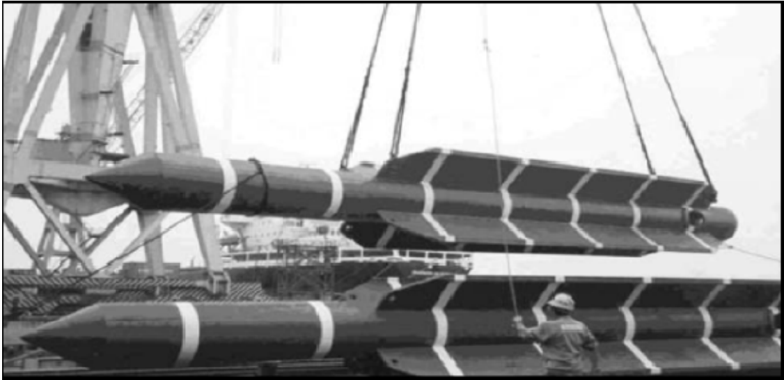
Figure V.1: Typical Torpedo Pile Geometries as used by Petrobras in the Campos Basin
