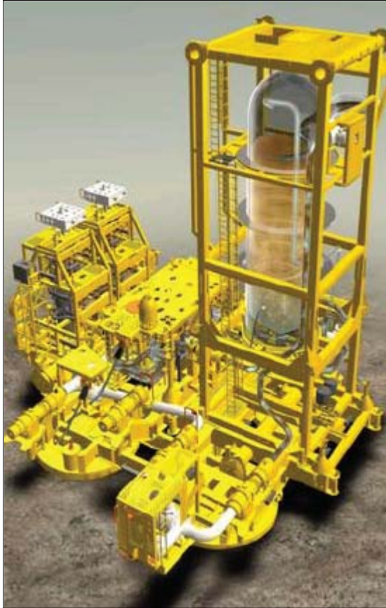
Figure 31: Pazflor vertical separation system
