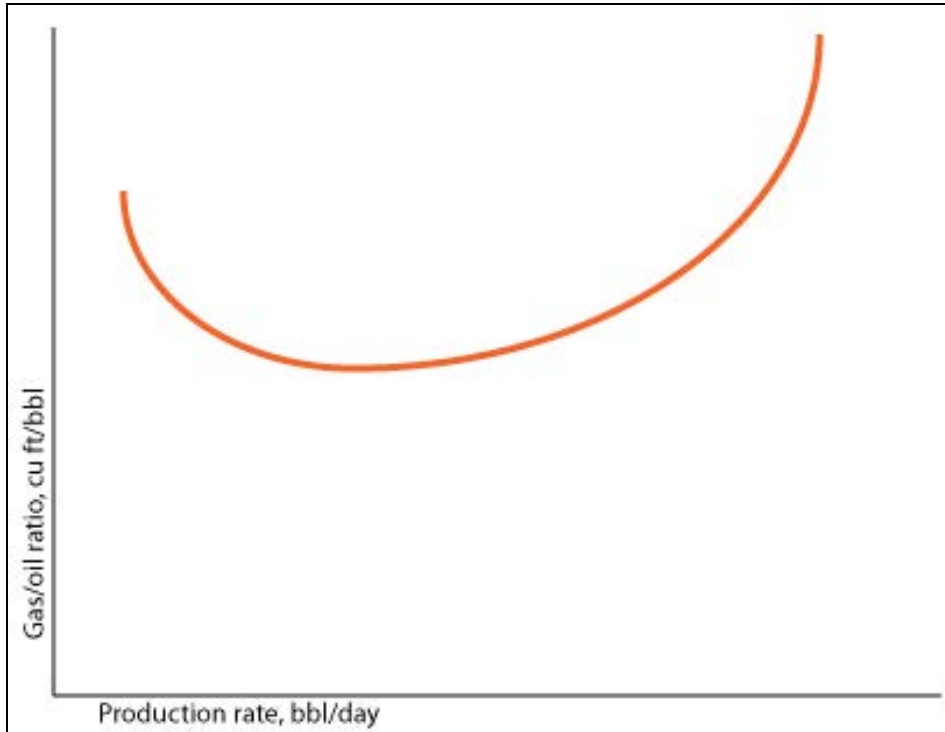
Figure 5: Indicative gas/oil ratio versus production rate for a commingled well
