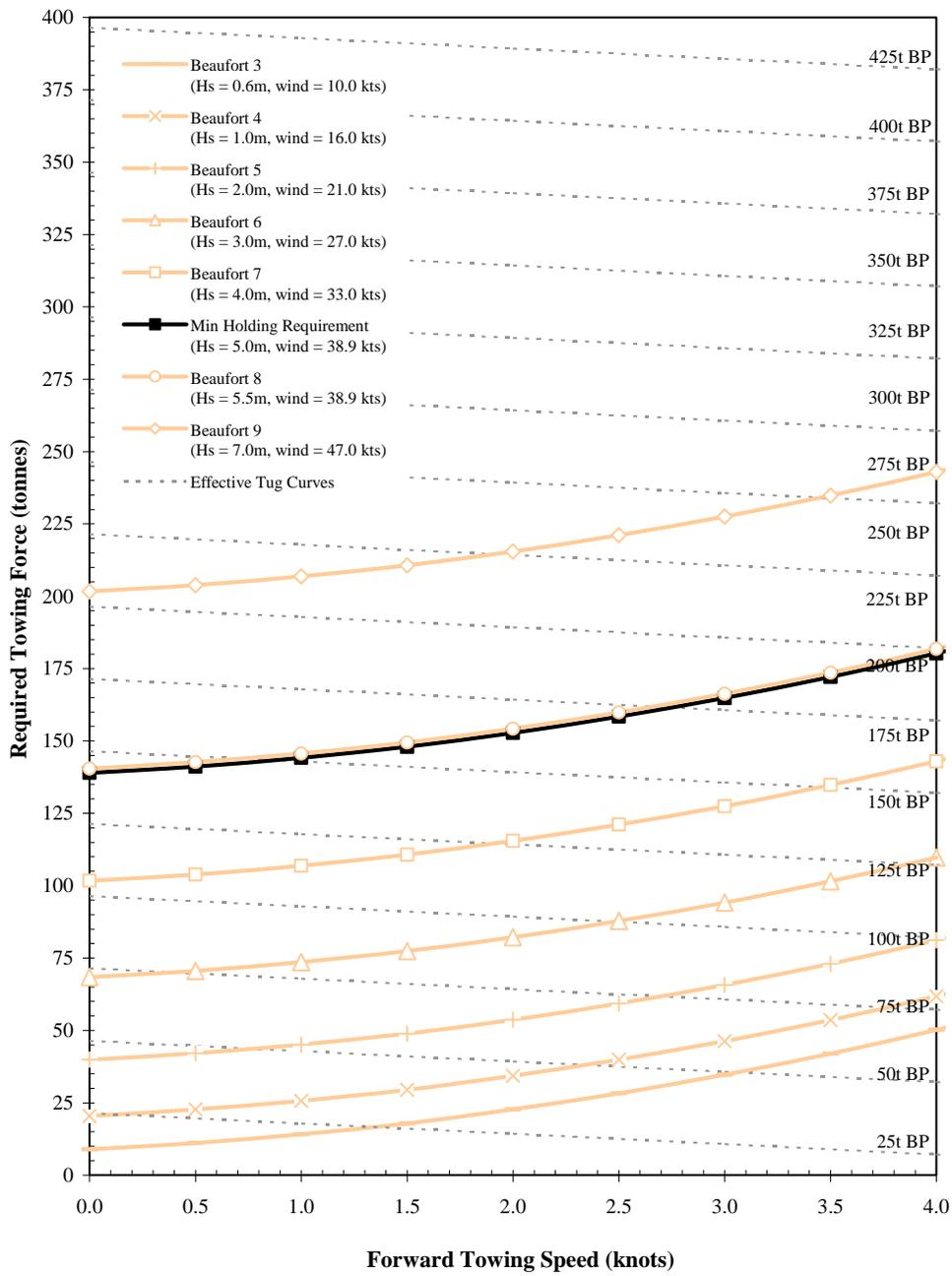
**Figure 55: Towing Curve for a Drill barge**
