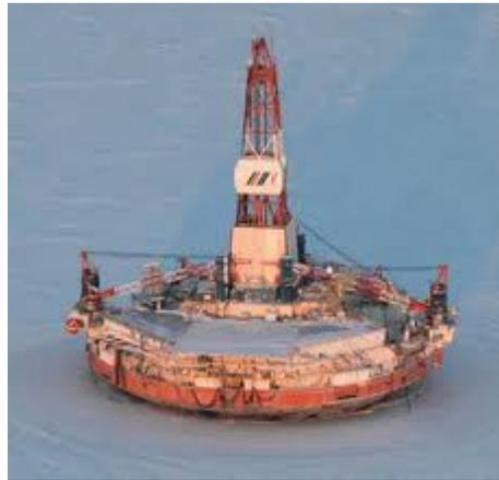
**Figure 35: Ice-breaking drilling Barge-Kulluk**
