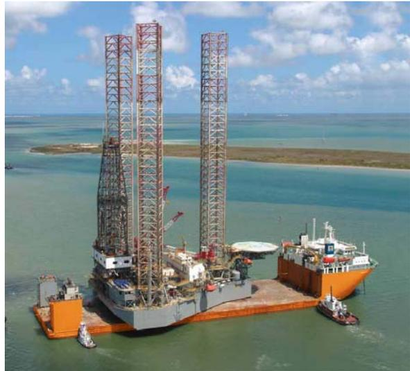
**Figure 39: M/V Black Marlin (3 Jack-up Loads, left). M/V Transhelf (Single Jack-up Load, right).**
