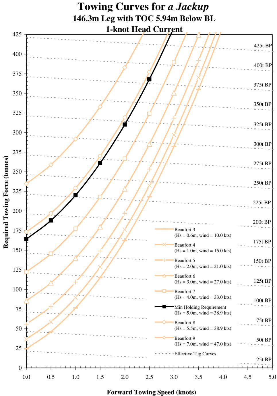
Figure 54: Towing Curve for a Jack-up rig
