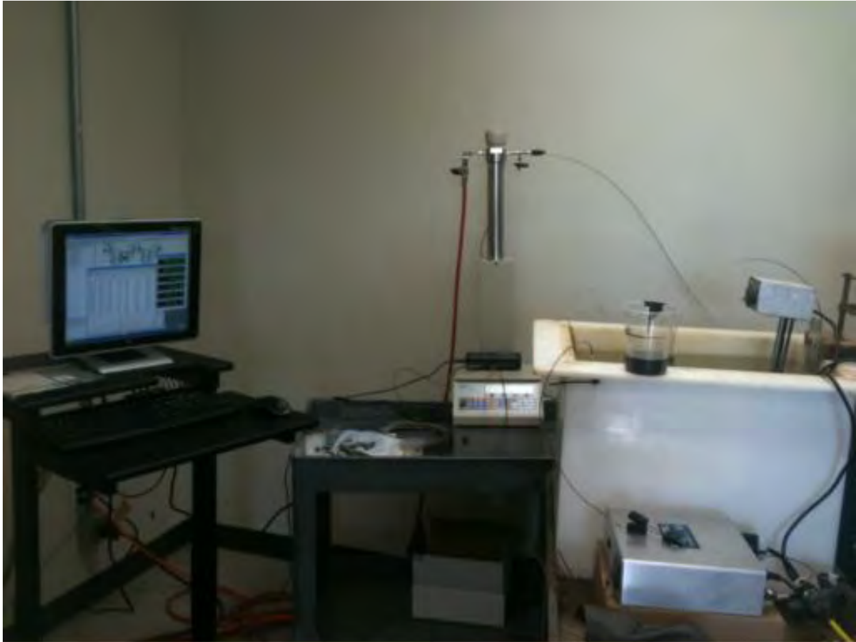
Figure 15: Volume Reduction Measurement during Cement Hydration Test Apparatus
