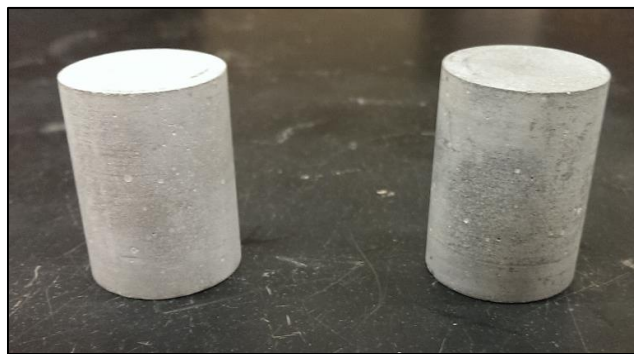
Fig. 2.35: Cured cylindrical samples for porosity and permeability and compressive strength testing
