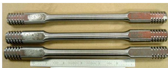
Fig. 3.9: Mini-pipe specimen (Cernocky et al. 2007)
