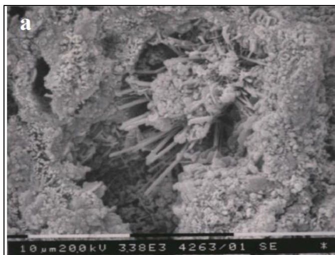
Fig. 2.7: SEM image of Class G cement showing presence of acicular needle like ettringite (Morales et al. 2003)
