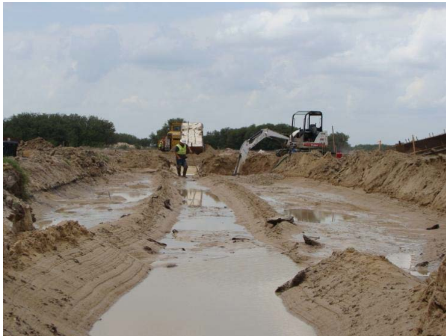
Figure 6.14: Typical Gouge Produced in Sand Test (Sancio et al., 2011 [117])
