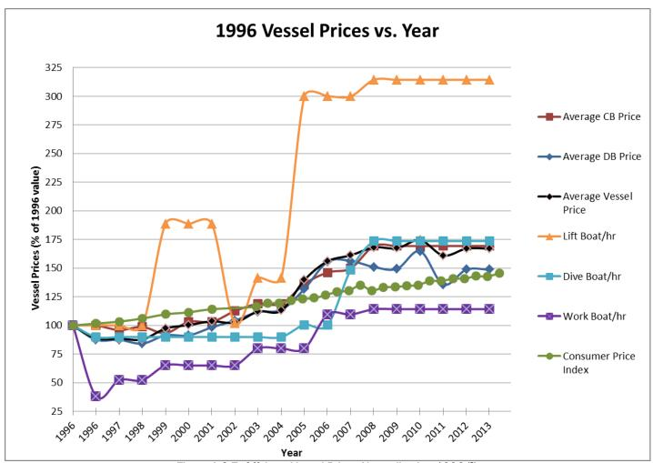
Figure A.6-7 Offshore Vessel Prices Normalized to 1996 (2)
