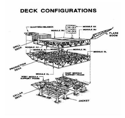
Figure 13.2. Deck Configurations
