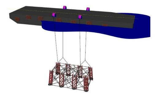
Figure 13.3. Lifting Barge Conceptual Drawing
