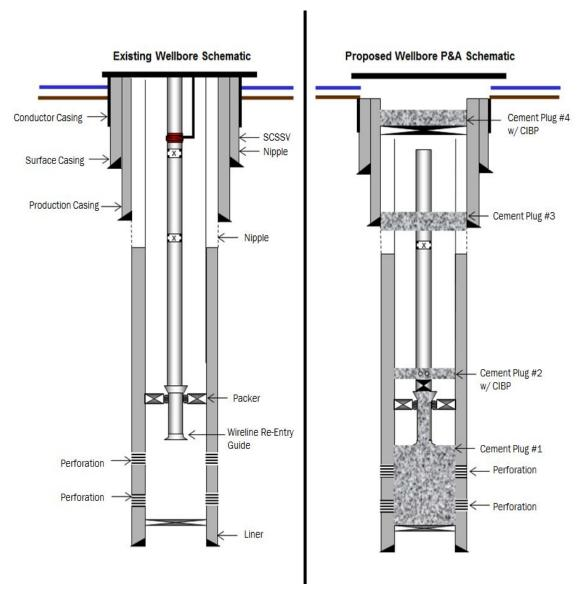
Figure 9.1. Typical Wellbore Configuration (Existing & PA Schematics)
