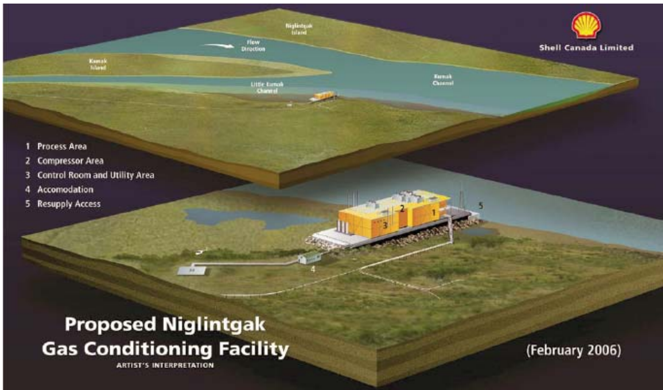
Figure 3-60: Proposed Placement of Niglintgak Gas Processing Facility on Seasonal Flood Plane (from Mackenzie Gas Project, 2006)
