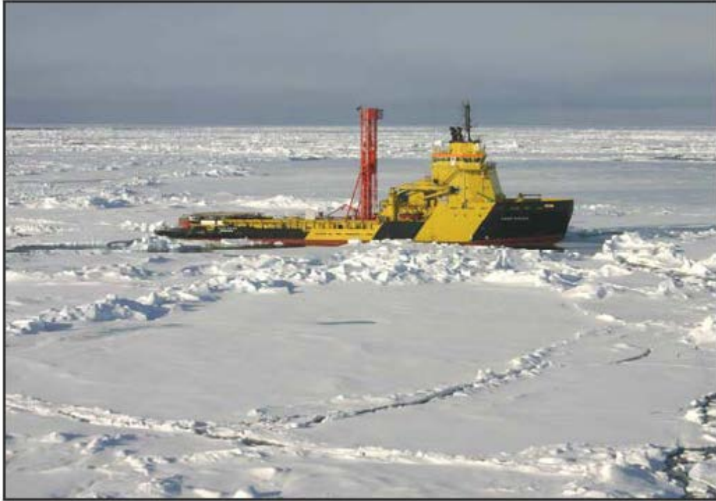
Figure 3-37: “Vidar Viking” Equipped with Compact Drill Rig, in the Central Polar Pack (Keionen et al., 2007)
