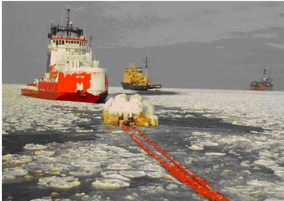
Figure 4-38: Ice Breaker “Smit Sibu” Providing Ice Management Operations for SALM Buoy Lay Down Operations on Sakhalin 2 (Courtesy of Don Connelly)
