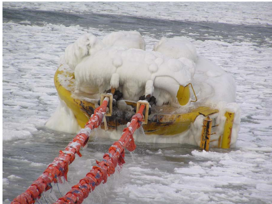
Figure 3-31: SALM Buoy Ice Up After Storm Event (Courtesy of DC Marine)
