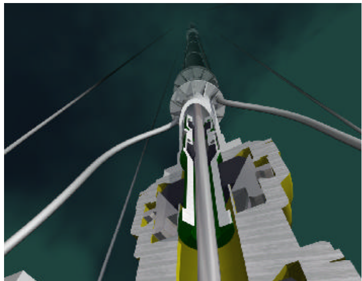
Figure 4.6 – Internal Rotating Control Head for Marine Risers
