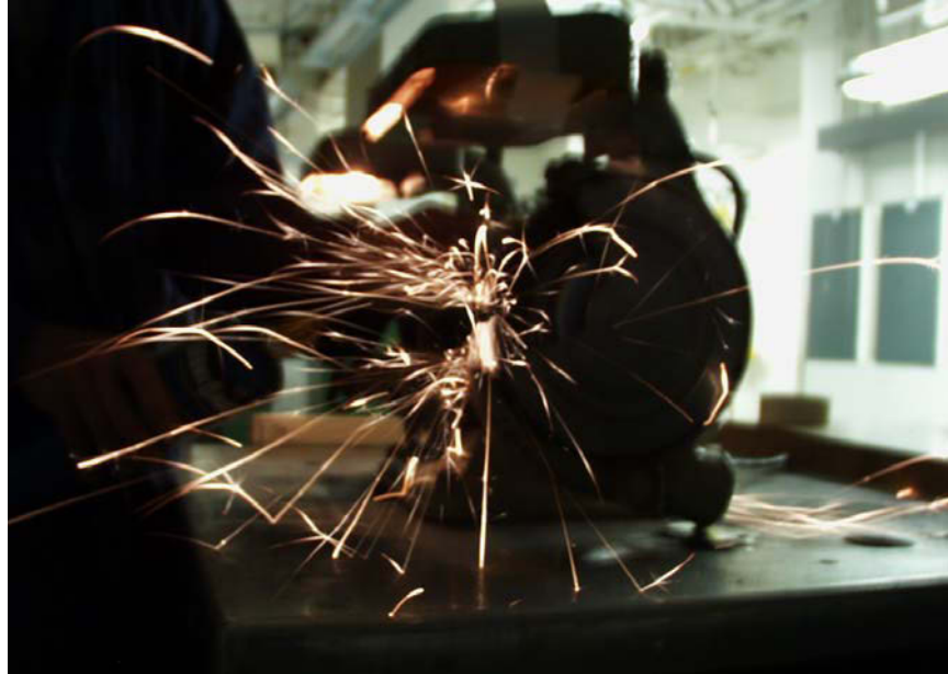
Figure 35. Sparks generated by steel grinding, which did not ignite flame for the propane-fueled brazing torch.
