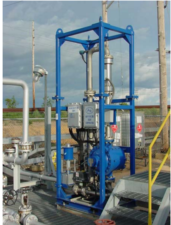
Figure 5.2: Multiphase Meter in Use in Venezuela
