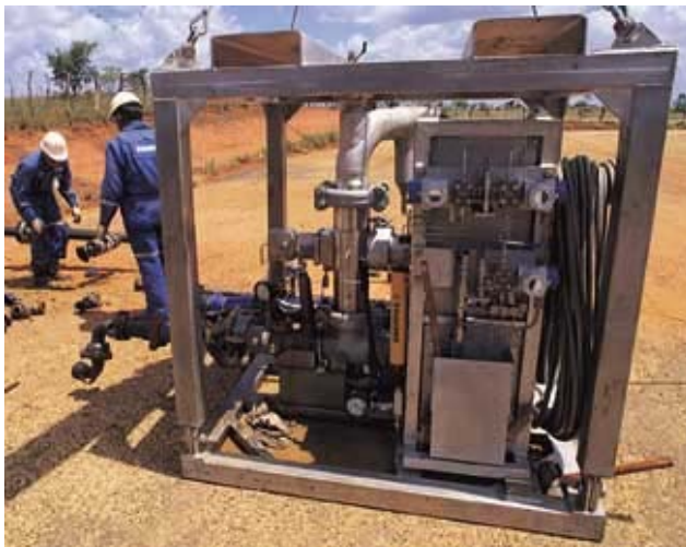
Figure 5.3: Portable Multiphase Meter (Schlumberger)
