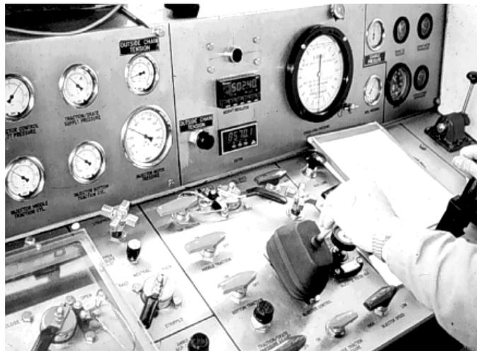
Figure 13. CTU Operator's Console
