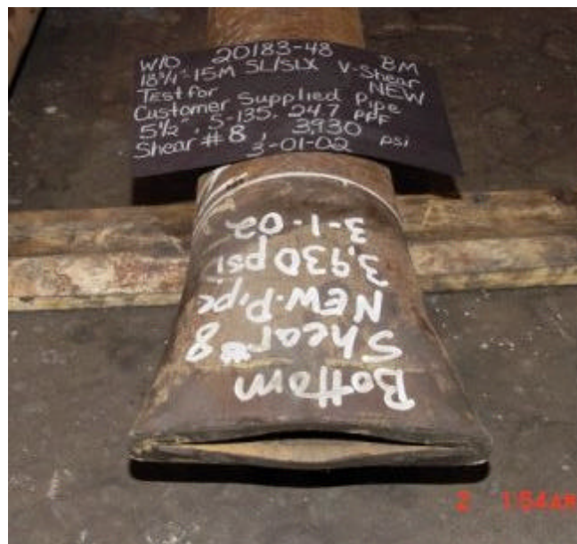
Shear test on old pipe (left) and new pipe (right). The new pipe required almost 2,000 psi more to shear than the old pipe even though the specifications on both pipes were the same.
