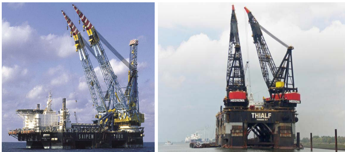
Figure 2.11 - Saipem 7000 and Heerema Thialf Semi-Submersible Crane Vessels
