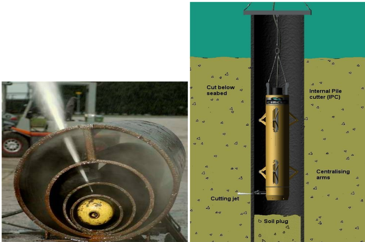
Figure 2.5 Water Abrasive Cutting c/w internal manipulators
