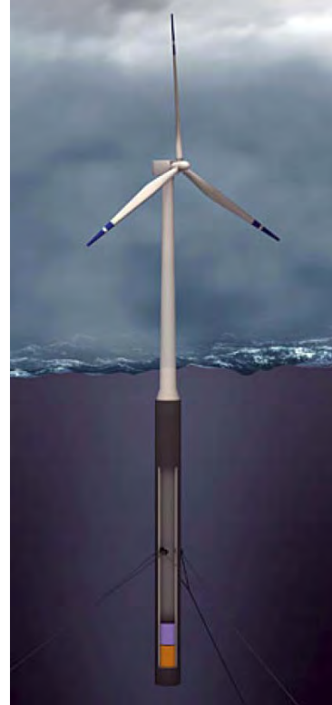
Figure 2.9. The Hywind Turbine and Support Structure
