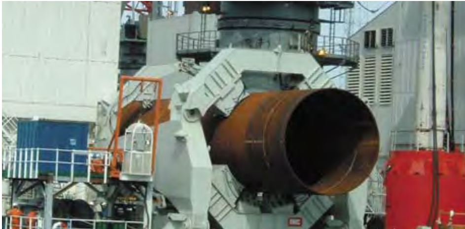
Figure 5.1. Monopile Upending Frame
