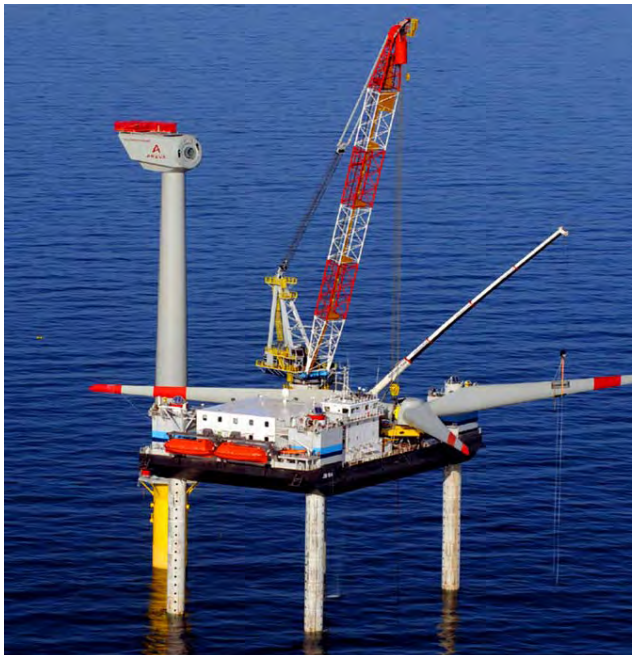
Figure 6.3. The JB 114 , a MSC SEA 2000 Jackup Barge
