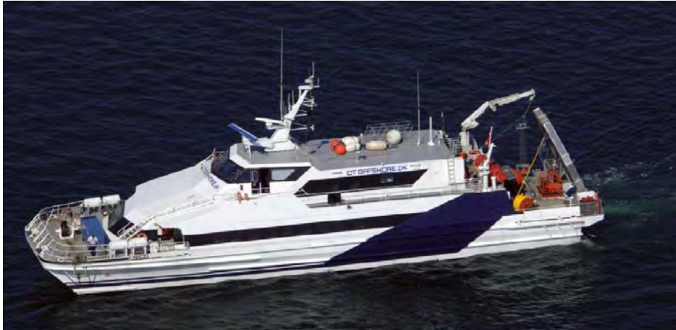
Figure 6.7. The Nico , a Modified Offshore Supply Vessel Installing Inner-Array Cable
