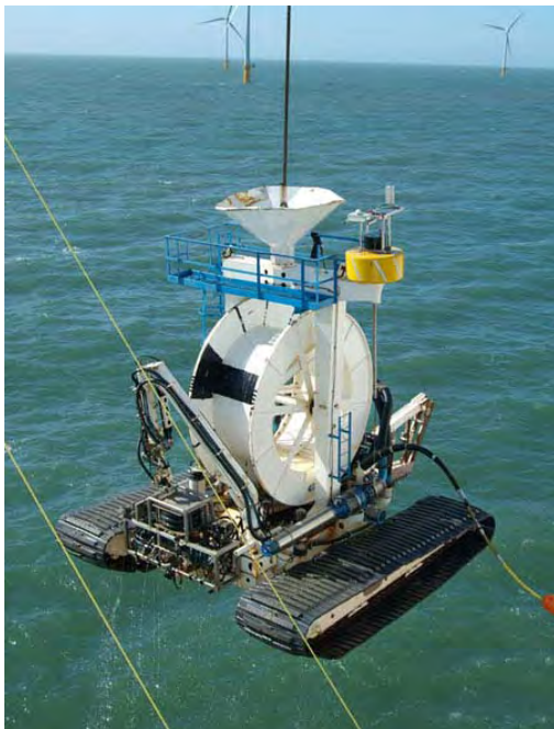
Figure 5.14. Tracked ROV Operated by the MV Resolution
