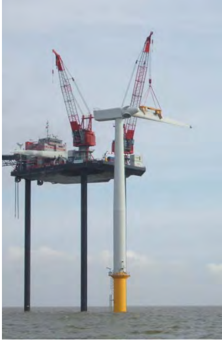
Figure 6.1. The KS Titan II Liftboat
