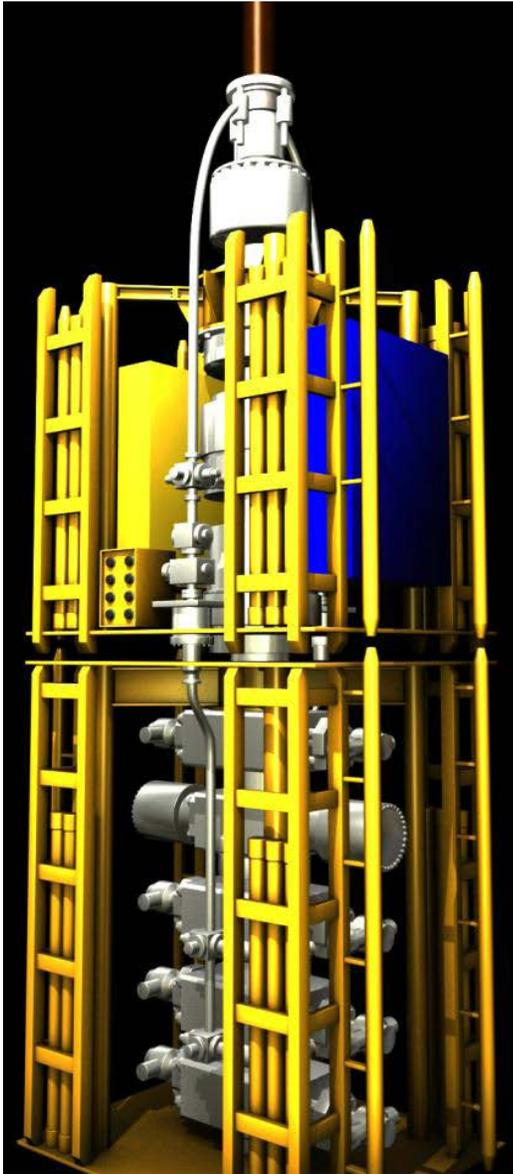
Figure 9: BOP Stack<sup>43</sup>
