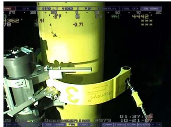
Figure 15: Deep water Pipe Pressure Sensor<sup>50</sup>
