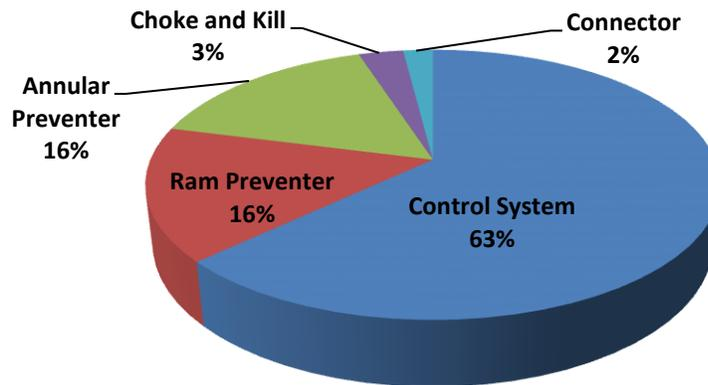
Figure 3.1: Failure Distribution from Subsea BOP from Study 4 [50]
