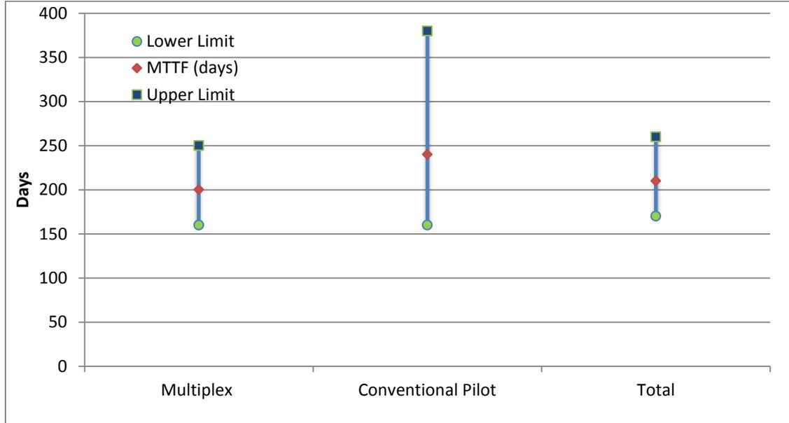
Figure 3.3: BOP Control System MTTF on Study 3 [31]
