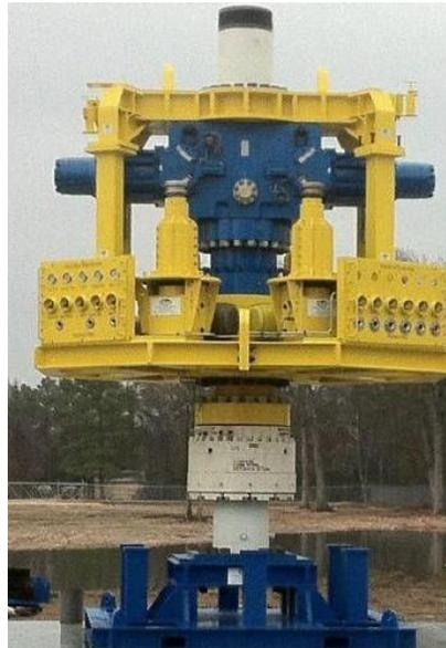
Figure 9.5: Capping Stack [12]
