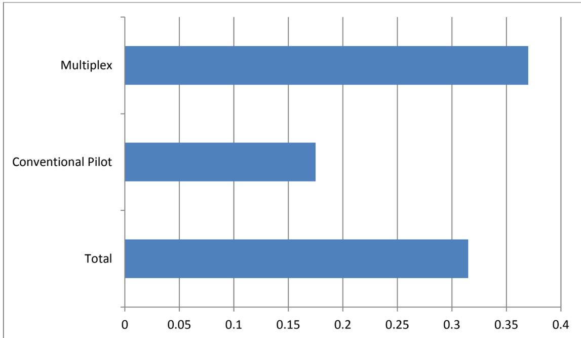
Figure 3.4: Average Failure Downtime per BOP Day on Different Types of BOP Control System for Study 3 [31]
