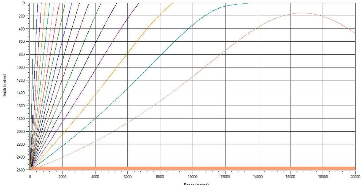
**Figure 7.13: Propagation Path to Seabed (2,600 meters) to Surface [12]**
