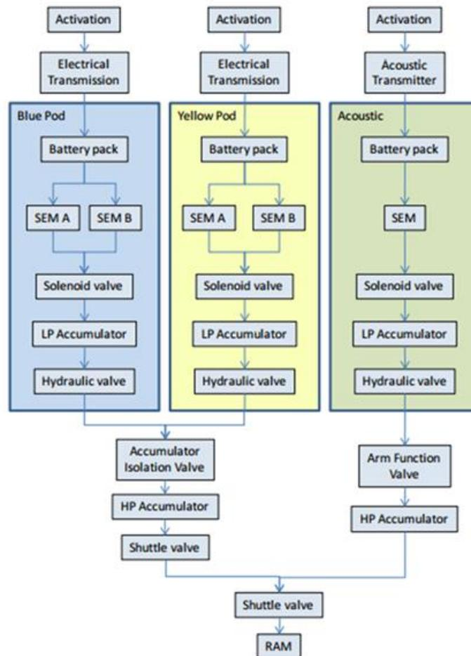
Figure 7.9: Single Point Failure at the Shuttle Valve [61]
