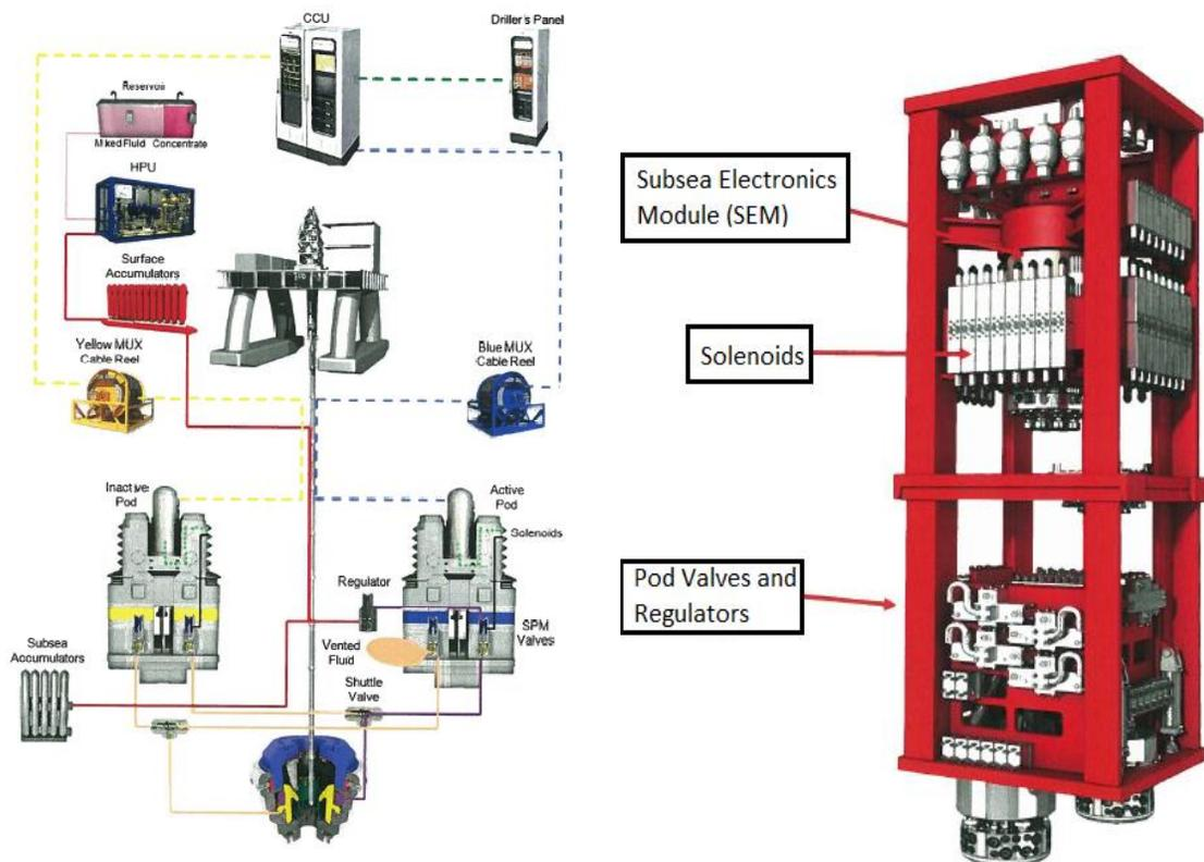
Figure 2.2: MUX BOP Control System and Cameron Mark 1 MUX Control Pod [2]
