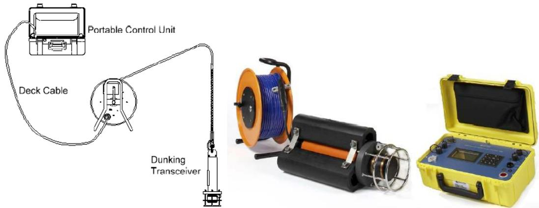
Figure 7.6: Portable Surface Control System [12]
