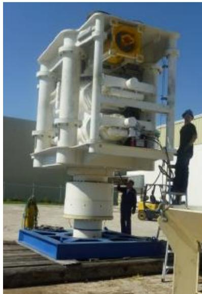
Figure 6.3: Subsea Isolation Device with MODSYS [42]
