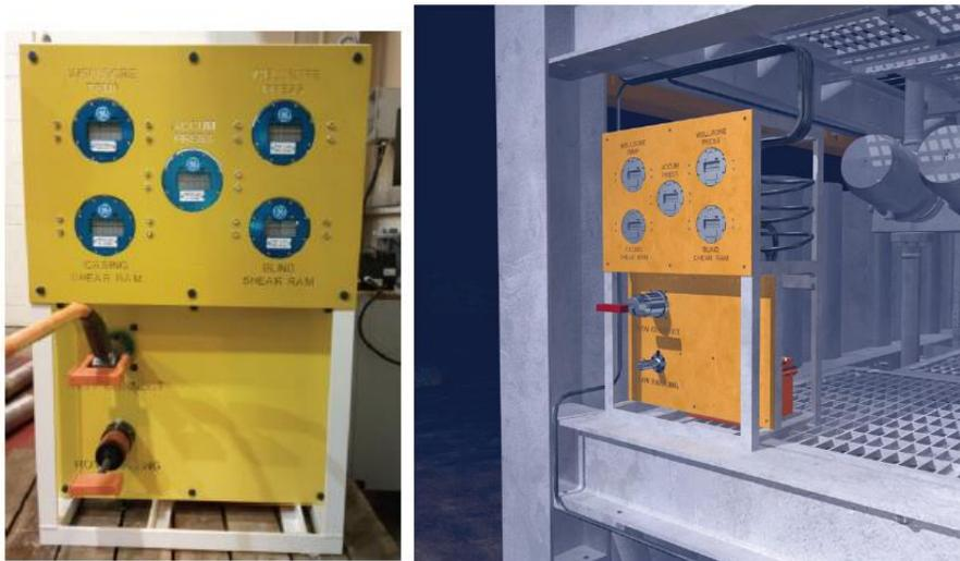
Figure 5.12: ROV Readable HPHT Display Panel [25]
