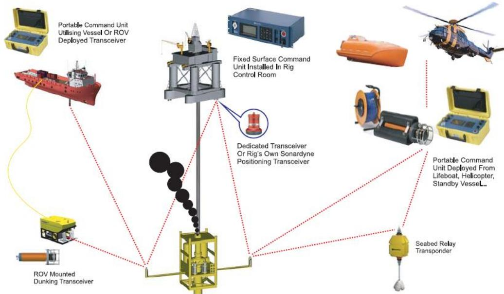
Figure 7.4: Application of Acoustic System [20]
