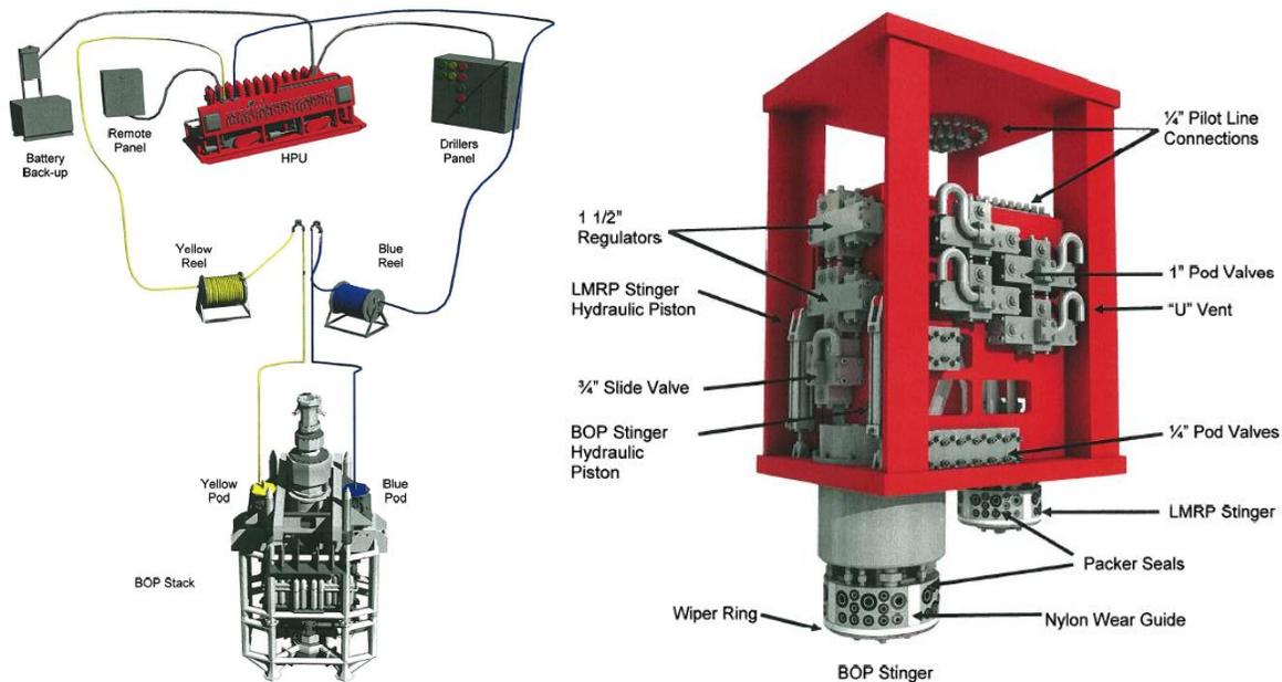
Figure 2.1: Conventional BOP Control System and Cameron Mark I Conventional Pod [2]
