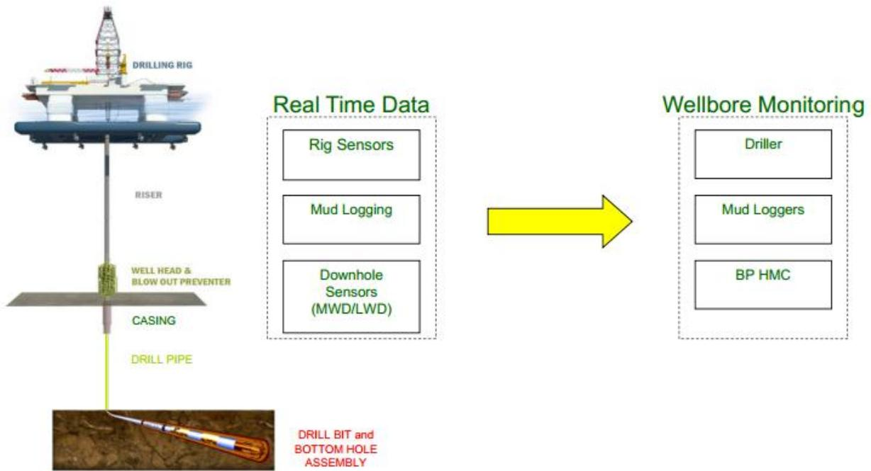
Figure 5.10: Real-Time Data & Well-Bore Monitoring Process [58]
