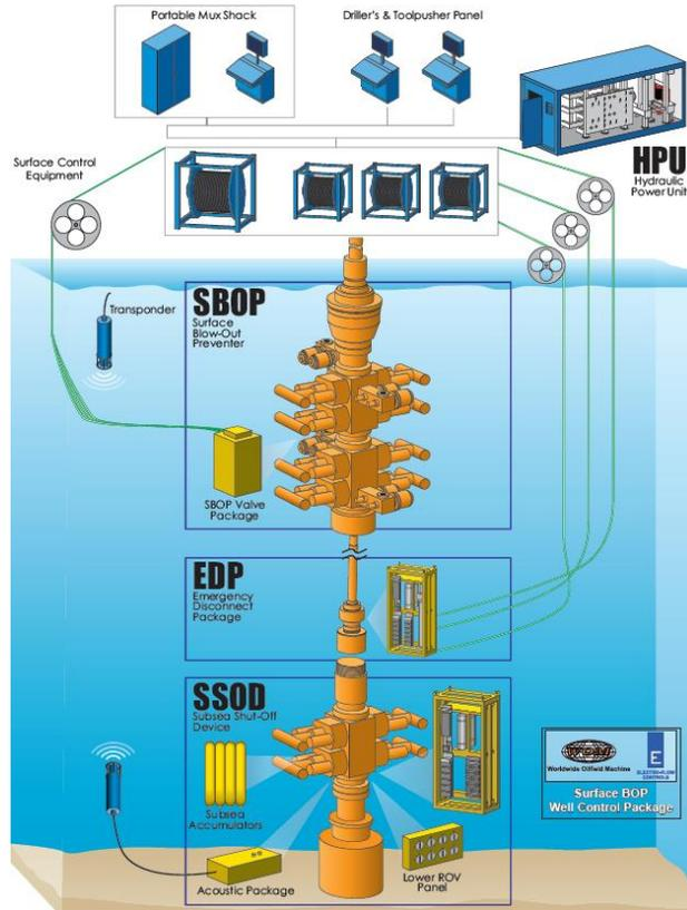
Figure 9.2: Surface BOP and SID/Subsea Shut-Off Device [26]
