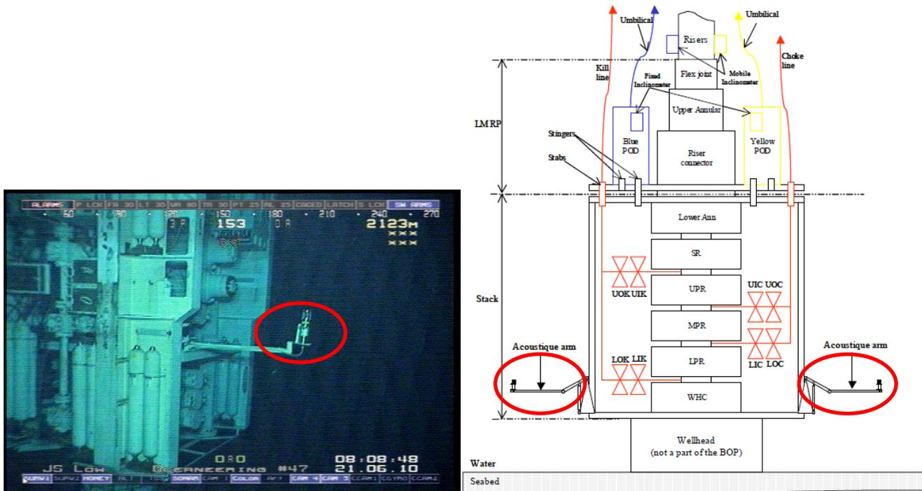
Figure 7.8: Placement of Transponders Attached to Arms on BOP [12, 19]
