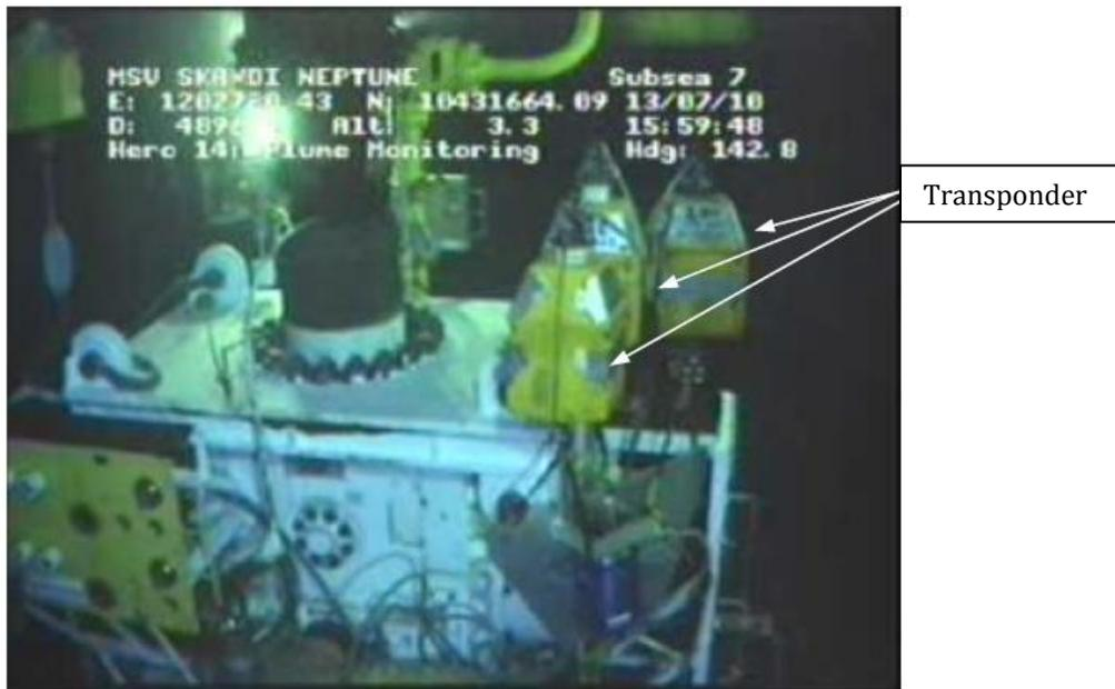
Figure 7.10: Transponders Operating Close to Subsea Blowout [12]
