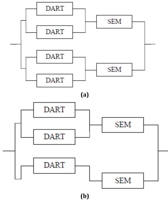
Figure 8.3: System Reliability Diagram with Enhanced Redundancy of Four DARTs [12]
