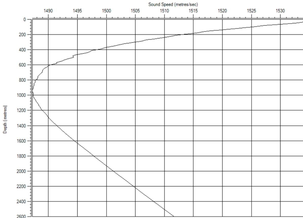
Figure 7.12: Sound Speed Variation with Water Depth [12]
