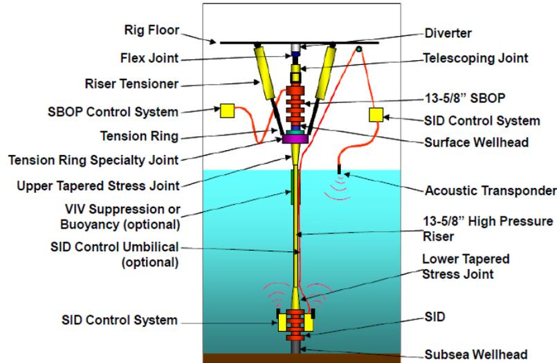
Figure 9.1: Surface BOP and SID/Subsea Shut-Off Device [18]
