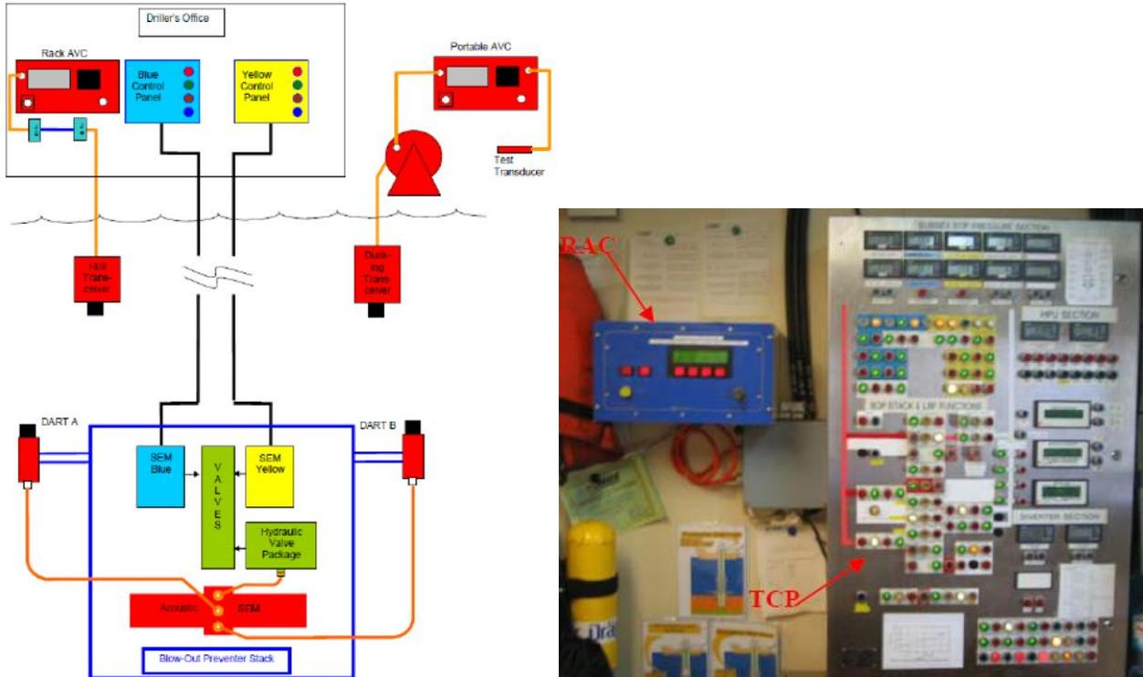
Figure 7.3: Acoustics System Schematic and Acoustic System (Blue Box) Hardwired on the Rig [21, 19]
