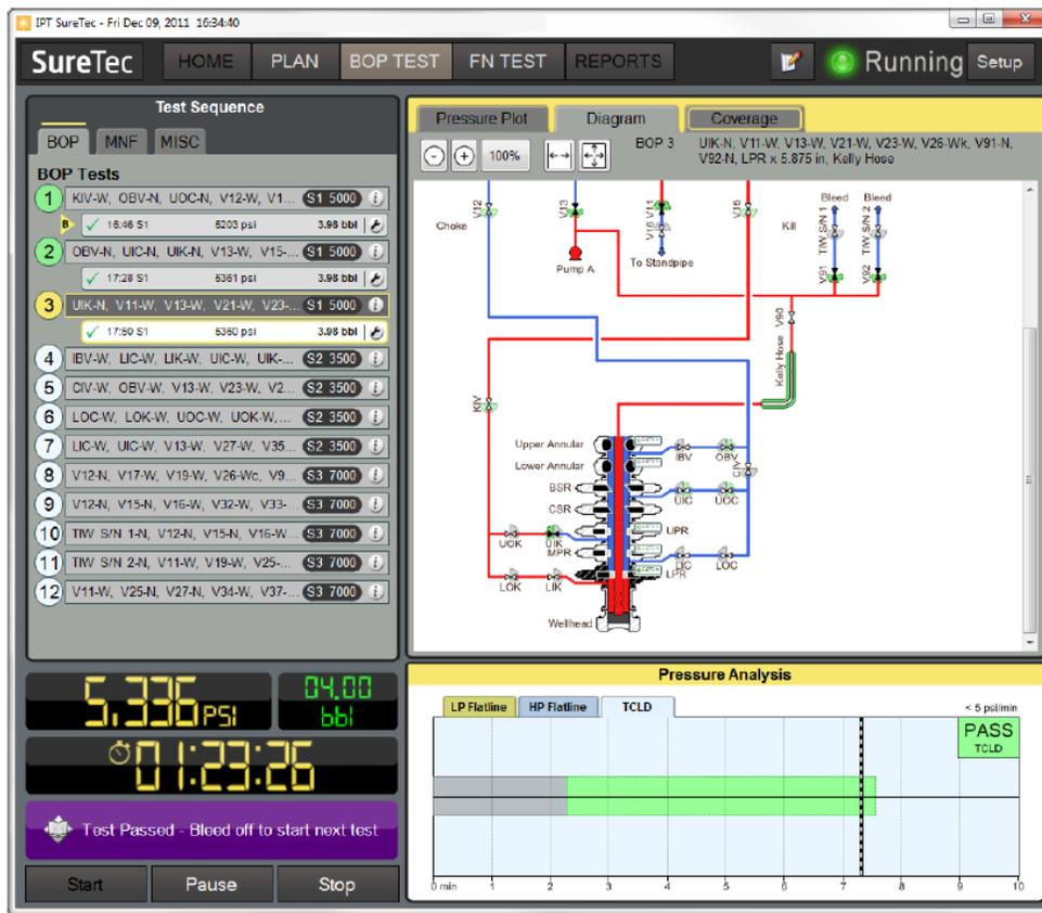
Figure 4.2: SureTec Testing Software Showing Valve Alignment and Pressure Paths [54]
