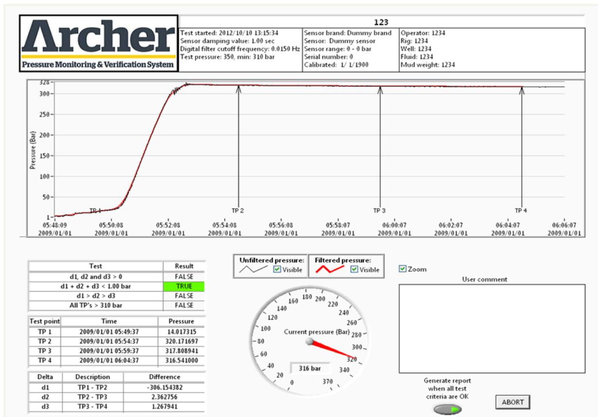
Figure 4.5: Snapshot of Pressure Test Results [43]
