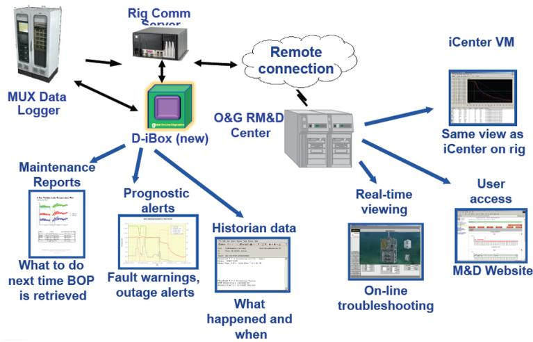
Figure 5.8: GE's Drilling iBox [30]
