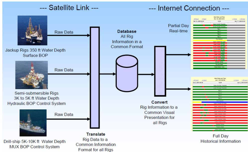
Figure 5.5: Multiple Rigs with Common Monitoring Display [41]
