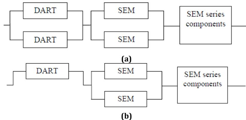
Figure 8.1: System Reliability Diagram for Standard System [12]
