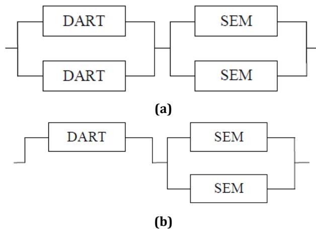
Figure 8.2: System Reliability Diagram for Dual Connector on Client Pod [12]
