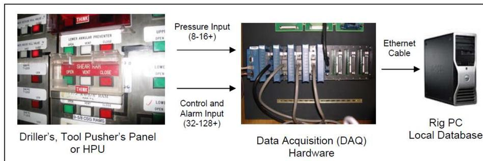
**Figure 5.1: BOP Monitoring Data Acquisition System [40]**
