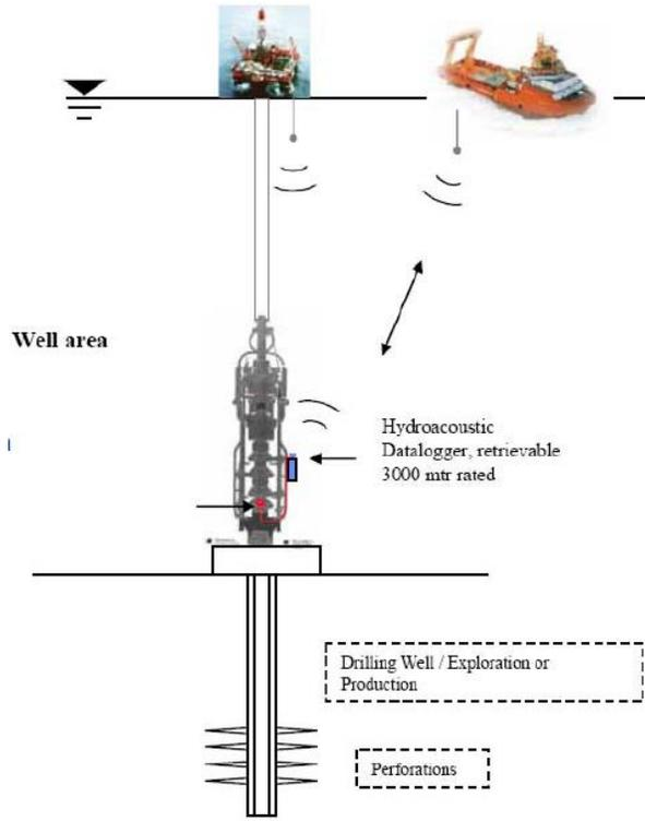
Figure 5.13: BOP Surveyor Operation [45]
