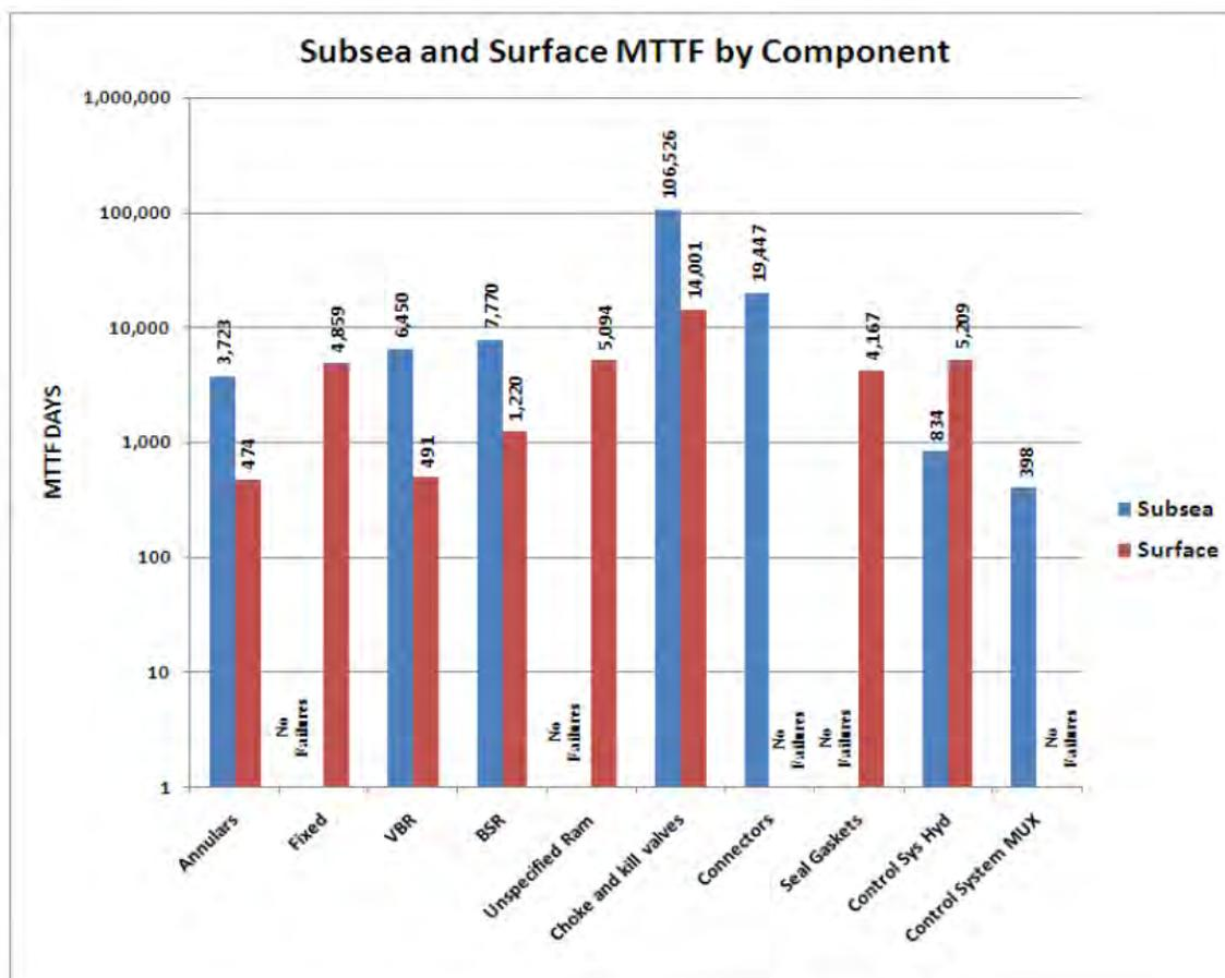
**Figure 2-10: Breakdown of MTTF for BOP Components Based on Failures Observed After Installation Testing (BOP in Service). Both Surface & Subsea Systems**
