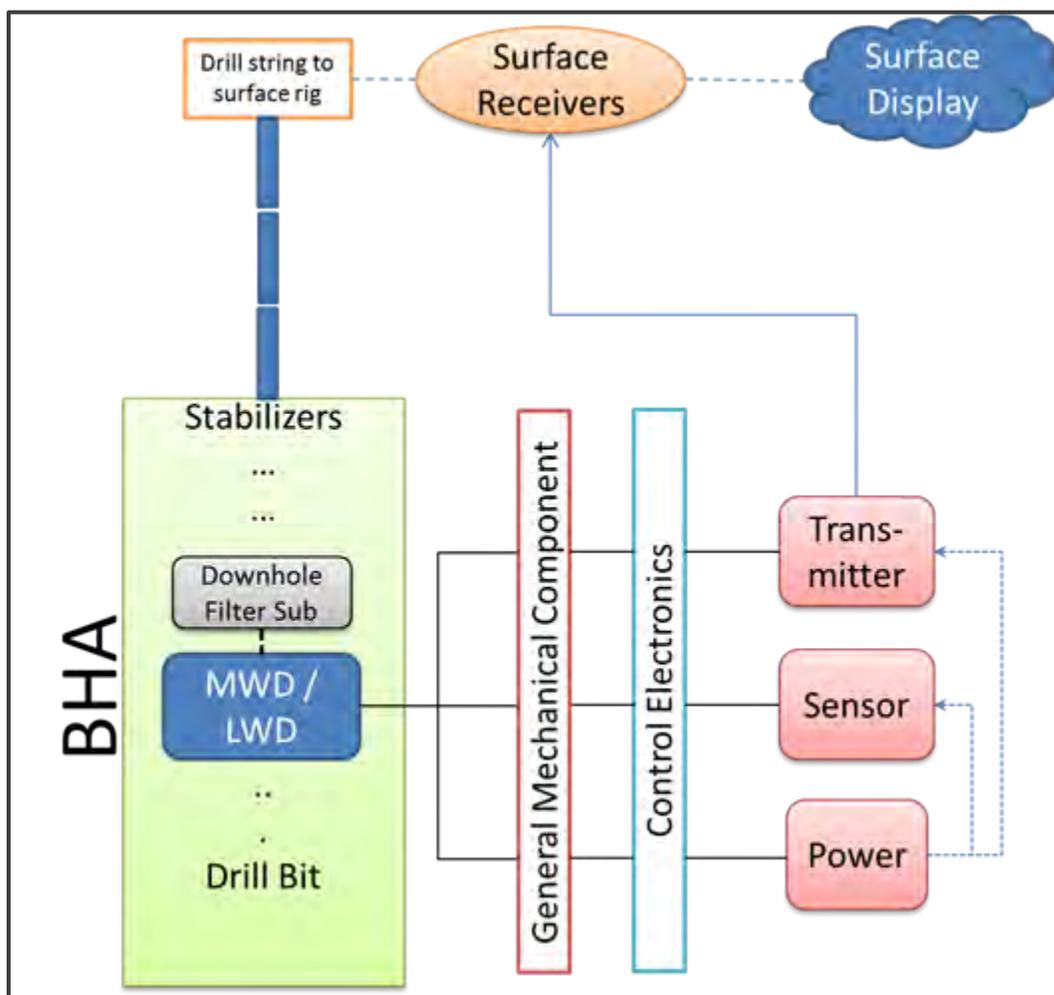
**Figure 4-5: General Schematic for MWD/LWD Systems**
