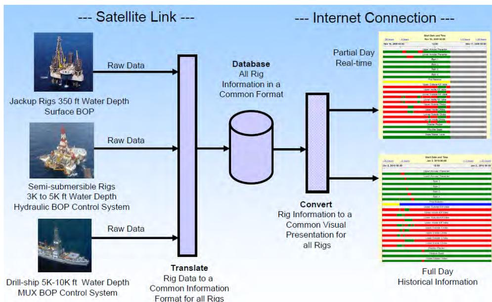
**Figure 3-12: Multiple Rigs with Common Monitoring Display [52]**
