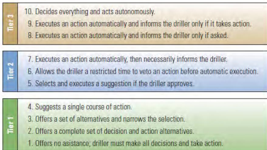
**Figure 2-18: Levels of Automation Ranging from Advisory Systems (Tier 3) to Full Automation where the Driller is Informed of the Actions Taken [95]**
