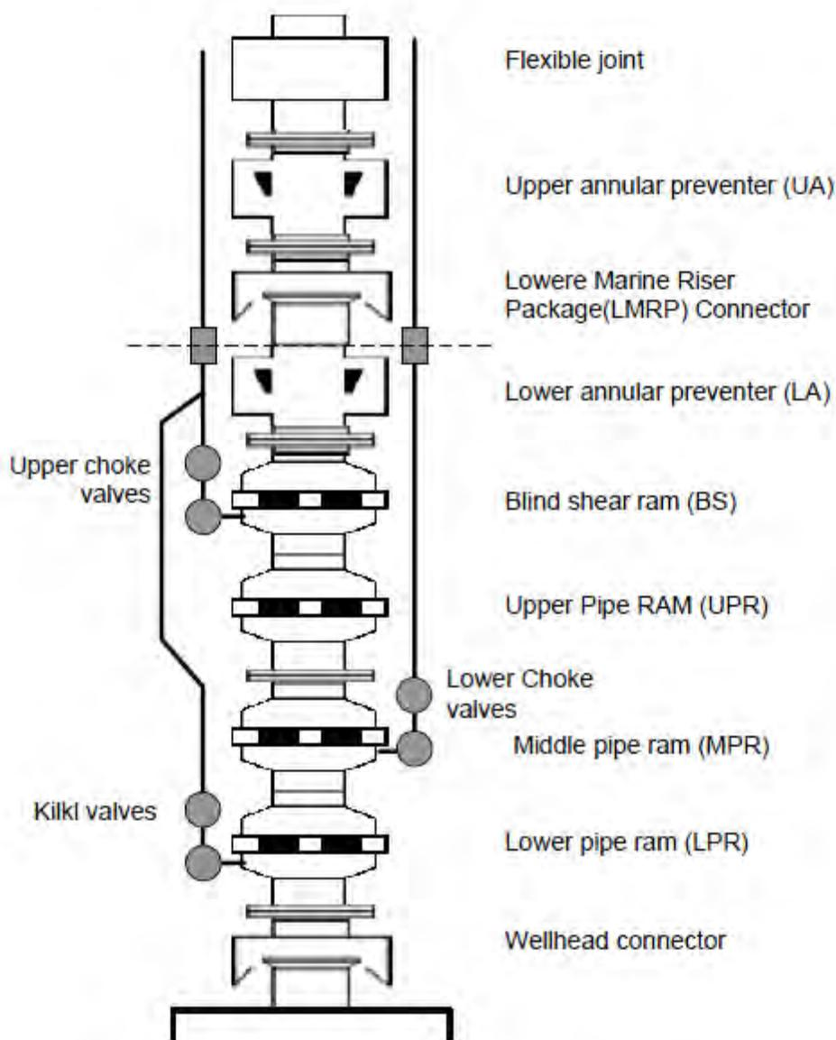
**Figure 2-7: Typical Configuration for a Subsea BOP Showing Choke & Kill Lines & Associated Valves [72]**
