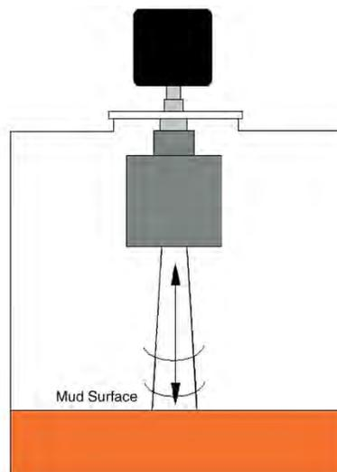
**Figure 3-2: Pit Monitor Sensor [39]**
