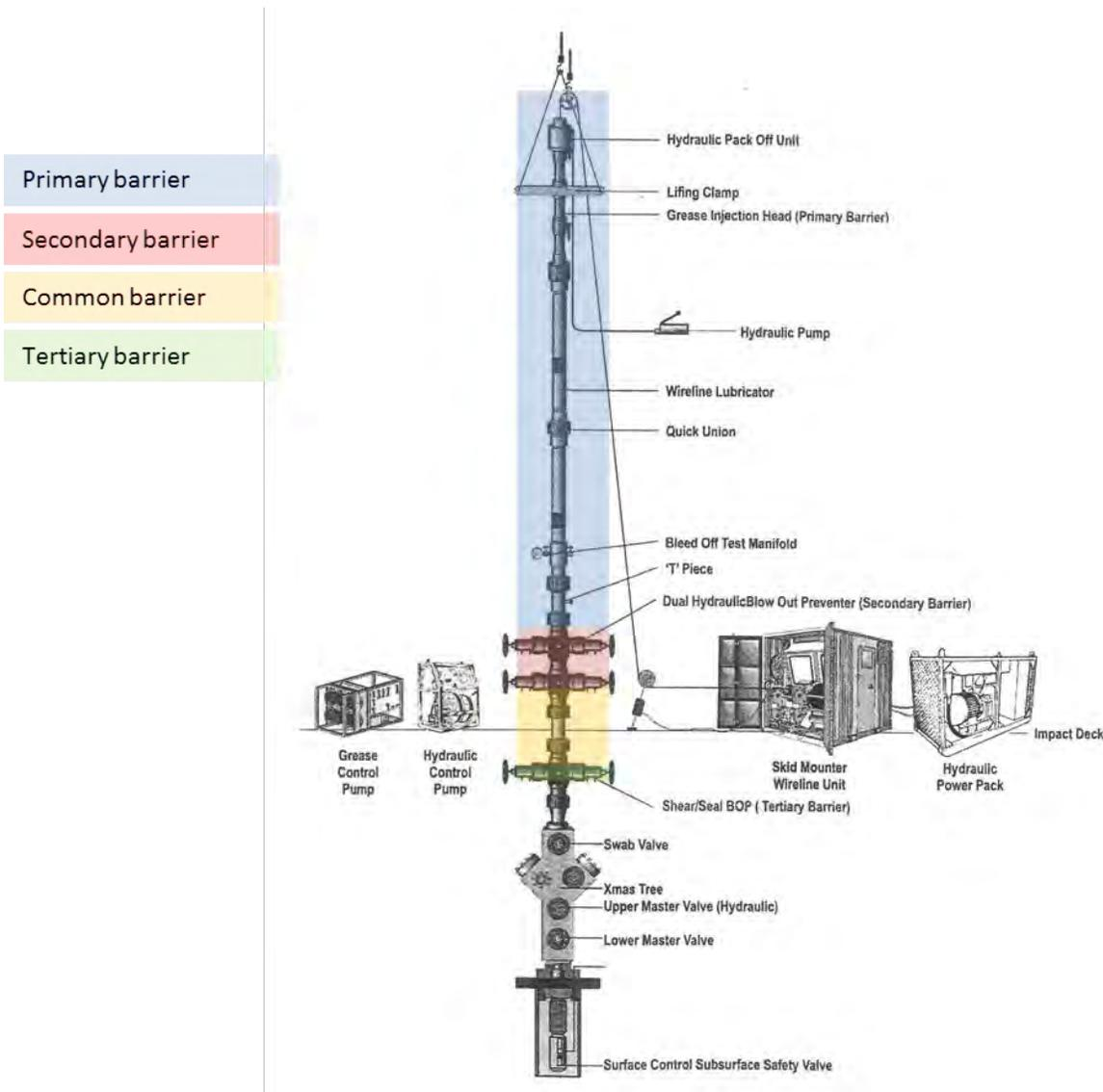
**Figure 2-12: Braided Line (E-line) Rig Up Showing Barrier Elements [78]**
