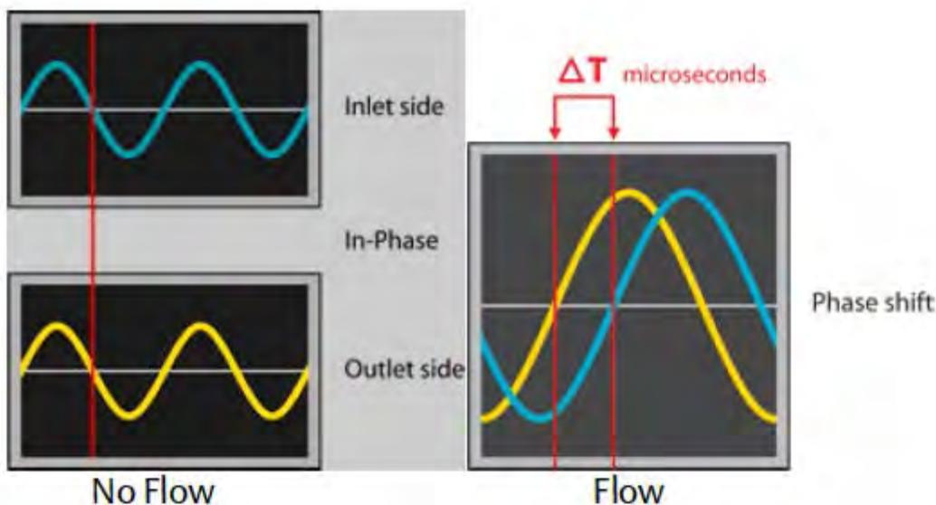
**Figure 2-22: Phase Shift between Inlet and Outlet Side Pickoff Coils during Flow Conditions [102]**
