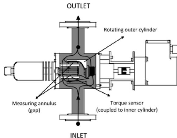
**Figure 2-19: Process Viscometer Model TT-100 [100]**
