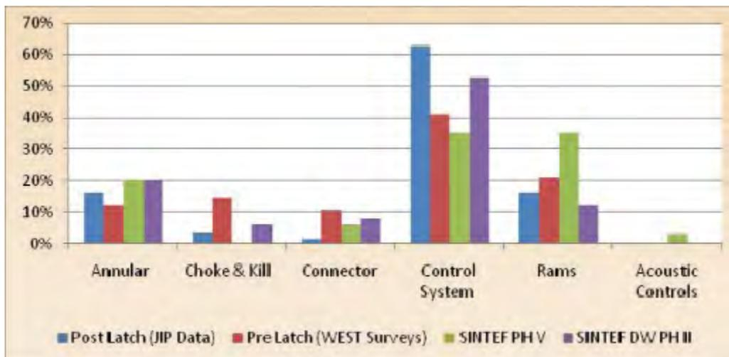
**Figure 2-8: Failure Distribution of Subsea BOP Components [75]**
