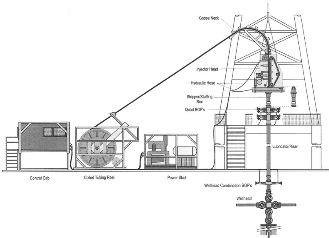
**Figure 2-14: Coiled Tubing Rig Up on a Surface Tree Showing Pressure Control Equipment [78]**
