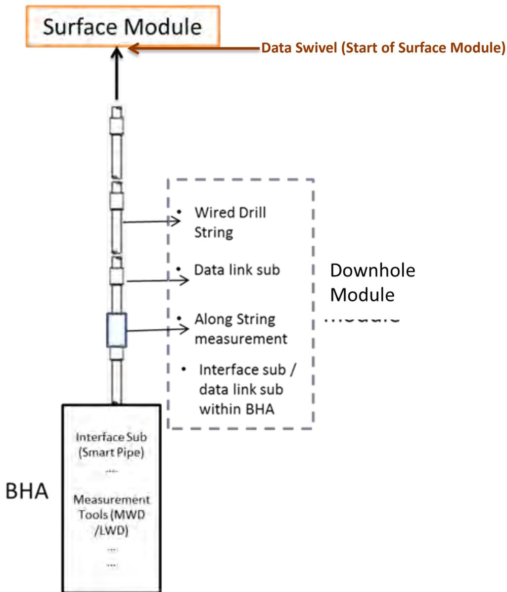
Figure 4-6: General Schematic for Wired Drill Pipe System
