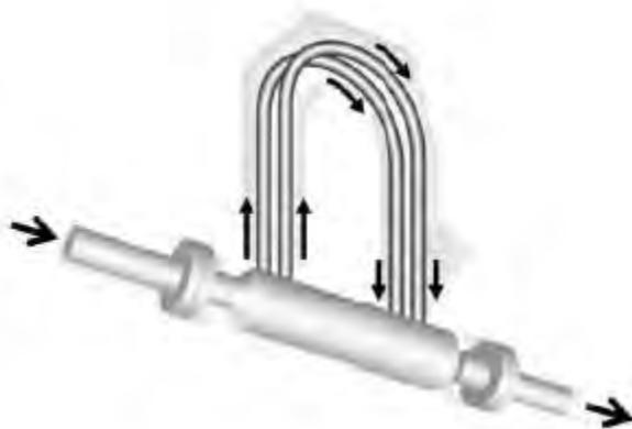
**Figure 2-20: Coriolis Flow Loop Paths [102]**
