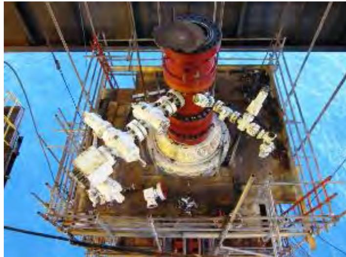
**Figure 2-40: Rotating Control Device**
