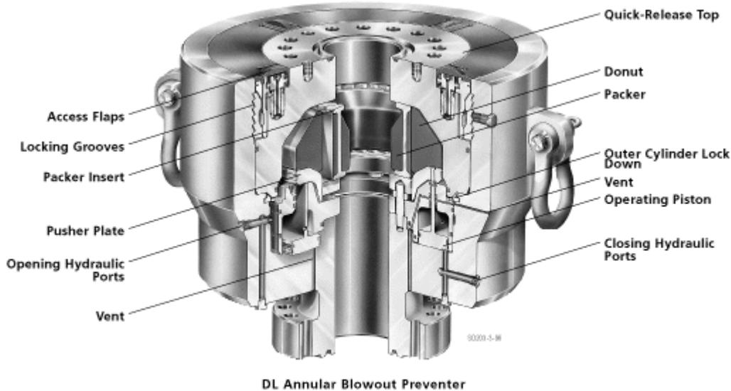
**Figure 2-5: Cameron DL Annular Blowout Preventer**
