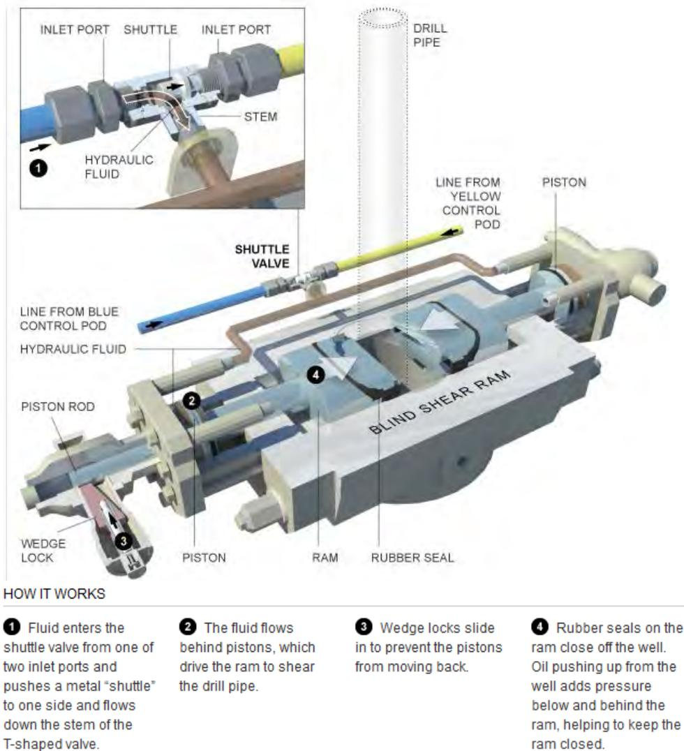
**Figure 2-6: Illustration of a Shear Ram BOP [71]**
