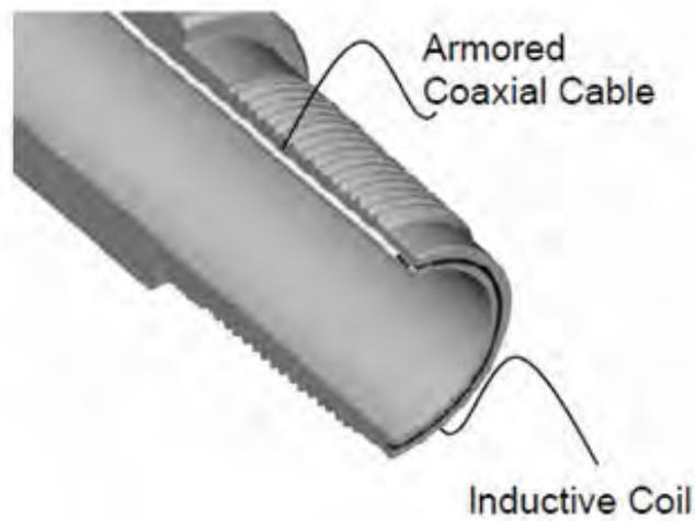
**Figure 3-4: Wired Drill Pipe with Armored Coaxial Cable Design [46]**
