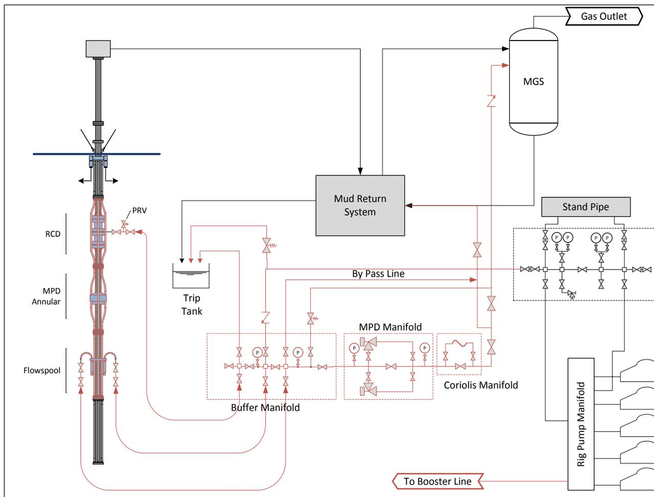
**Figure 4-4: General Schematic for Floater Rig MPD System<sup>18</sup>**
