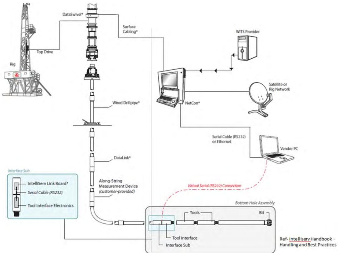
**Figure 4-2: Sample Schematic of a Wired Drill Pipe System (NOV, 2013 [7])**
