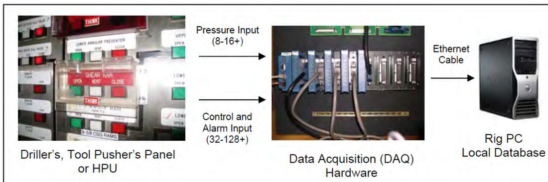
**Figure 3-8: BOP Monitoring Data Acquisition System [51]**
