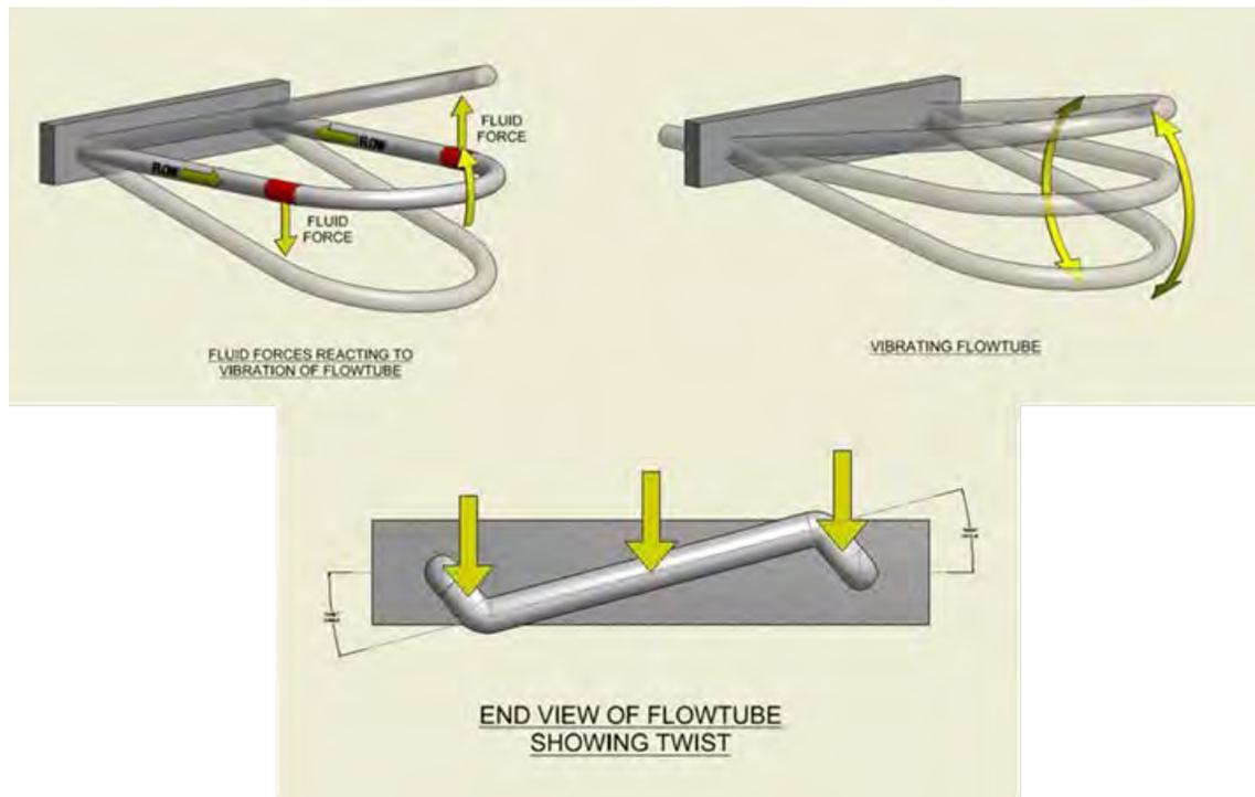
**Figure 2-21: Function of Coriolis Flowmeter Illustrating Twist Induced under Flow Conditions Due to Coriolis Effect [103]**
