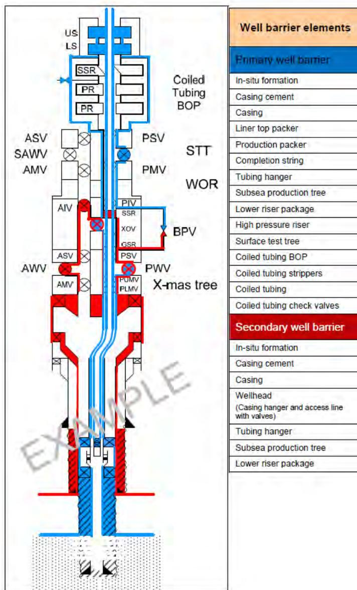
**Figure 2-2: Barrier Envelope for CT Operations on Vertical Subsea Tree with LRP [10]**
