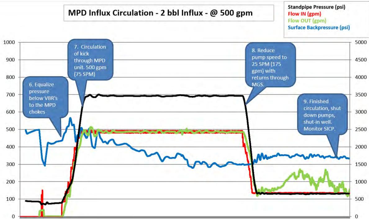
**Figure 2-39: Circulation of Influx through MPD System**
