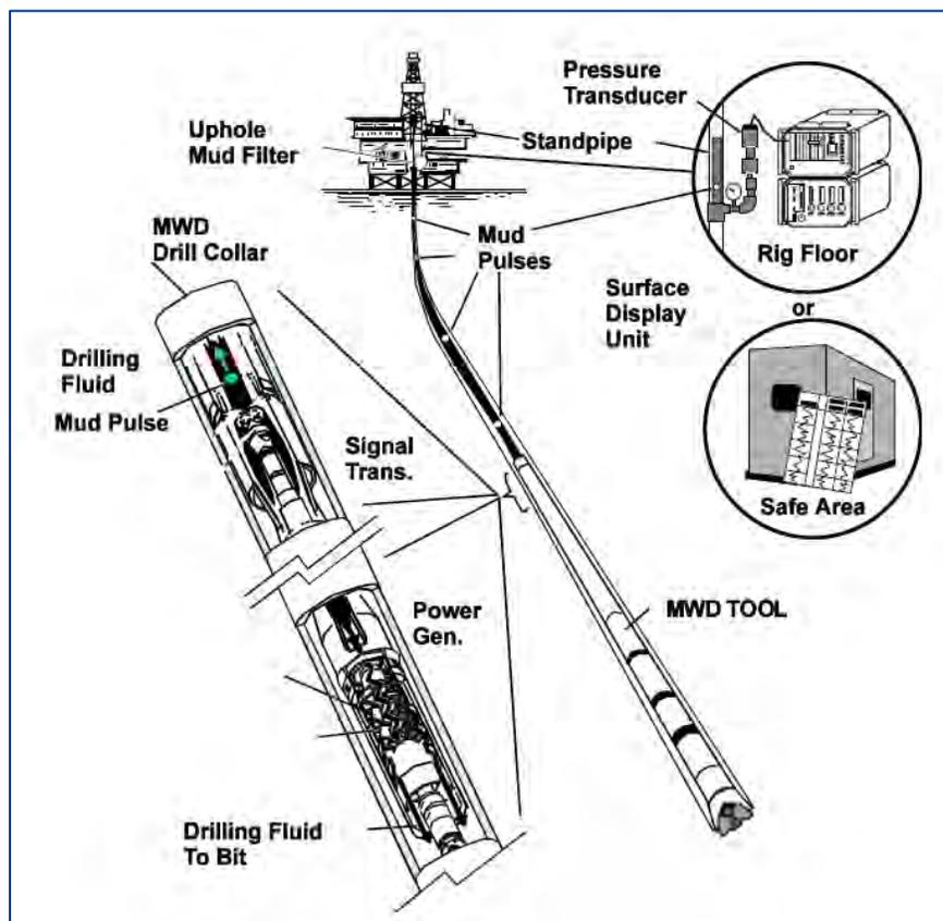
Figure 4-1: Example Illustration of a Typical MWD/LWD System (Baker Hughes, 2008 [3])
