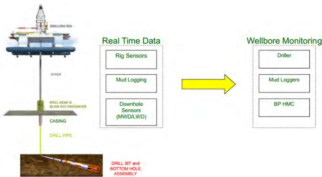
**Figure 3-16: Real Time Data and Wellbore Monitoring Process [55]**
