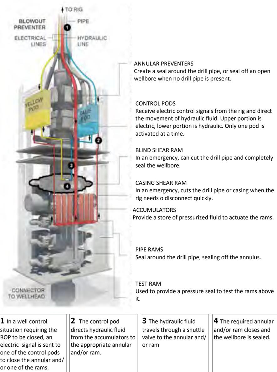
**Figure 2-4: Closing of the BOP When a Kick Is Detected**
