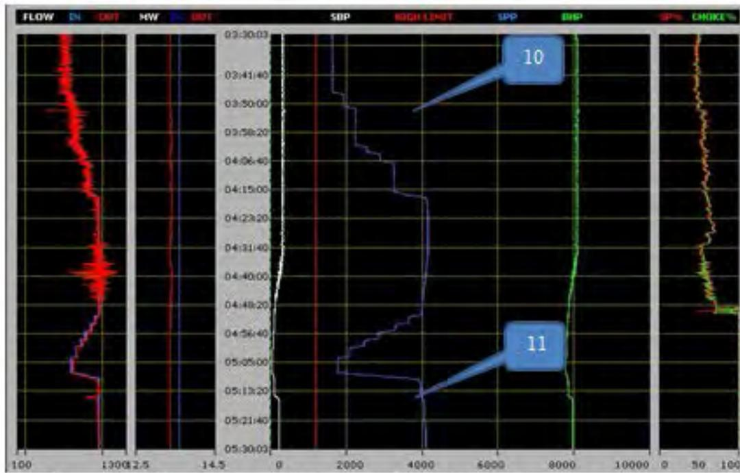
Figure 2-37: Circulating out Influx 1. Complete Bottoms Up.
