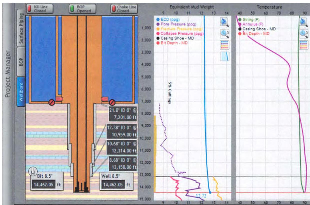
**Figure 2-24: Screenshot of Safevision Display Showing Interpreted Log Data [106]**
