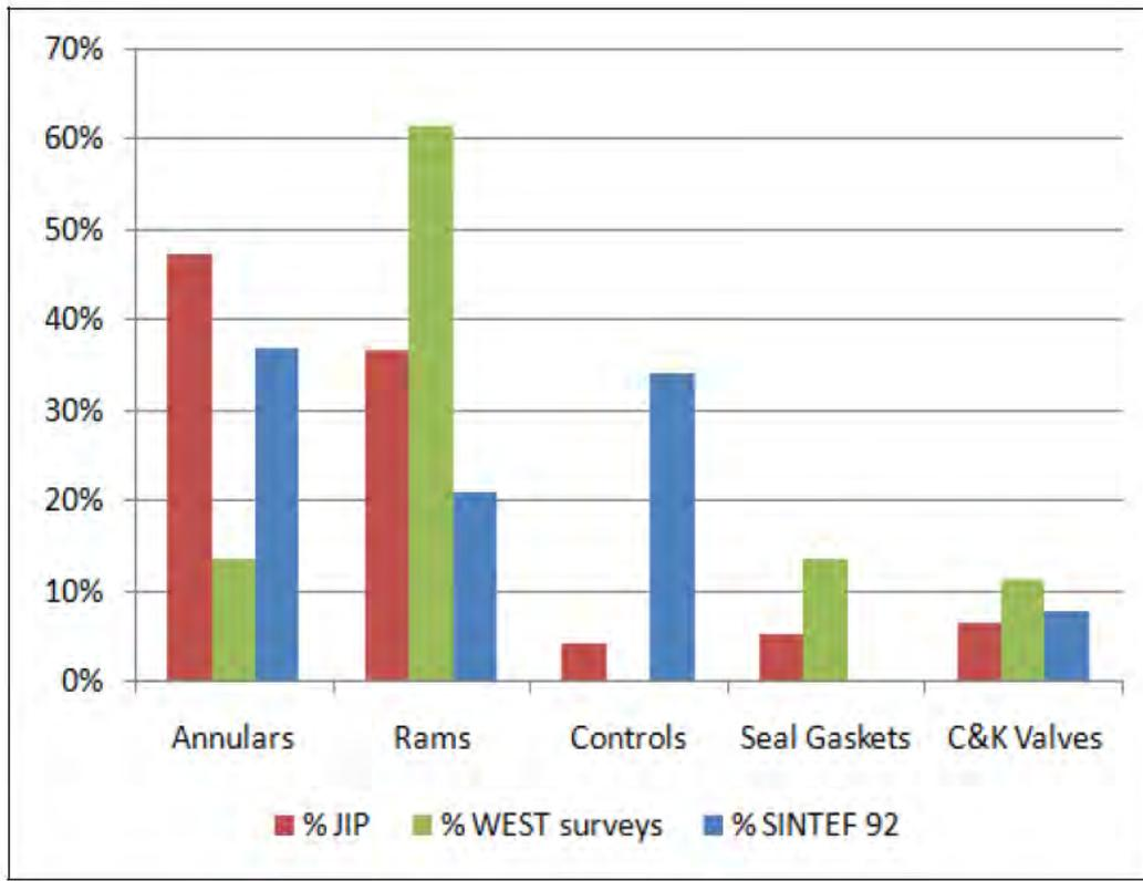
**Figure 2-9: Failure Distribution of Surface BOP Components [76]**
