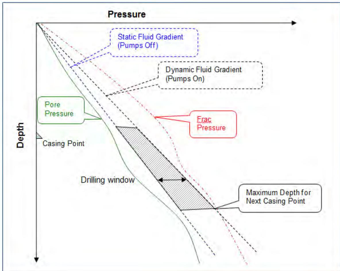
**Figure 2-3: Conventional Drilling Fluid Gradients & Casing Setting Points [1]**
