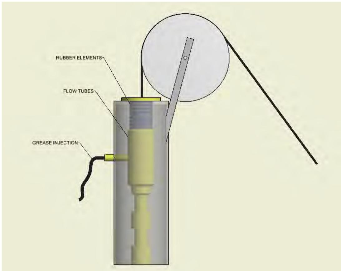
**Figure 2-13: Schematic of Grease Injector [79]**
