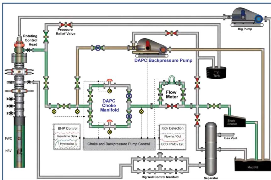
**Figure 2-27: Schematic Showing Applied Backpressure MPD Equipment (Courtesy of Schlumberger) [1]**
