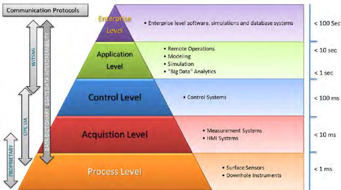
**Figure 2-15: Modified Purdue Automation Pyramid [83] Showing Transition from Process Level (Measurement Instrumentation) to Enterprise (Remote) Software Systems**
