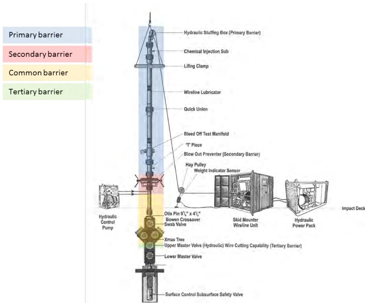
**Figure 2-11: Slickline Rig Up on a Surface Tree Showing Pressure Control Equipment [78]**
