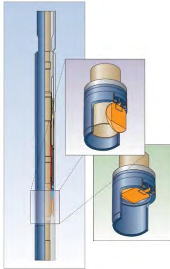
**Figure 3-17: Surface Controlled Subsurface Safety Valve (SCSSV) [60]**
