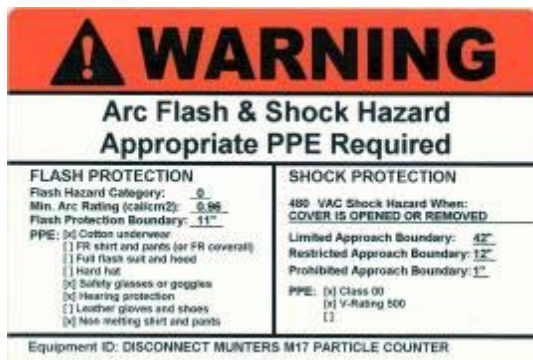
Figure 29 – Example Arc Flash Warning Label
