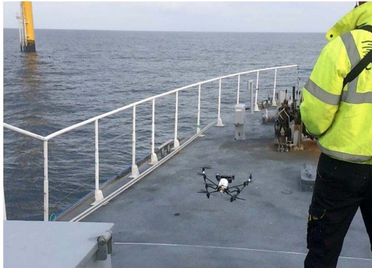
Figure 2 – MetMast Inspection with Drone 55
