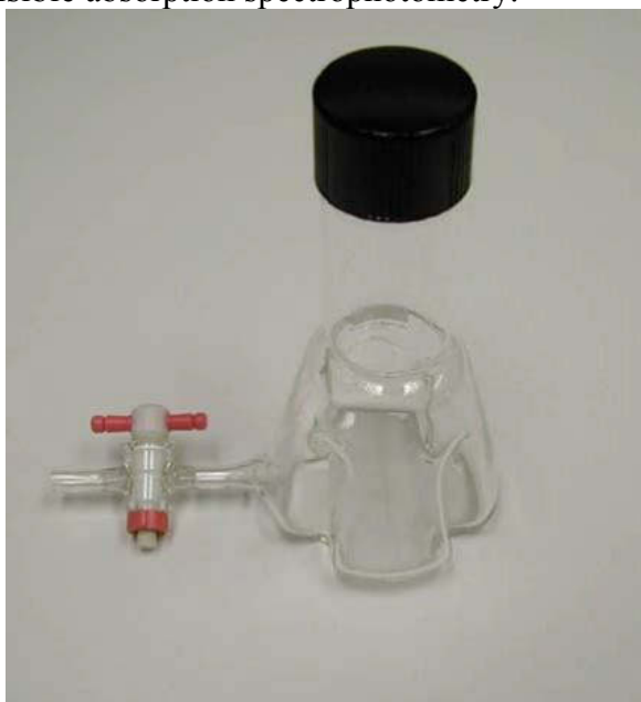
Figure 1. Photograph of the baffled trypsinizing flask.
