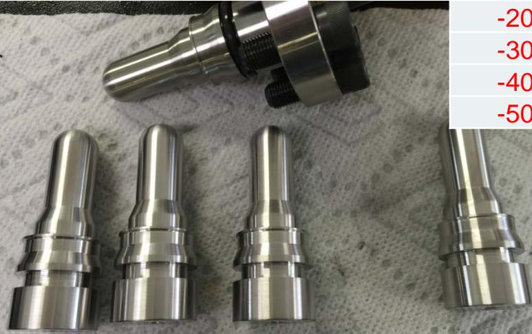
Actual dimensions of parts have been used in the report to correct values of the nominal clearances
