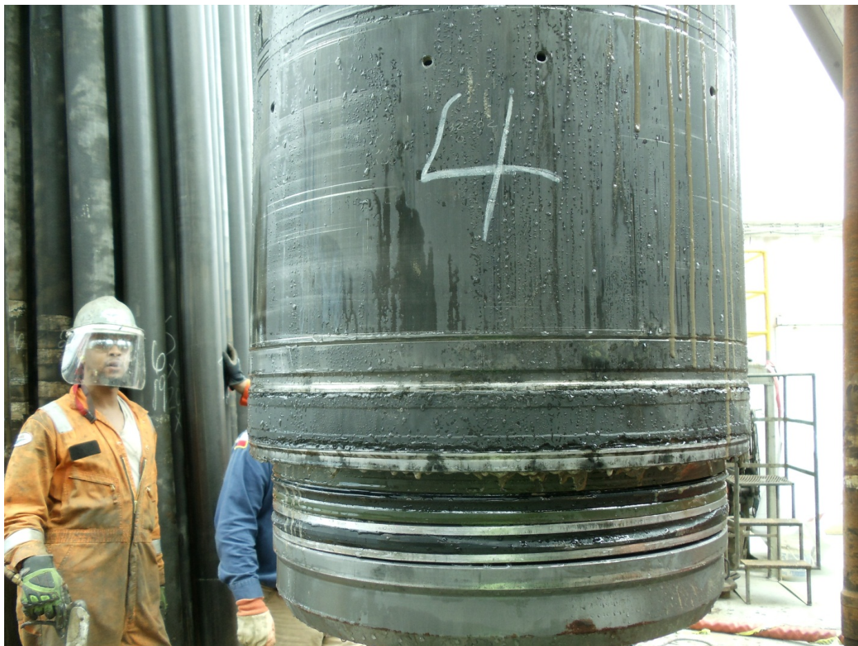
FIGURE 2: PULLED SUB MUDLINE CASING HANGER SEAL
