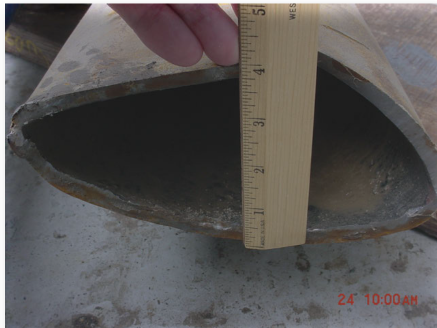
Picture of sheared 6-5/8" drill pipe pulled to the surface
