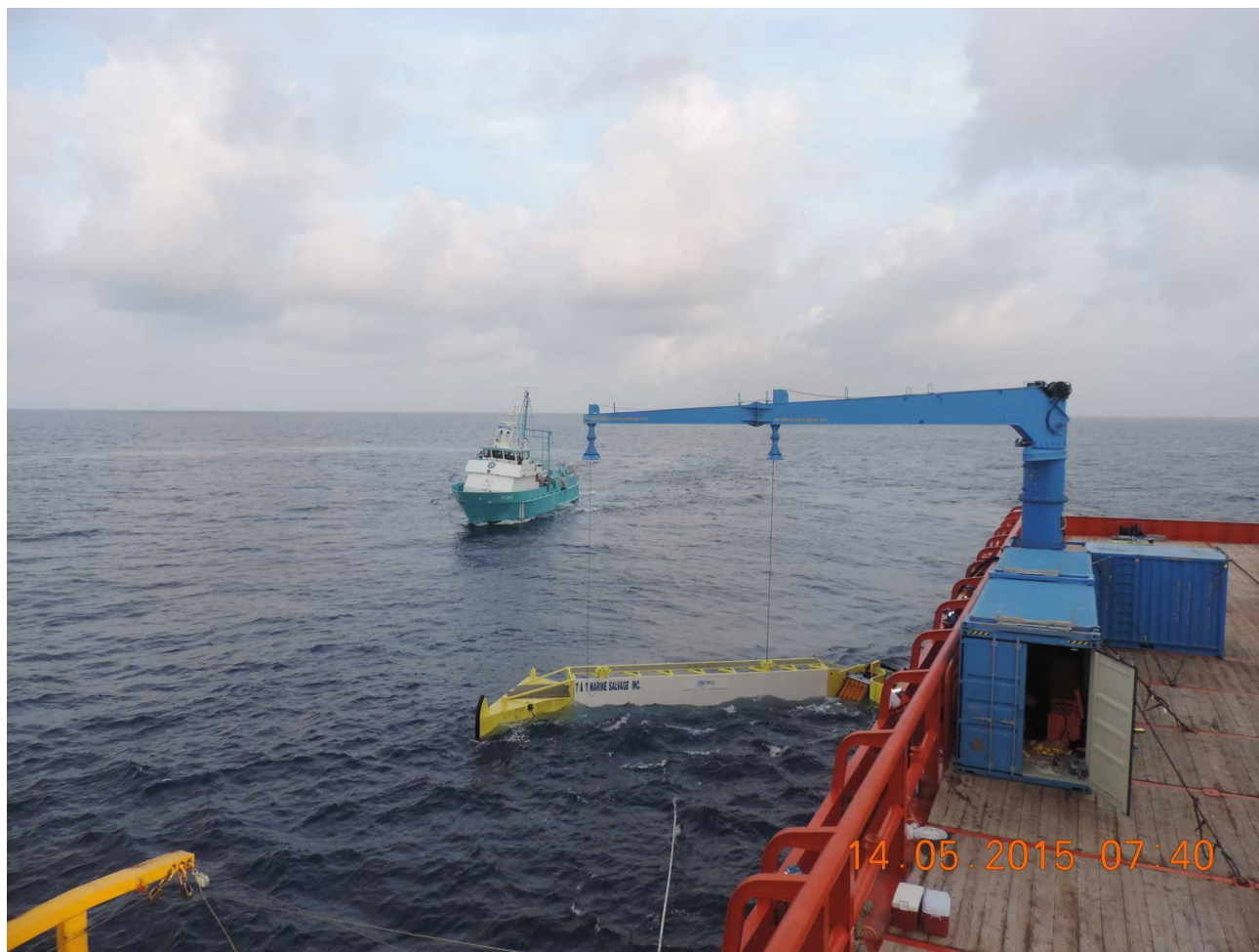
Figure 14. Example of a Rigid Arm System. (Photograph courtesy of Clean Gulf Associates, KOSEQ Rigid Sweeping Arms - Clean Gulf Associates ).
