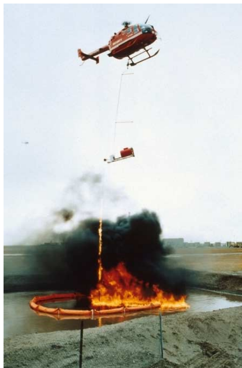
Figure 6. Heli-torch and Fire-Resistant Boom Test
