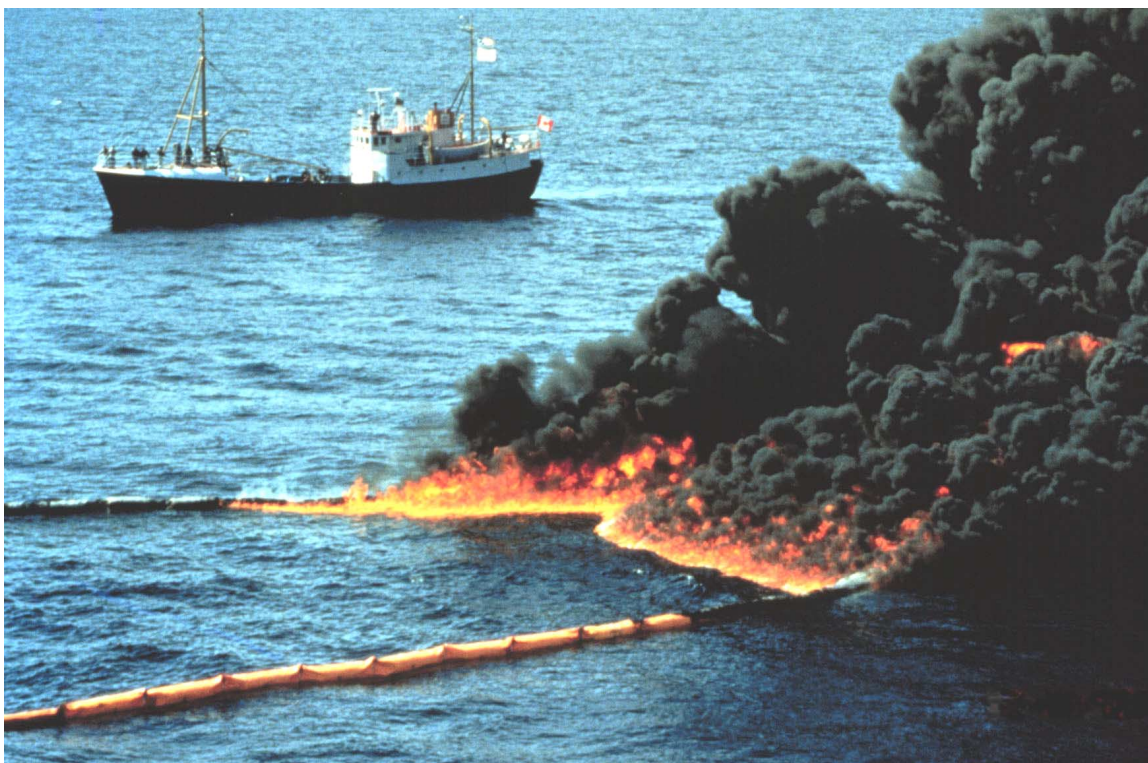
Figure 1. ISB Operation with Fire-resistant Boom
