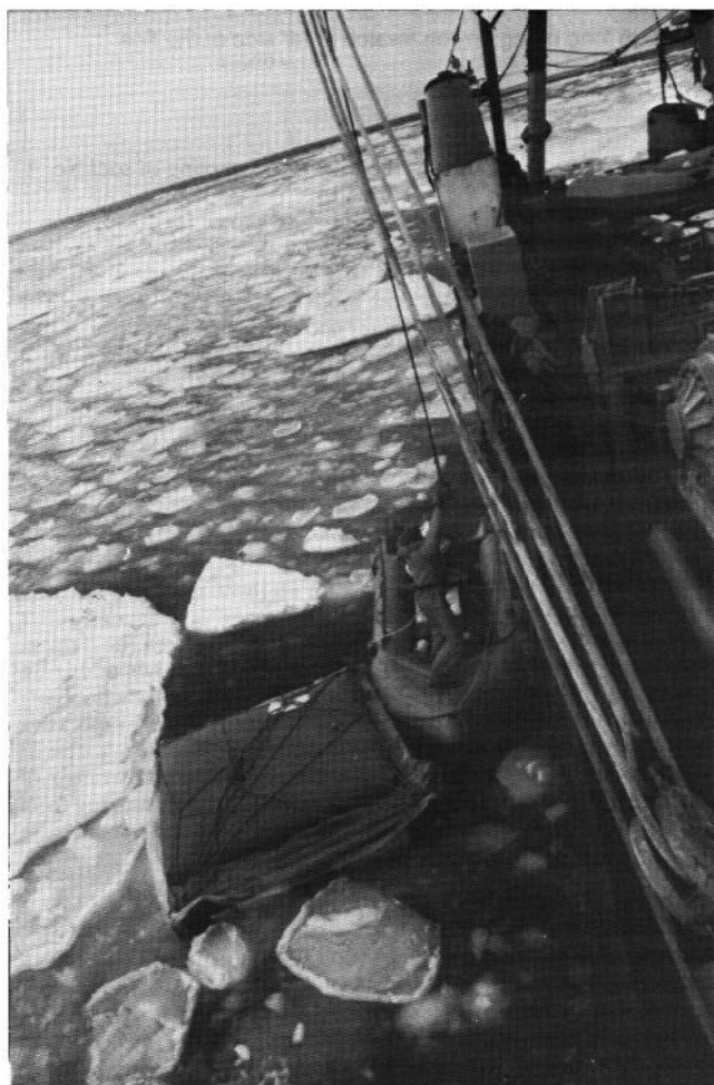
Figure 3. The oil-filled raft for spill No. 1
