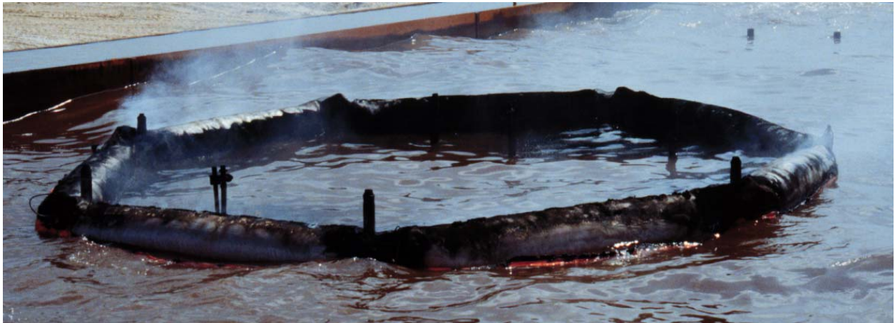
Figure17. Boom 2, after burning
