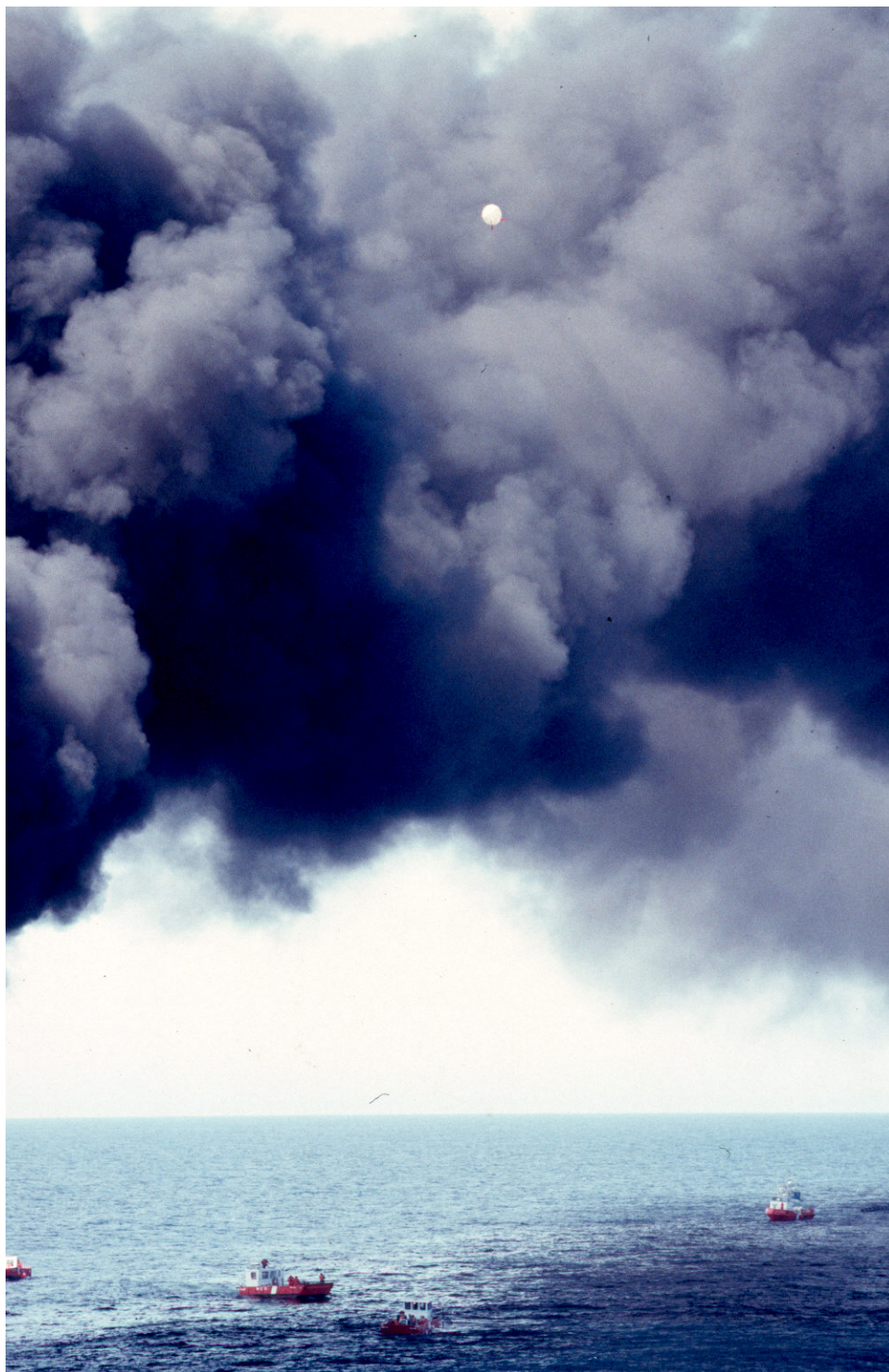
Fig. 8. NIST samples smoke plume approximate 300 m downwind of the burning oil using instruments suspended beneath the mini-blimp (top-center of photograph above smoke plume) tethered to support vessel (lower-left).
