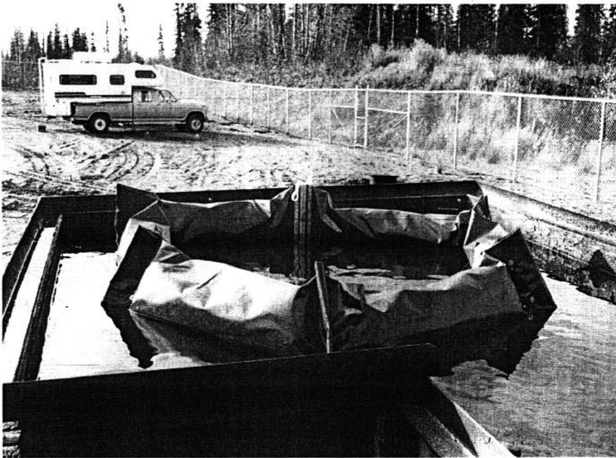
FIGURE 5 FIRE BOOM IN POSITION PRIOR TO IGNITION OF CRUDE OIL
