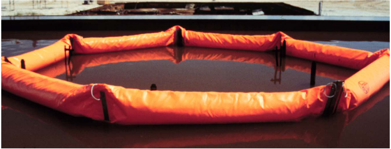
Figure 15. Boom 2, before burning
