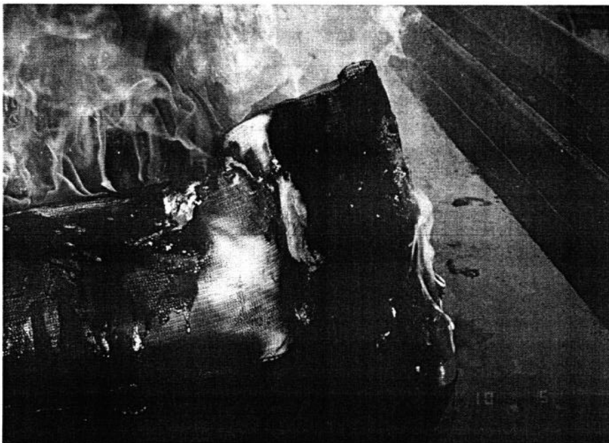
FIGURE 7 CLOSEUP VIEW OF THE FIRE BOOM AS THE LAST PORTION OF THE SACRIFICIAL LAYER IS BURNED OFF
