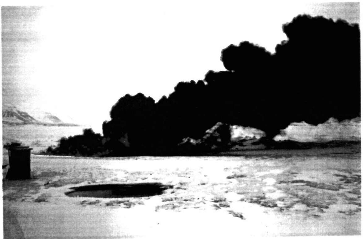
Figure 6.8: Experiment L1: 25% evaporated, 50% water-in-oil emulsion, 0% ferrocene
