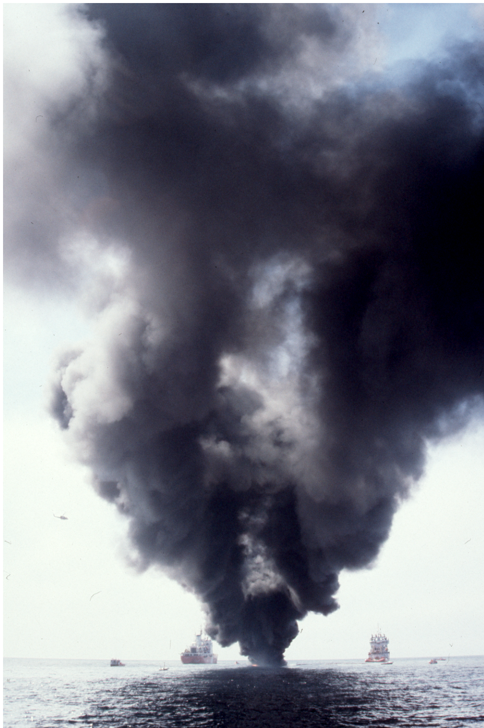
Fig. 26. Photograph taken from about 200 m downwind of the Newfoundland Offshore Burn Experiment (NOBE) showing the two large counter-rotating vortices which characterize the structure of the rising smoke plume.
