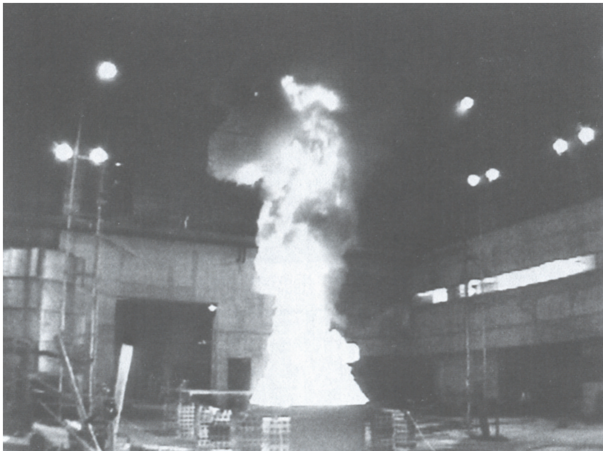
Fig. 3. Two-meter diameter crude oil fire in NRIFD, Japan test hall.
