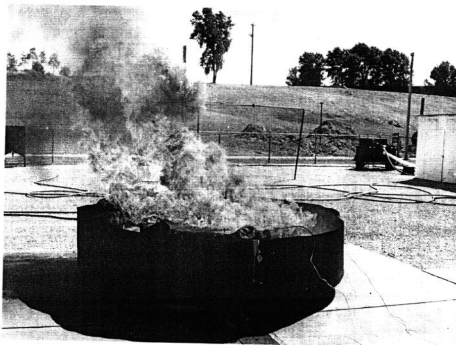
FIGURE 3 FIRE BOOM AFTER IGNITION OF HEPTANE IN 6-HOUR BURN TEST
