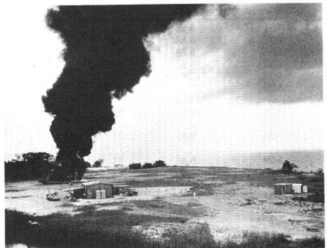
Figure 4. 17.2 meter effective diameter Louisiana crude oil fire at the USCG Safety and Fire Test Detachment mesoscale test facility in Mobile, Alabama
