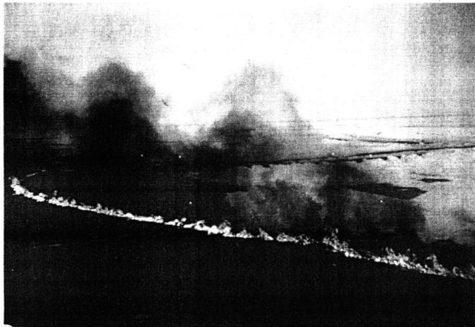
FIGURE 4 NEARLY CONTINUOUS PATH OF BURNING GELLED GASOLINE FOLLOWING SLOW, LOW-LEVEL PASS OF THE HELITORCH
