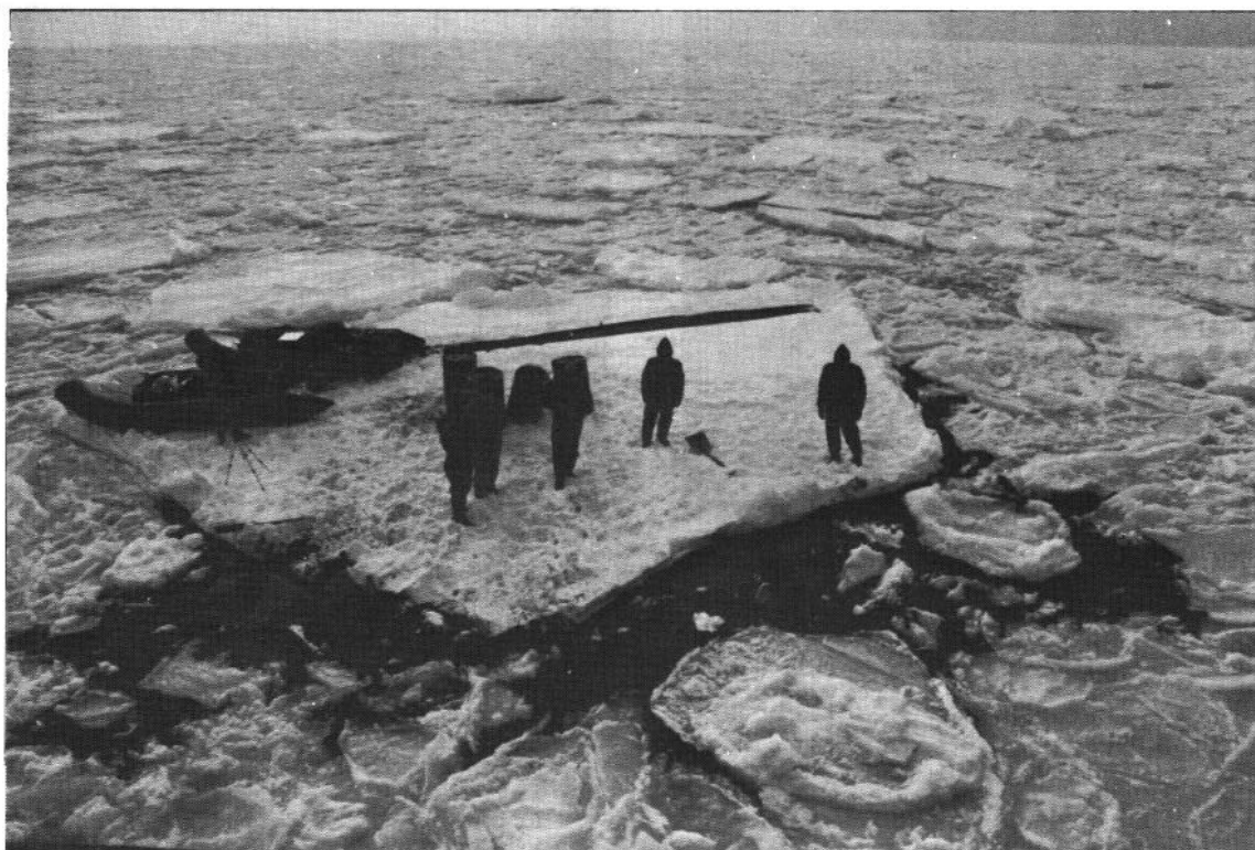
Figure 5. Oil release from drums on ice floe for spill No. 3—note the 10 m long orange nylon swatch at far side of the floe to provide scale for aerial photography
