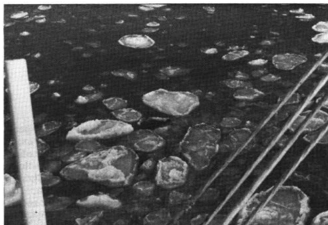
Figure 13. Oil on top of small ice pancake (near center of photo) amidst sheen
