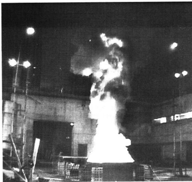
Figure 3. Two meter diameter Murban crude oil fire at Fire Research Institute in Japan
