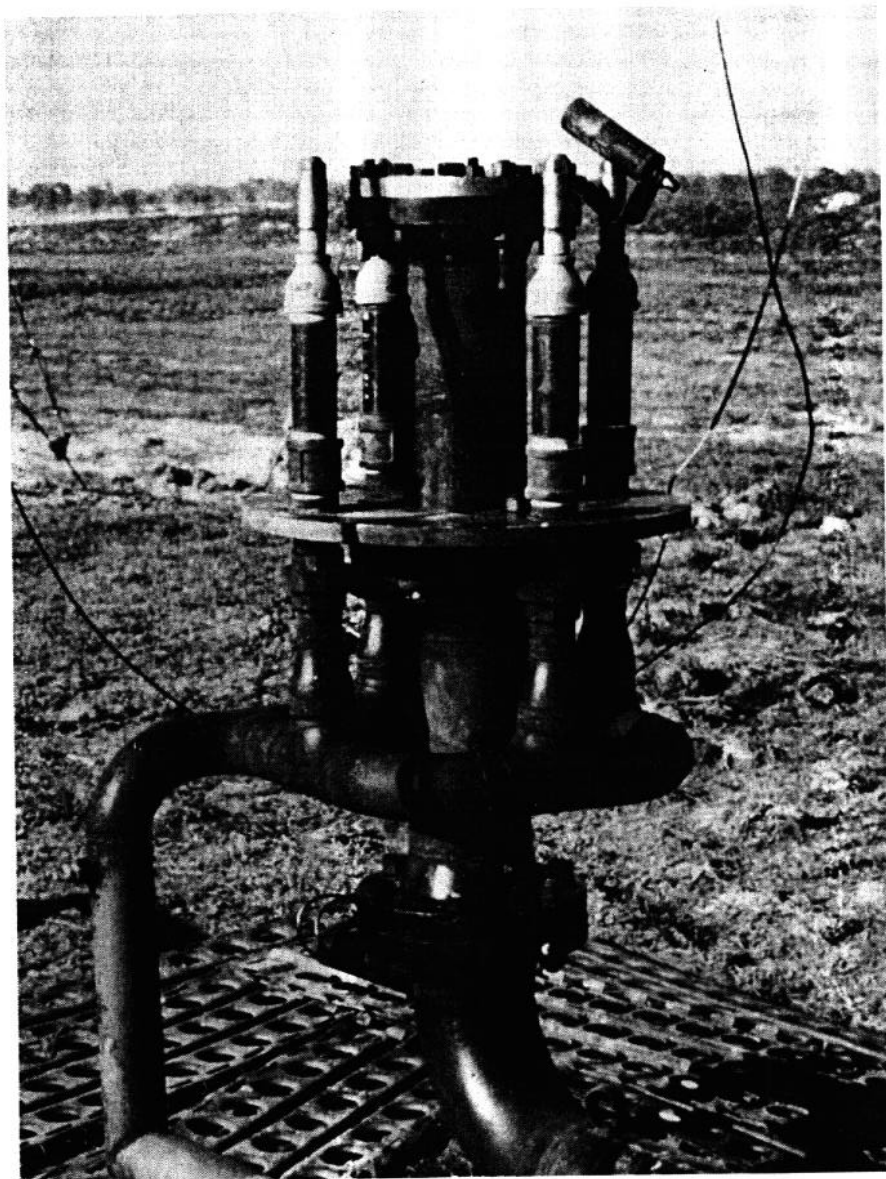
External water injection configuration features four nozzles spraying parallel to the gas flow (Fig. 3).
