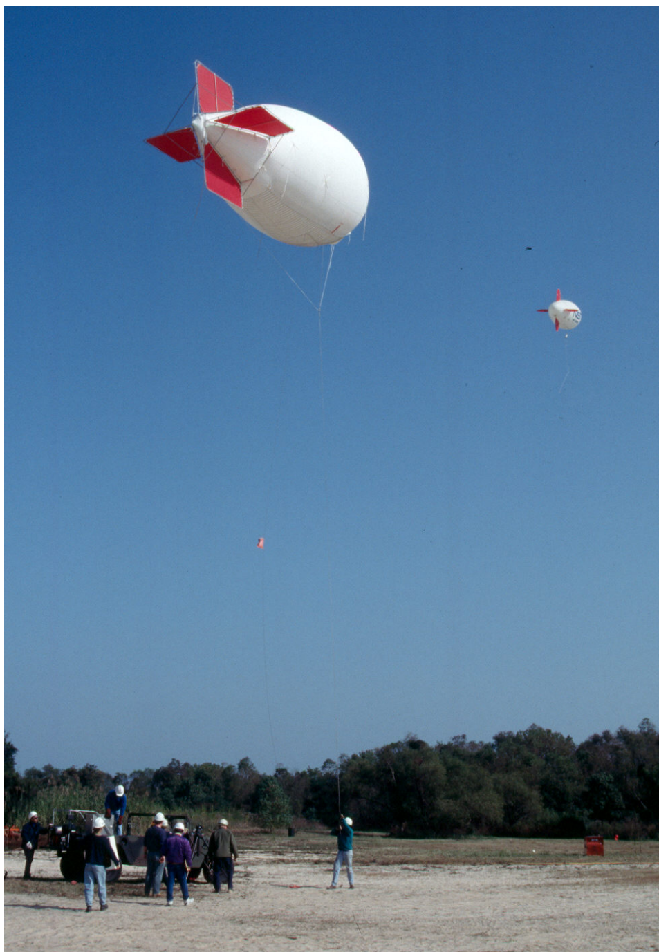
Fig. 6. Mini-blimp used to support instrument packages for smoke plume gas and particulate sampling.
