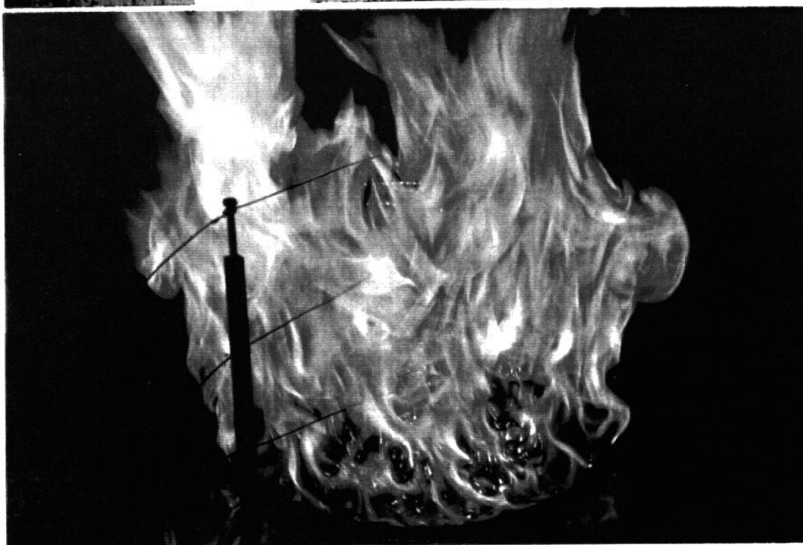
Figure 3.5: Thermocouples in flames
