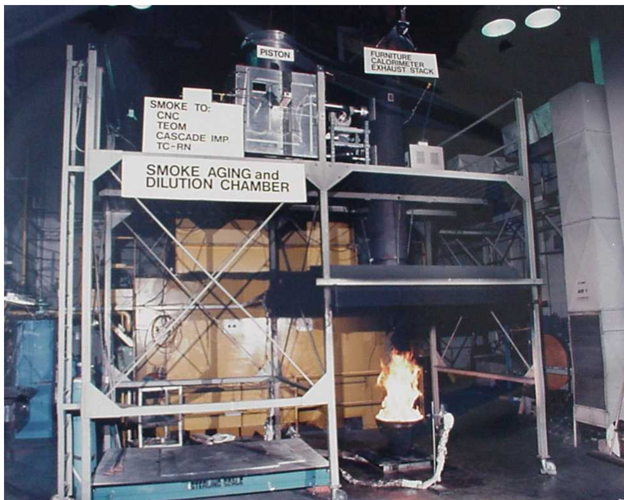
Fig. 2. NIST large calorimeter with smoke sampling equipment installed.
