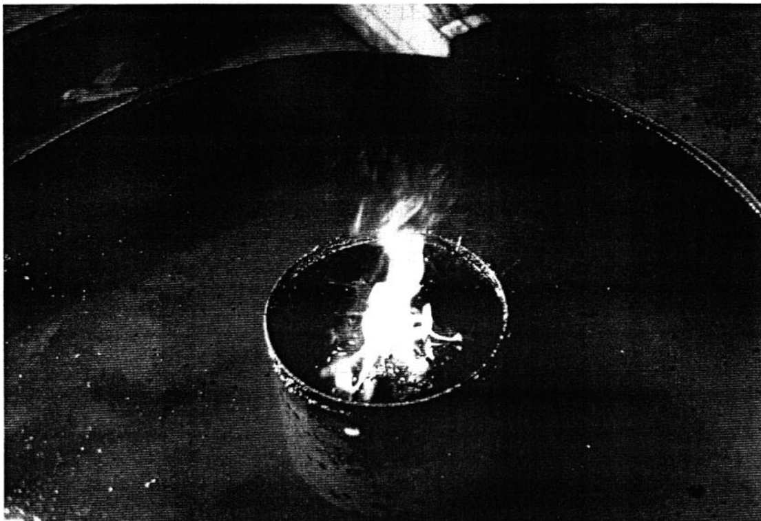
Figure 4 — 10 cm square oil-soaked sorbent pad used for second ignition attempt
