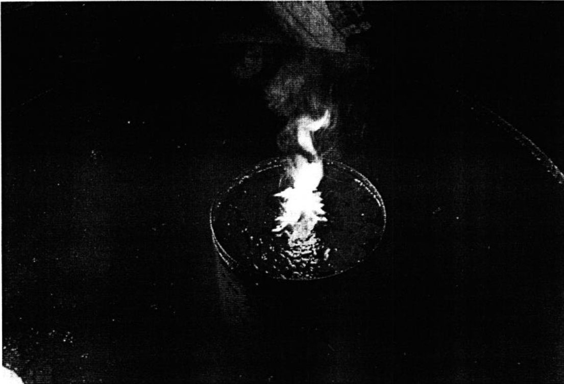
Figure 3 — 5 cm square oil-soaked sorbent pad used for first ignition attempt
