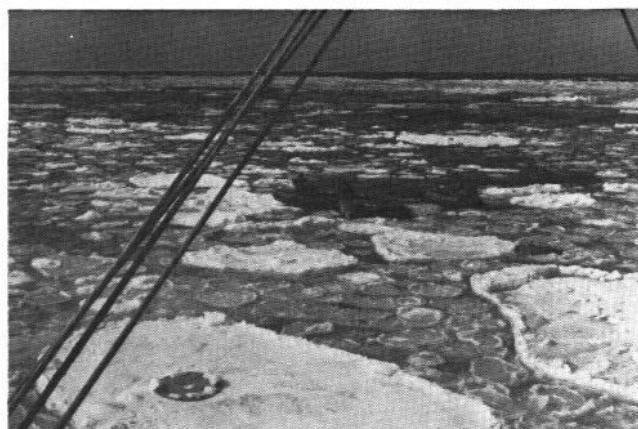
Figure 4. Oil release, spill No. 1—note the disk marker for aerial photography on floe in foreground
