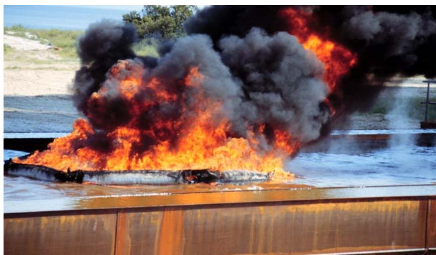
Figure 9. Burning beginning outside boom
