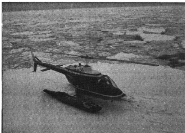
Figure 6. Remote sensing helicopter with sensors mounted on struts
