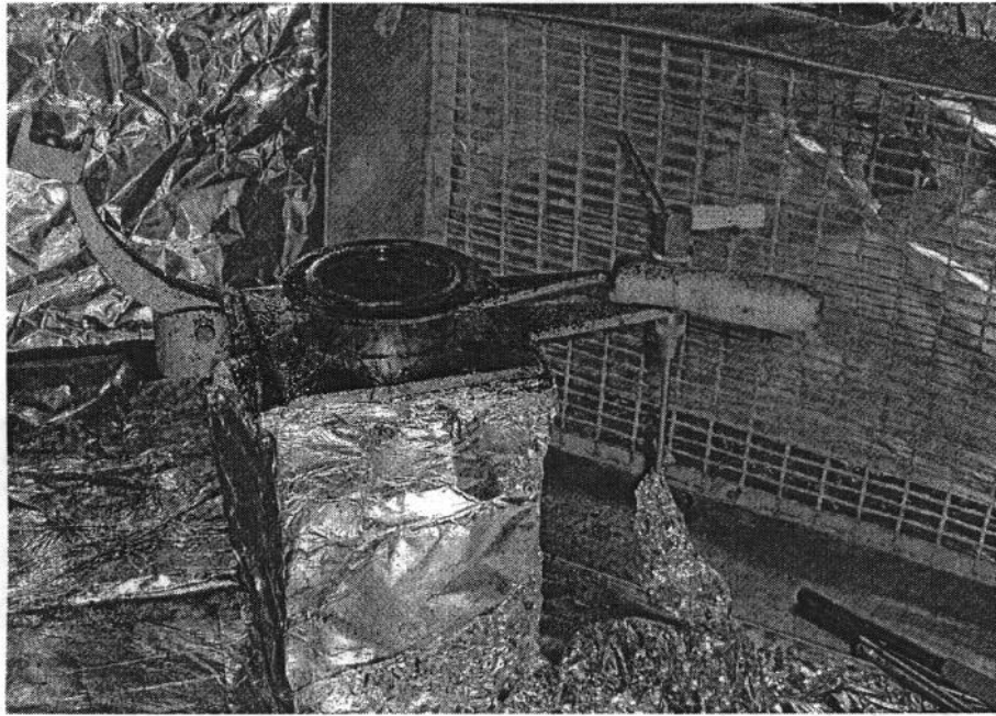
Figure 1 The Cleveland Open Cup Apparatus Used for Small-scale Burning
