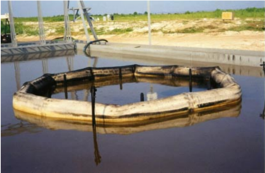
Figure 2. Hydro-Fire Boom, post burn in Mobile.
