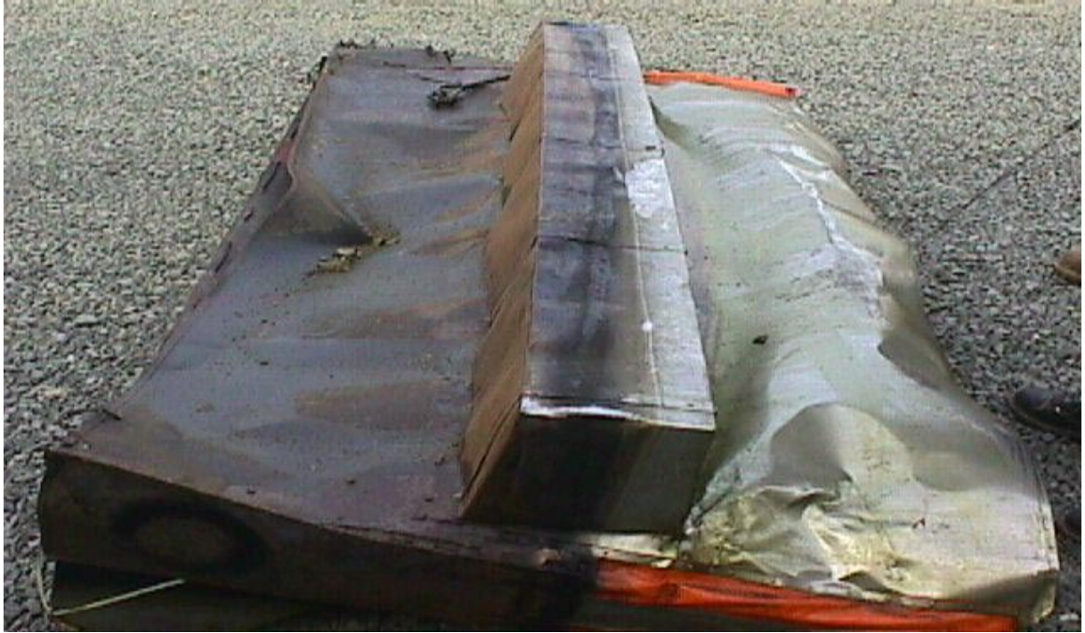
Figure 5. Spill Tain TM boom, arrival condition of boom.
