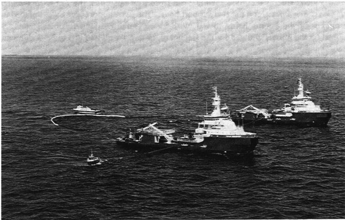
Figure 3.2 Towing formation during test runs using the Texas Responder , Gulf Coast Responder , and a boom handling boat.
