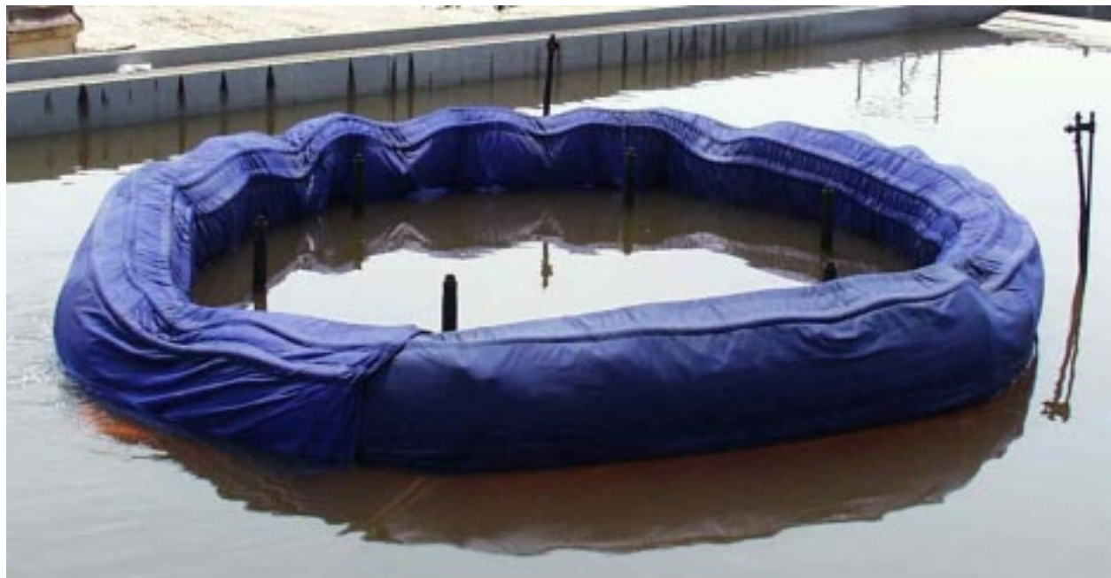
Figure B-2. Boom 2, before burning, in water.
