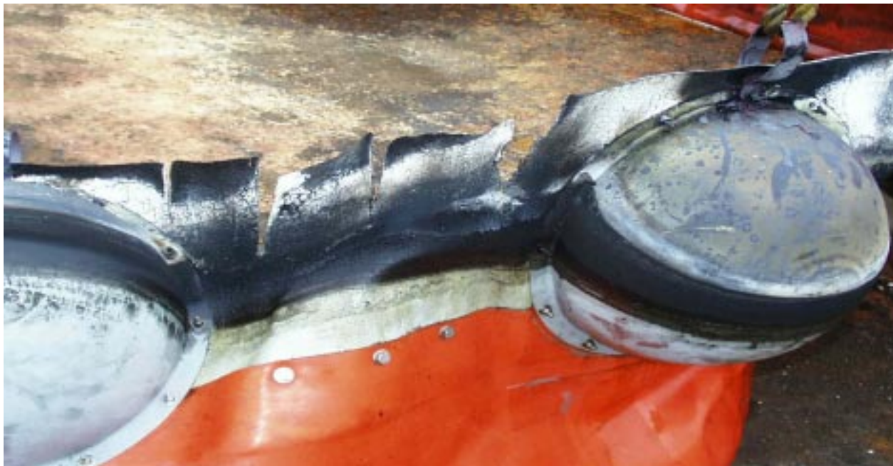
Figure D-6. Boom 4, after burning, close-up.
