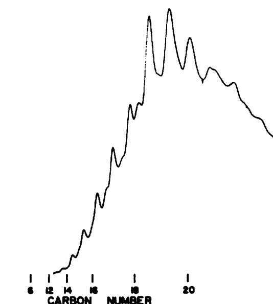
FIG.B RESIDUE OF 6 HRS. AGED FUEL OIL
