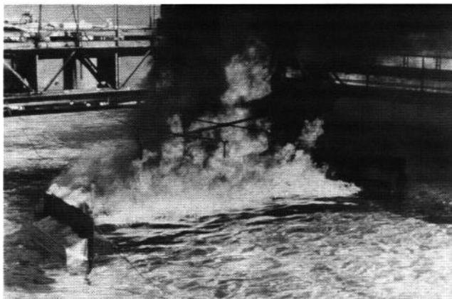
Figure 5. Fireproof boom being tested at the OHMSETT facility
