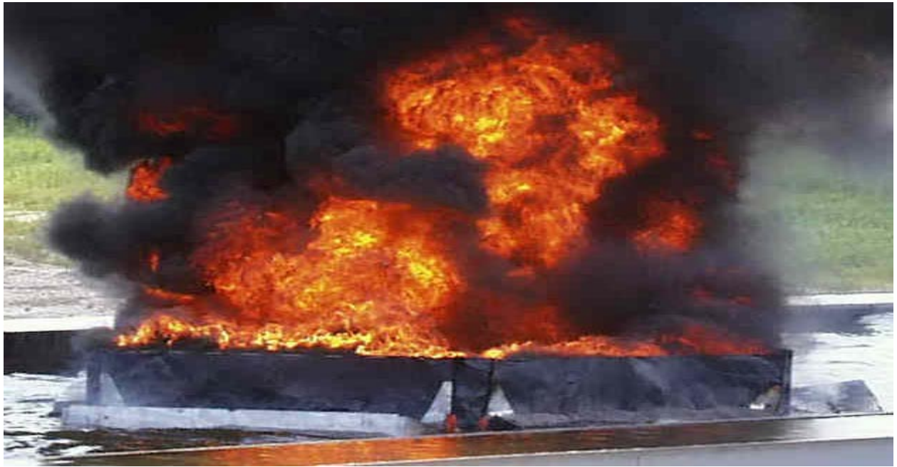
Figure C-3. Boom 3, during burning.
