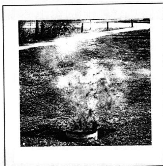
Figure 6. 1 metre Norman Wells burn with 4% ferrocene.
