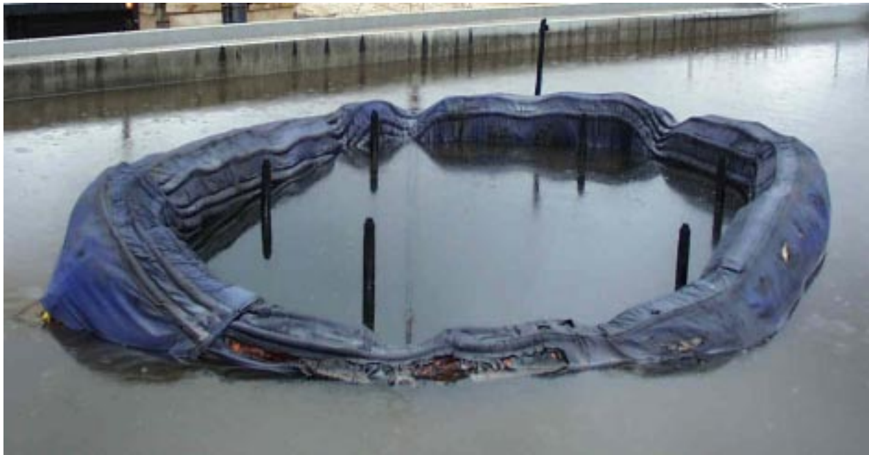
Figure B-4. Boom 2, after burning, in water.
