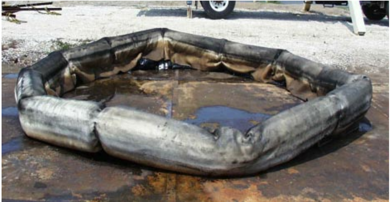
Figure A-5. Boom 1, after burning, on ground.
