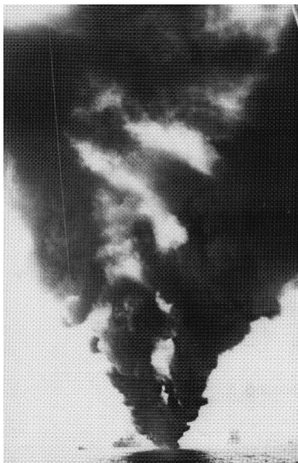
Figure 2. Photograph taken from about 200 m downwind of the Newfoundland Offshore Burn Experiment (NOBE) showing the two large counter-rotating vortices that characterize the structure of the rising smoke plume
