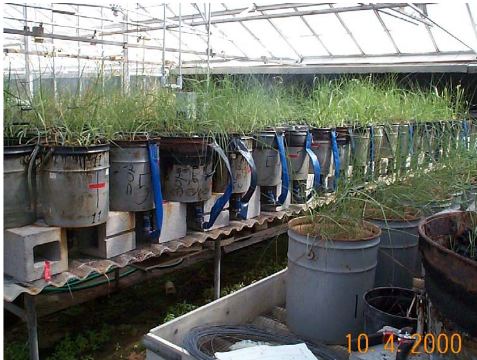
Figure 7. Vegetation Recovery Was Apparent 40 Days After In-Situ Burning.
