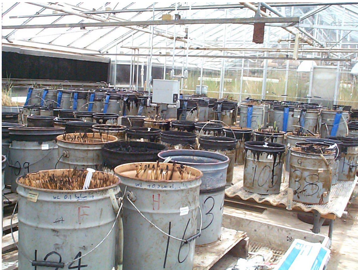
Fig. 6. Burned marsh sods were held in the greenhouse to evaluate the treatment effects on vegetation recovery. Most aboveground biomass of the marsh plants was consumed by the fire during the in-situ burns.
