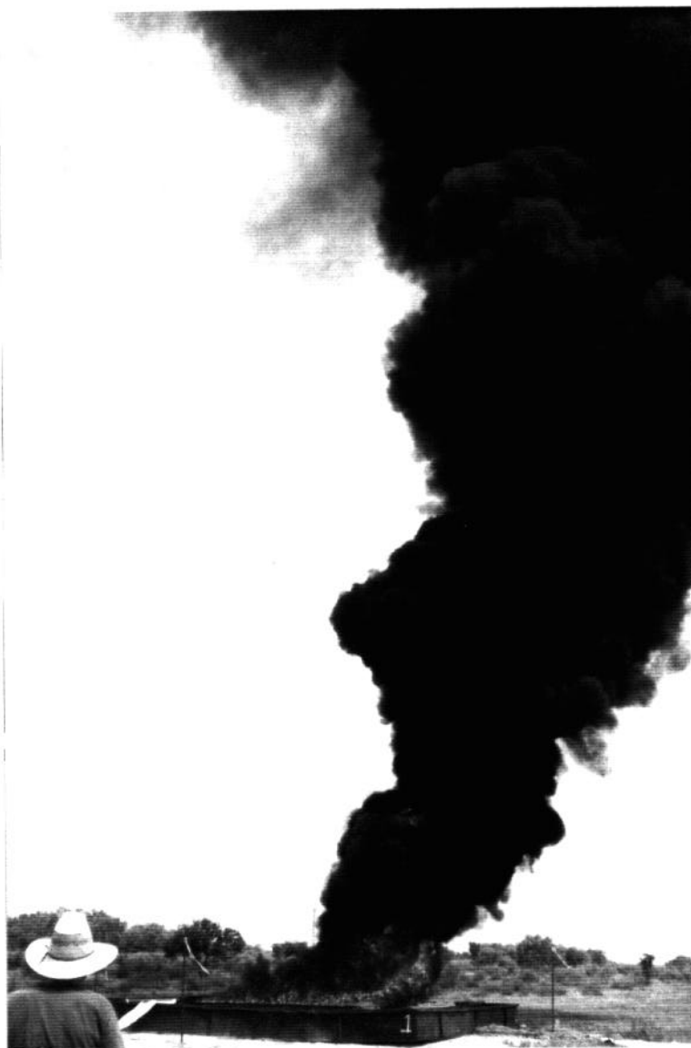
Figure 6.1: Smoke production of baseline burn on day 1 of testing
