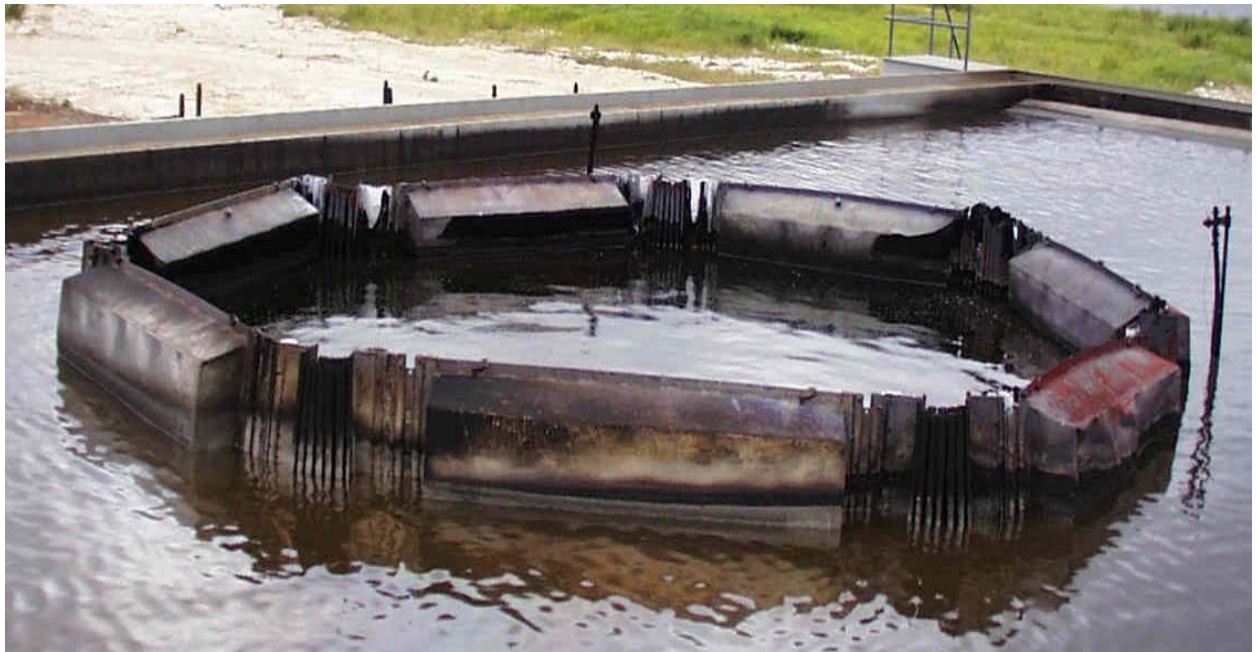
Figure E-4. Boom 5, after burning, in water.
