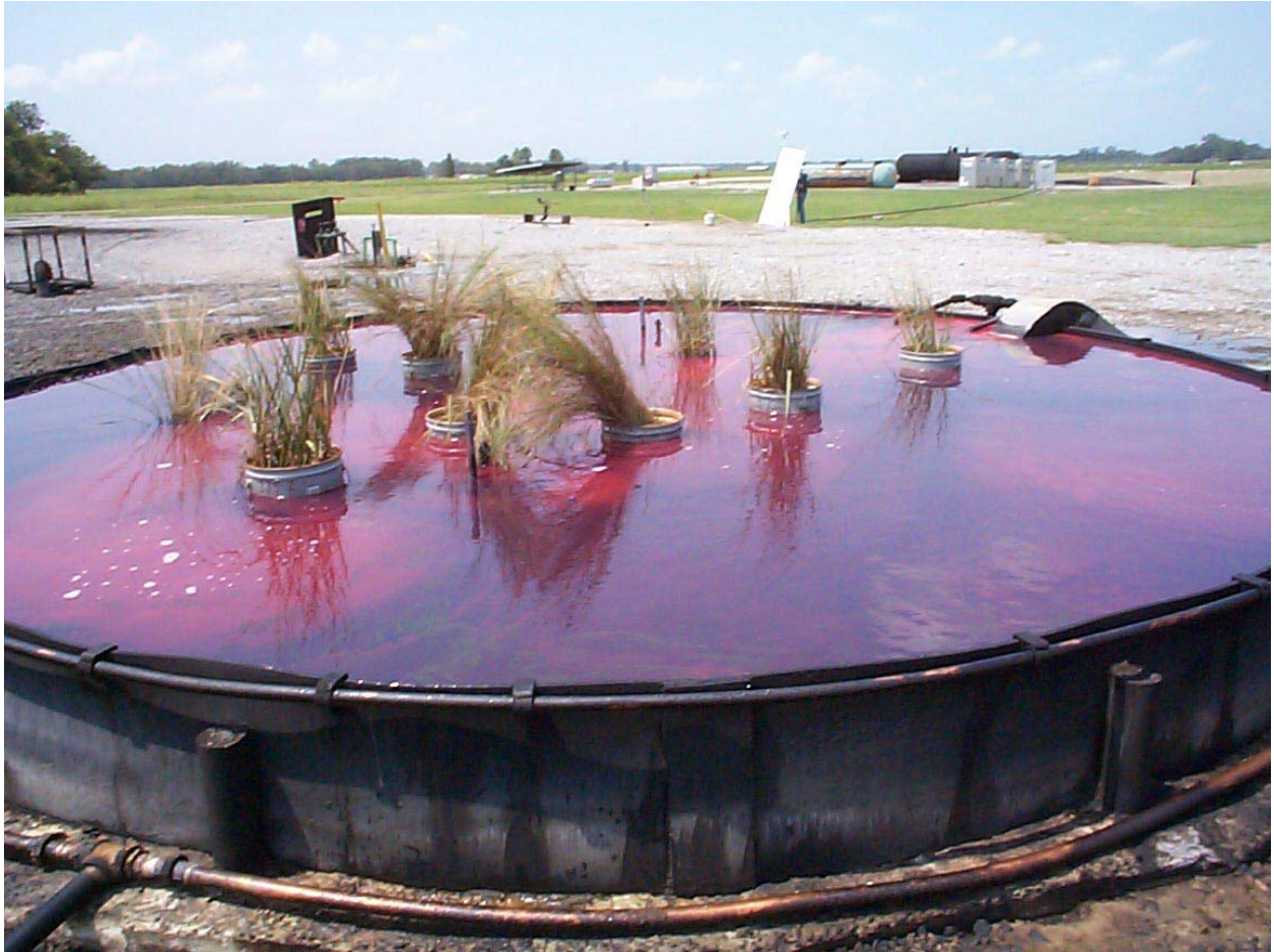
Fig. 3. Diesel fuel was added to the 6 m burn tank before the burn.
