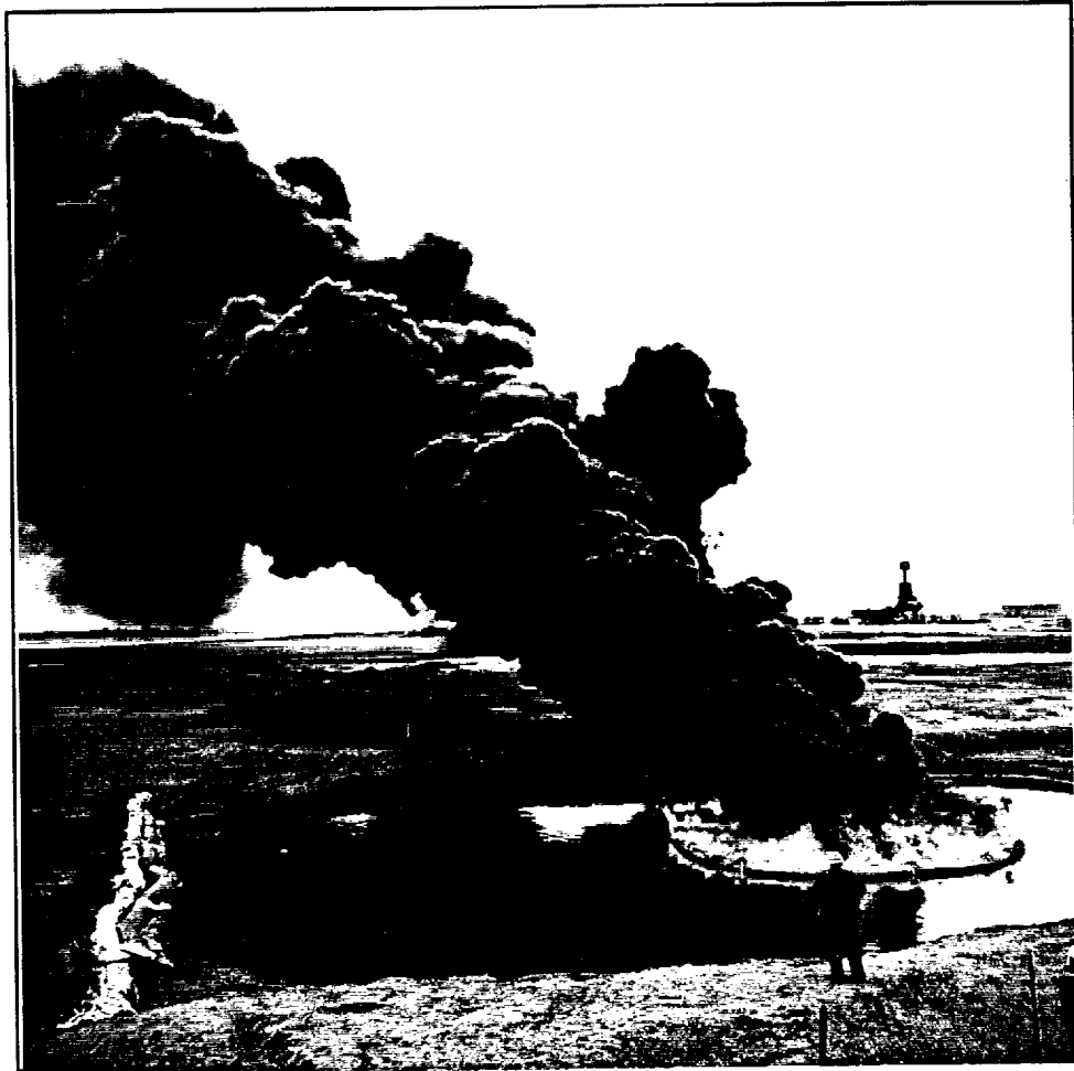
Figure 59 50% water emulsion burn a few minutes after ignition
