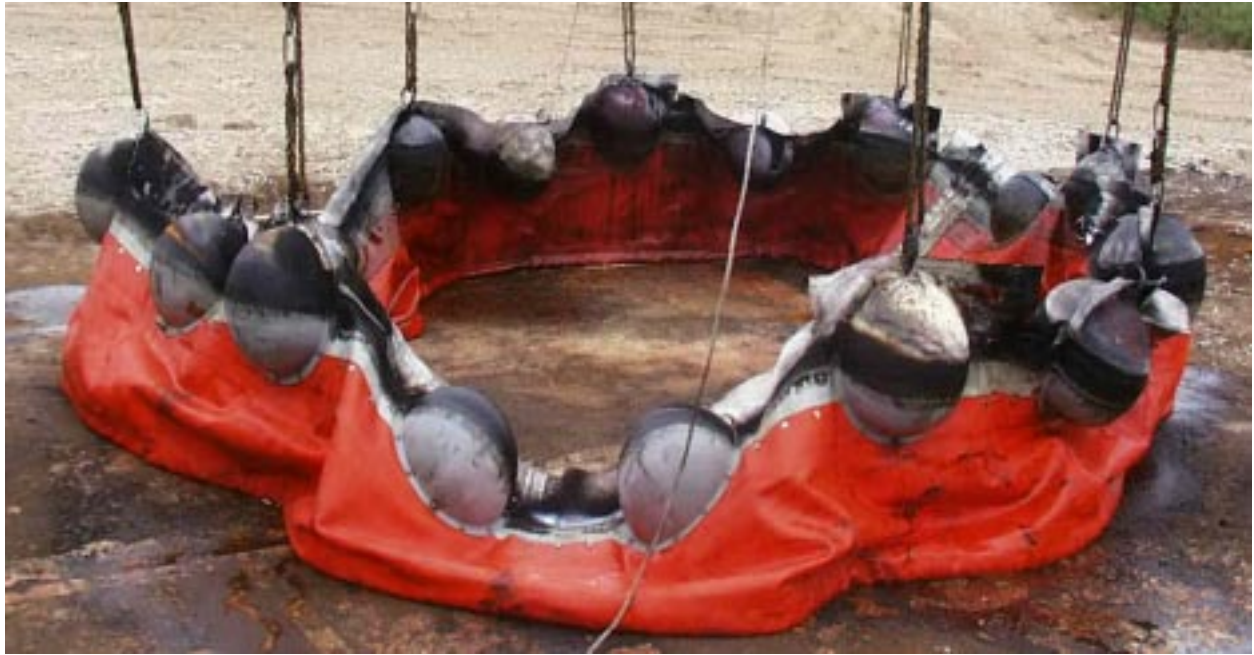
Figure D-5. Boom 4, after burning, on ground.
