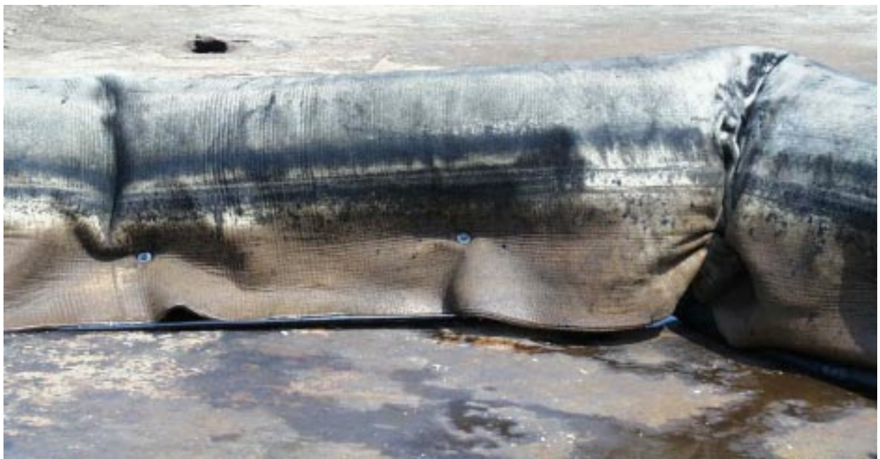
Figure A-5. Boom 1, after burning, on ground.
