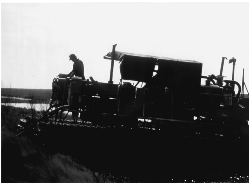
Figure 3. Marsh buggy-mounted skimmer pump used to skim condensate from barrow pits at the Rockefeller Refuge oil spill, Cameron Parish, Louisiana
