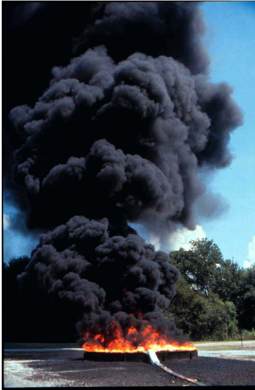
Figure 2 In situ burning of salt marsh sods in the 6 m burn tank for either five or 20 minute burn duration.
