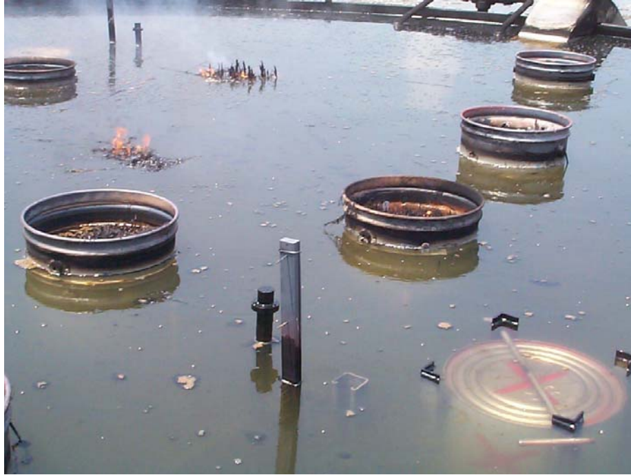
Figure 5. Most Diesel Fuel Was Consumed by the Fire After a 700 s Burn.
