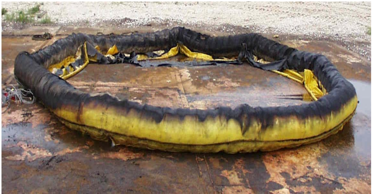
Figure F-5. Boom 6, after burning, on ground.
