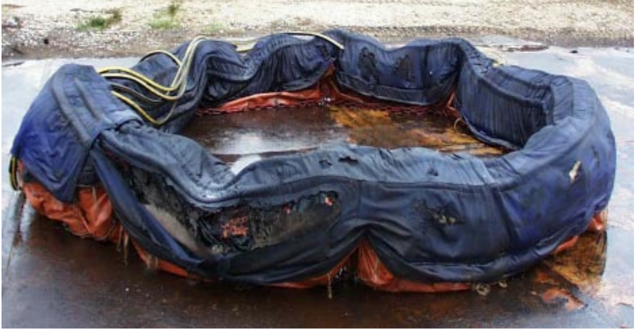
Figure B-5. Boom 2, after burning, on ground.
