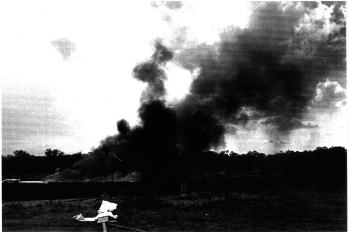
Figure 6.4: Smoke plume produced during test 9 with sub-surface bubbler
