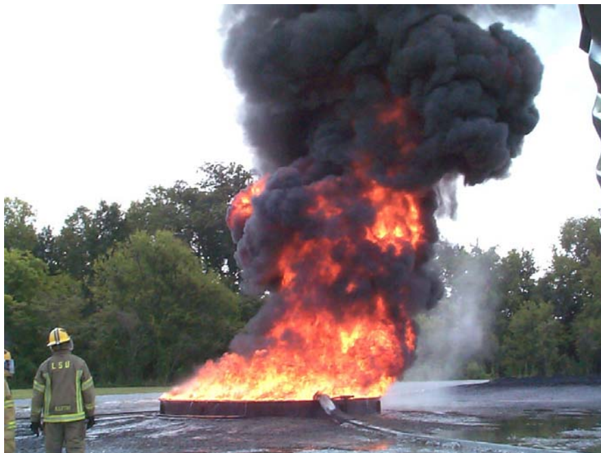
Figure 4. The Fire Intensity in the Burn Tank Was Similar to That of an In-Situ Burn in the Field.
