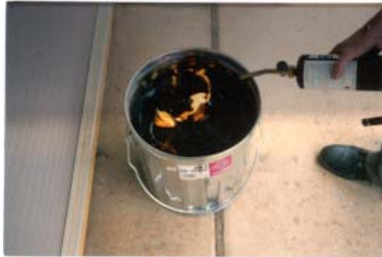
Figure 3. In situ burning of crude oil contaminated soil.
