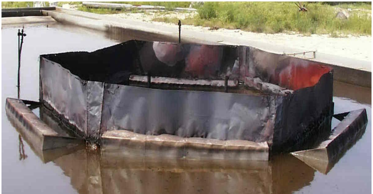
Figure C-4. Boom 3, after burning, in water.
