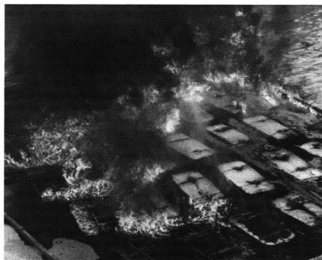
Figure 2. In the first test (calm water/fresh oil 45-percent ice cover) the slick was ignited in the northwest corner of the boomed area. Flames spread south and east through the ice channels. In this test, oil was distributed over the entire test area rather than from the center of the test area as in subsequent tests.
