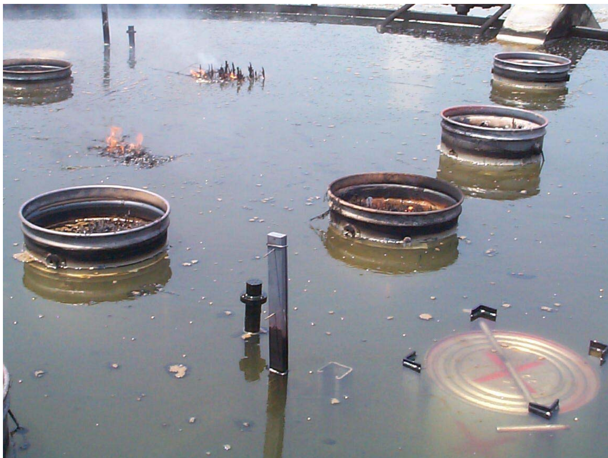
Fig. 5. Most diesel fuel was consumed by the fire after a 700 s burn.
