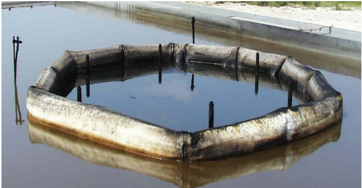
Figure A-4. Boom 1, after burning, in water.
