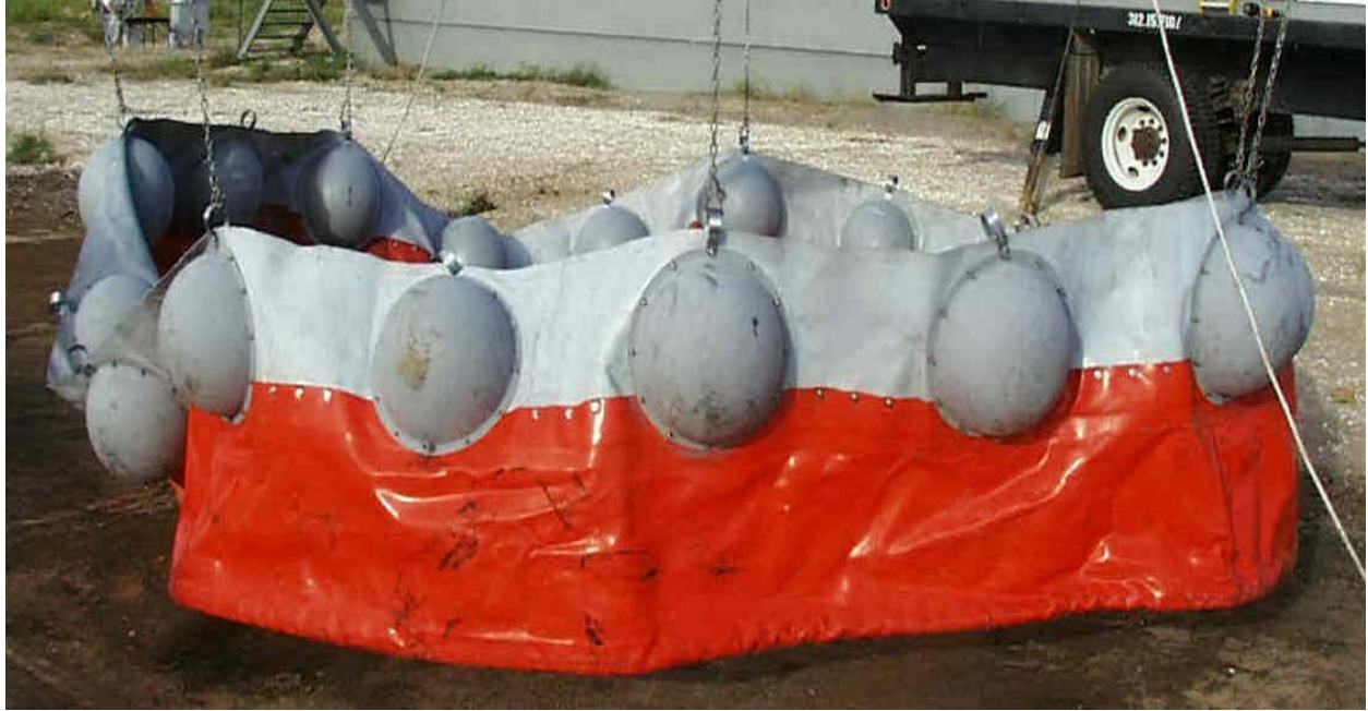
Figure D-1. Boom 4, before burning, on ground.
