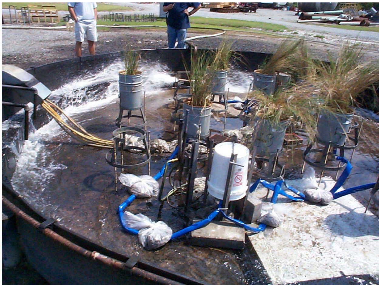
Fig. 1. The 6 m burn tank, containing salt and brackish marsh sods with soil surface at different elevations, was filled with water before the burn.
