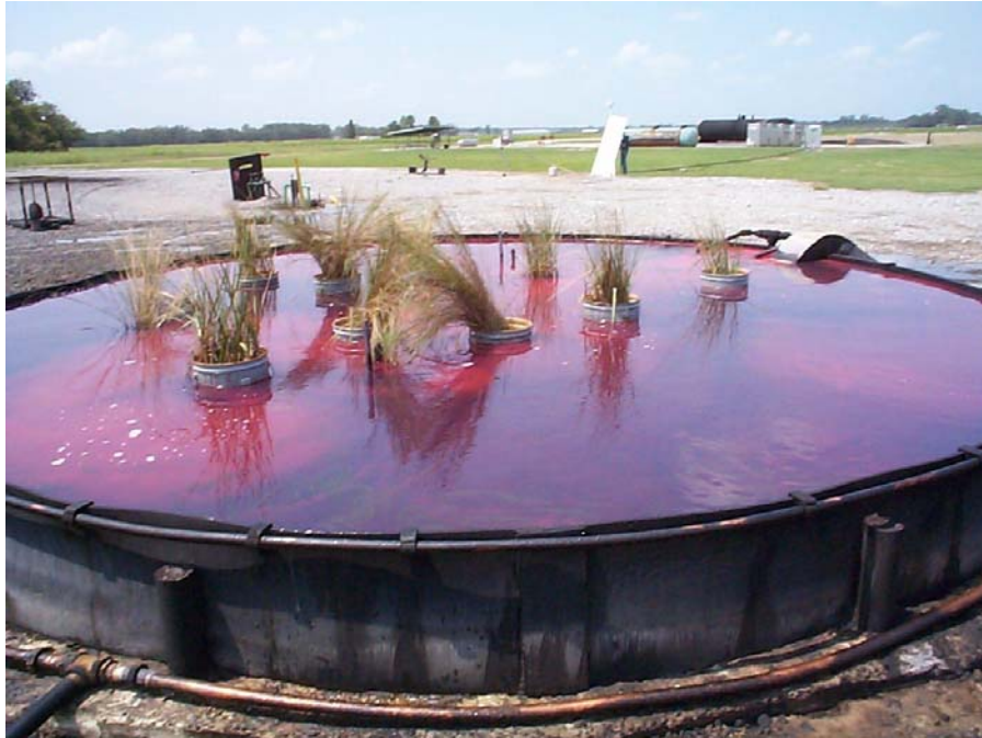
Figure 3. Diesel Fuel Was Added to the 6 m Burn Tank Before the Burn.
