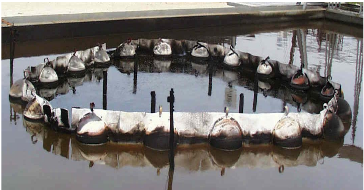
Figure D-4. Boom 4, after burning, in water.
