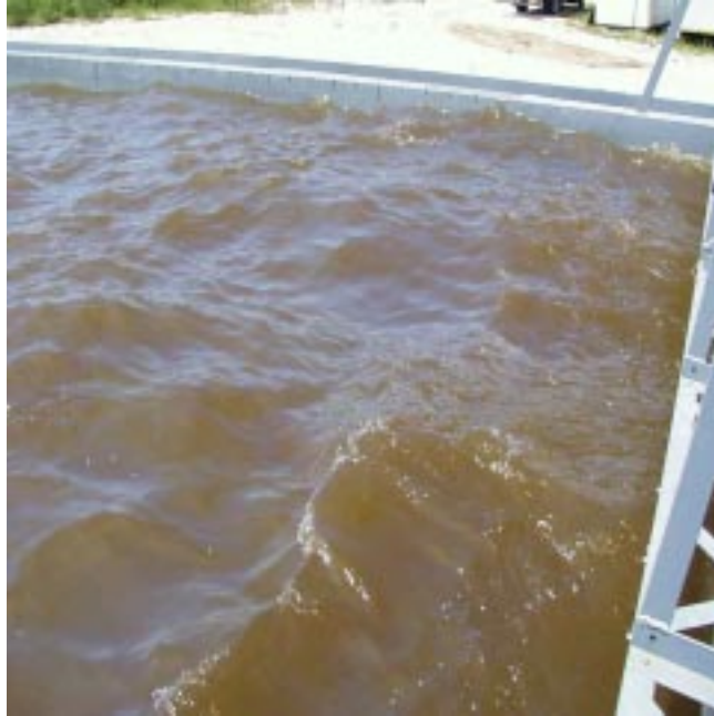
Figure 4. Tank with wave maker in operation.
