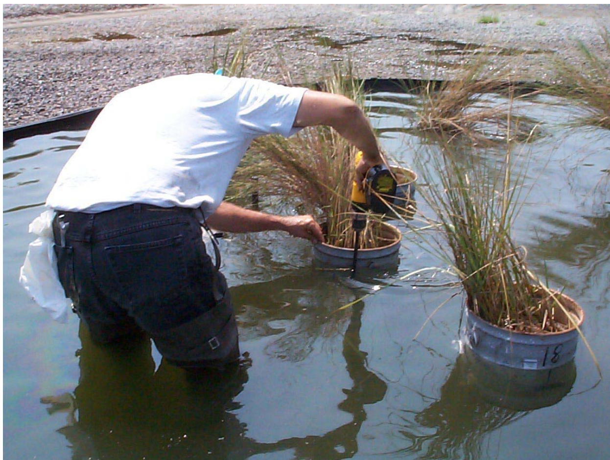
Fig. 2. Fine adjustment of the soil surface of the sods to 10, 2, and -2 cm below the water surface in the 6 m burn tank was conducted before the burn.
