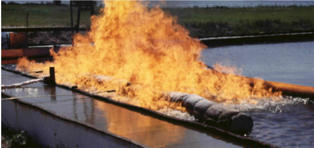
Figure 3. Fire in Propane Wave Tank
