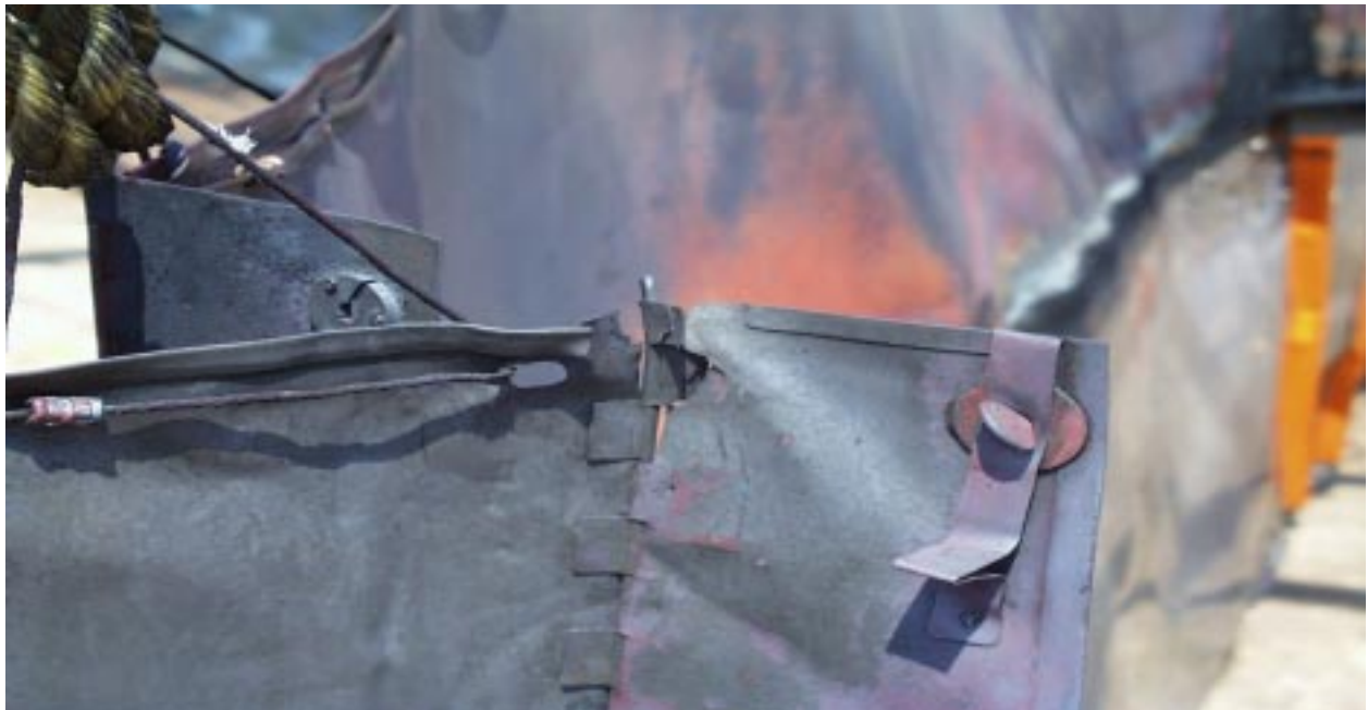
Figure C-6. Boom 3, after burning, close-up.
