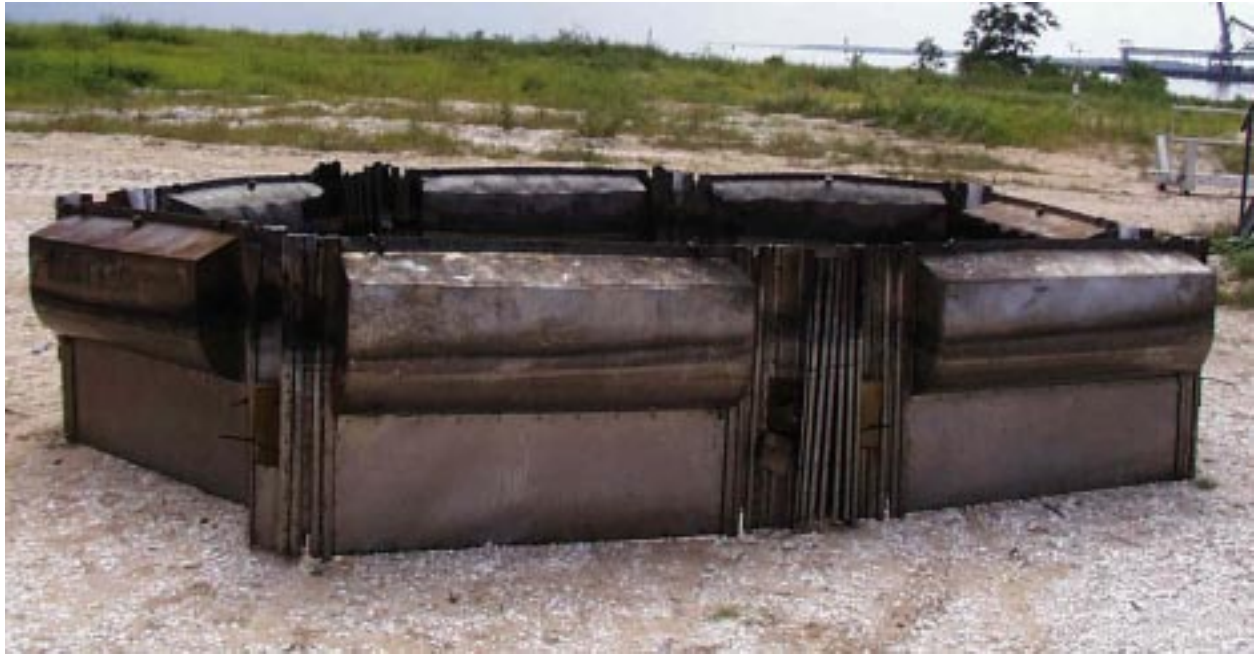
Figure E-5. Boom 5, after burning, on ground.
