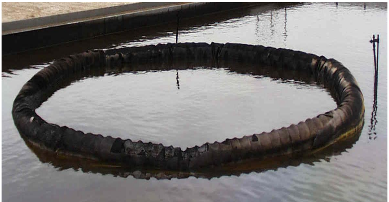
Figure F-4. Boom 6, after burning, in water.
