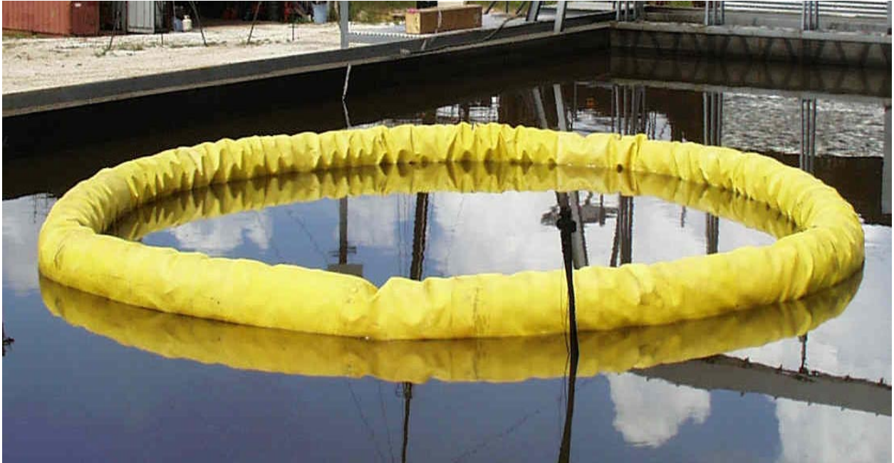
Figure F-2. Boom 6, before burning, in water.
