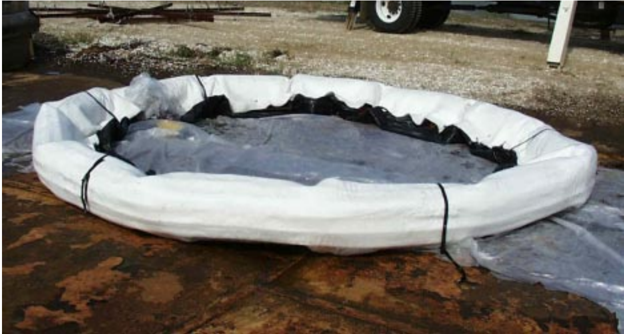
Figure A-1. Boom 1, before burning, on ground.
