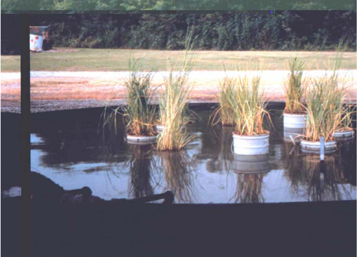
Figure 1 Salt marsh sods located in the 6 m burn tank with soil surface at -10 , -2 , 0 and +10 cm relative to the watersurface before the burn. Half of the sods received 1.5 \text{ l m}^{-2} of diesel oil 24 hour prior to the burn.
