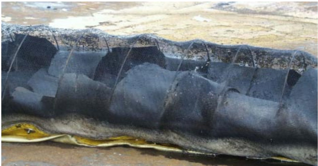
Figure F-6. Boom 6, after burning, close-up.
