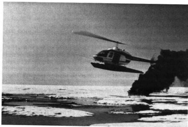
Figure 2. Burning crude oil poured on the surface of land-fast ice. Ignition was achieved by using an air-deployable ignitor.
