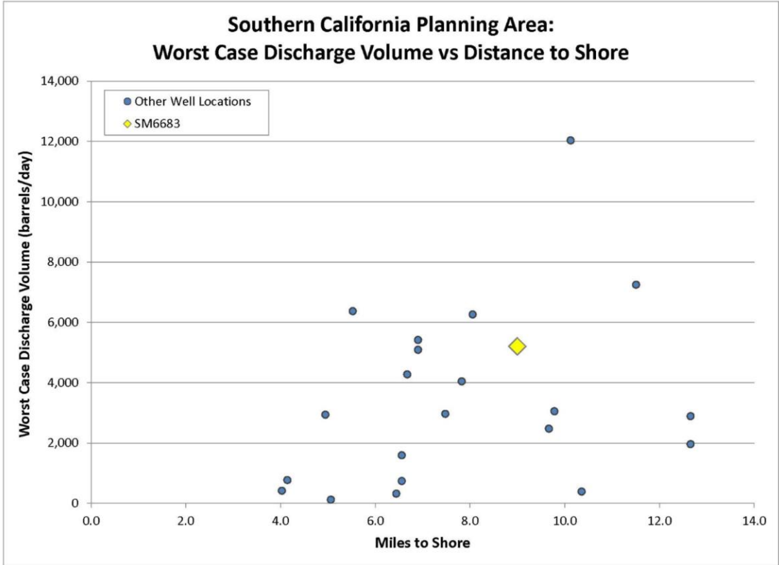
Figure 64: Distances to Shore for WCD Volumes in the Pacific OCS Region and the Location of the Scenario Used in Modeling Highlighted
